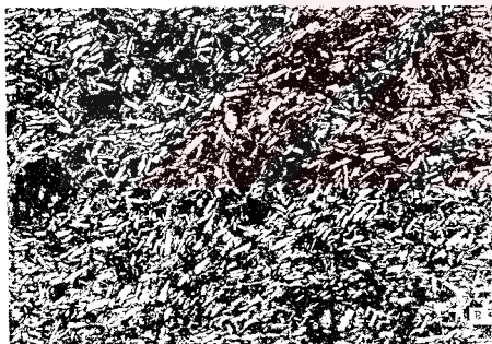
Figure 2. 47 Photomicrograph Showing the Typical Trachytic Texture in Foça Alkaline Lavas. Note the Typically Elongated Microlitic Matrix (a) , Microlitic Matrix Wrapping the Phenocrysts (b, shown by dashed arrow) . The Solid Arrow Shows the Microcrystalline Matrix Grown Over the Feldspar Phenocryst. The Long Side of the Photograph is 6 mm in Length.
