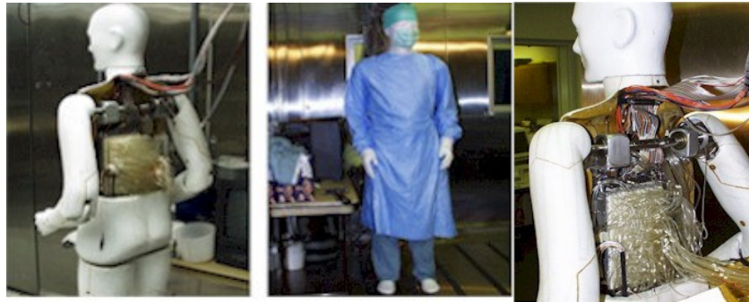
Şekil 3.6 Terleyen manken Coppelius (NC State University Textile Protection and Comfort Center)
