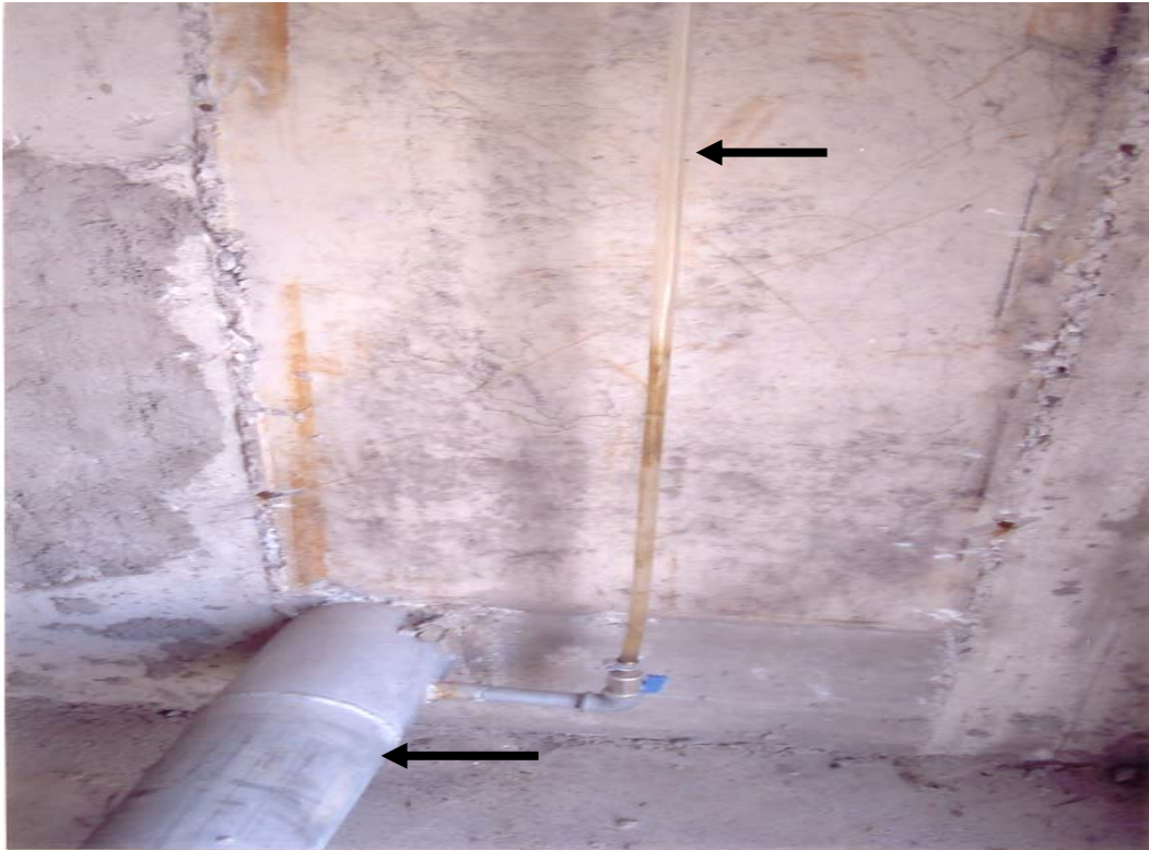
Figure 5.15: To observe the water surface in the tank, the piezometric tube connected to suction flange and datum.
