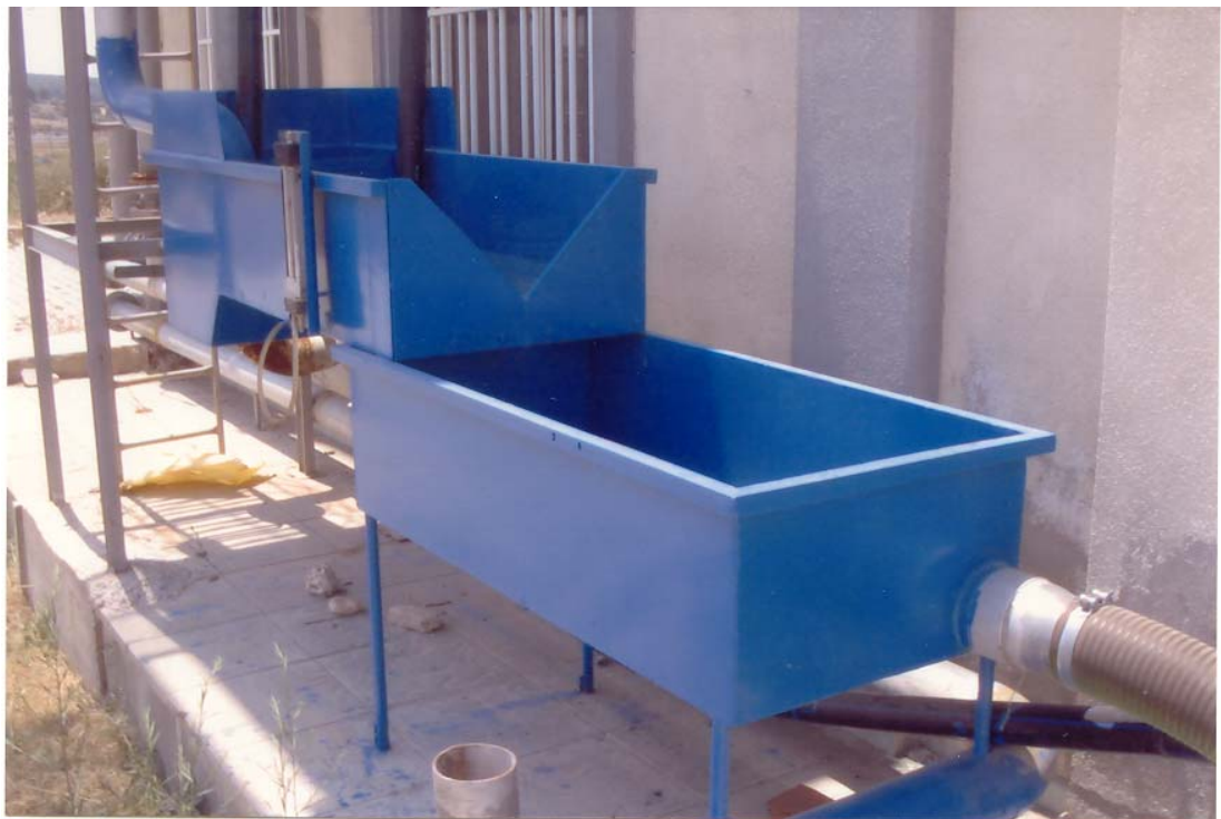
Figure 5.26: 90 degrees triangular V notched weir to measure the steady state discharge in system 2, same as used in the system 1.
