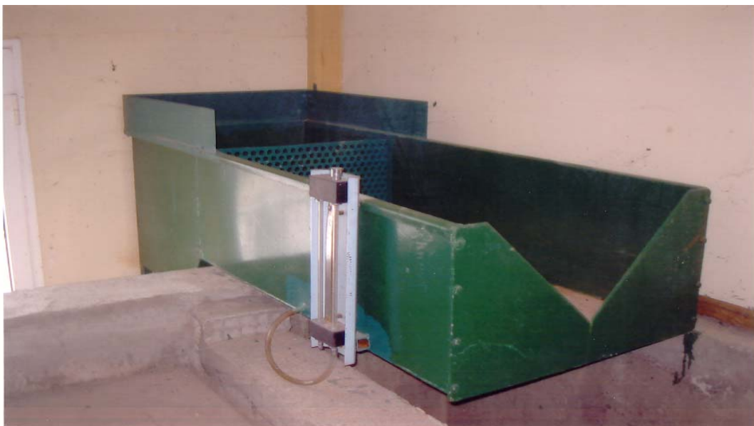
Figure 5.16: 90 degrees triangular V notched triangular weir to measure the steady state discharge for the first system.
