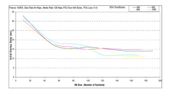
Figure A.21Initial startup time analyses for Filesize 100KB, Data Rate 64 Kbps, PDU Size 640 Bytes, PDU Loss %10.
