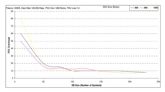
Figure A.1 Transmission cost analyses for Filesize 100KB, Data Rate 128-256 Kbps, PDU Size 1280 Bytes, PDU Loss %1.
