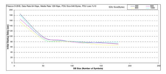
Figure A.30 Initial startup time analyses for Filesize 512KB, Data Rate 64 Kbps, PDU Size 640 Bytes, PDU Loss %10.
