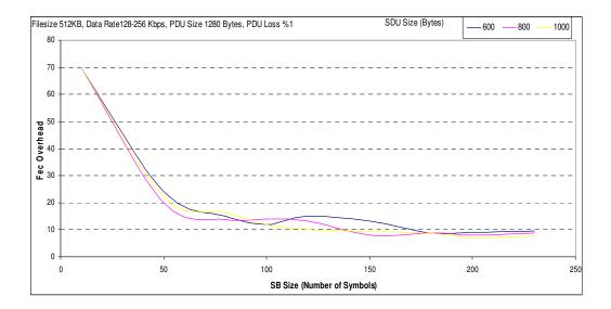
Figure A.4 Transmission cost analyses for Filesize 512KB, Data Rate 128-256 Kbps, PDU Size 1280 Bytes, PDU Loss %1.
