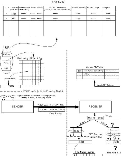
Figure 3.6 Example of the FLUTE flow diagram.
