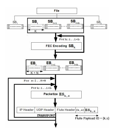
Figure 5.3 System model for the interleaved download delivery.
