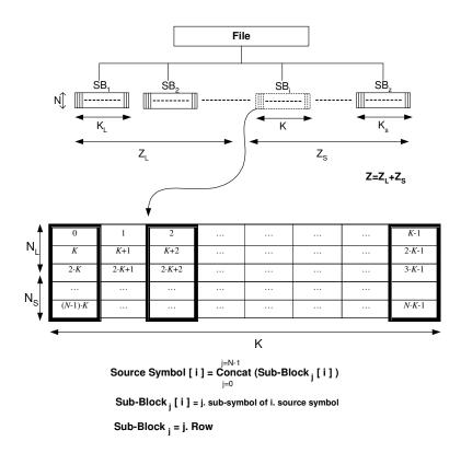
Figure 4.5 Source block construction.
