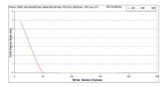
Figure A.15 Initial startup time analyses for Filesize 100KB, Data Rate 256 Kbps, PDU Size 1280 Bytes, PDU Loss %10.
