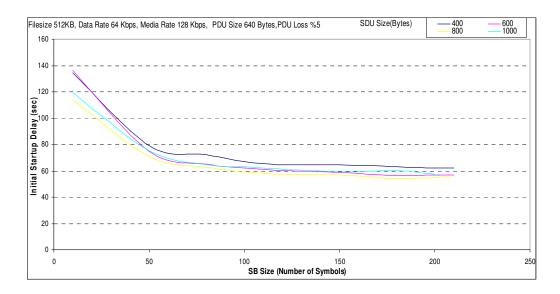
Figure A.29 Initial startup time analyses for Filesize 512KB, Data Rate 64 Kbps, PDU Size 640 Bytes, PDU Loss %5.
