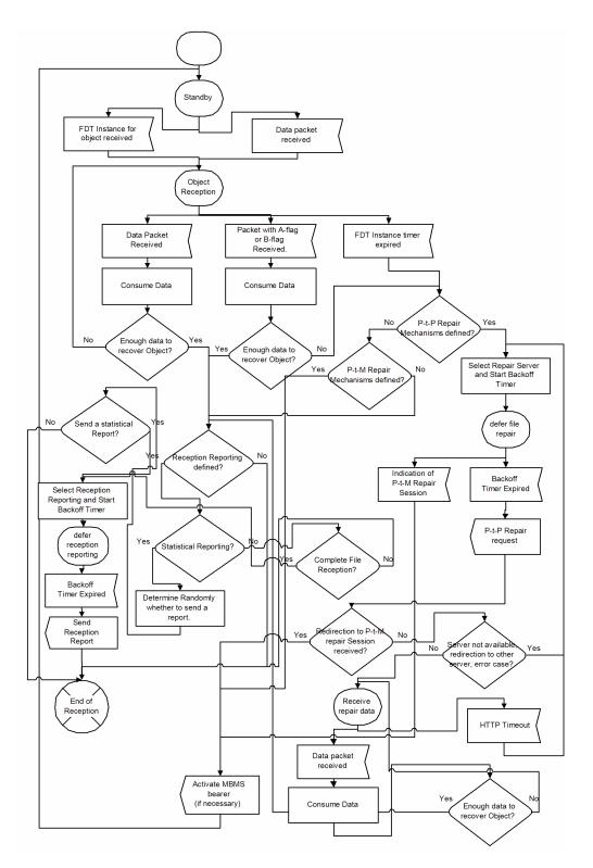
Figure 4.6 Detailed SDL diagram for the file download process of MBMS UE (3GPP TSG 26.946, 2007, p.15).
