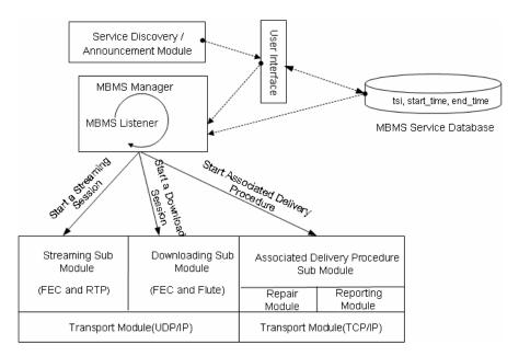
Figure 5.1 Vidiator MBMS prototype software modules.
