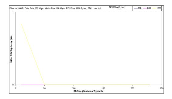
Figure A.13 Initial startup time analyses for Filesize 100KB, Data Rate 256 Kbps, PDU Size 1280 Bytes, PDU Loss %1.
