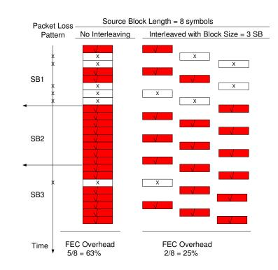
randomization of the transmission order of all symbols. In the example in Figure 2.8, different transmission strategy is used to show the effect of interleaving.
