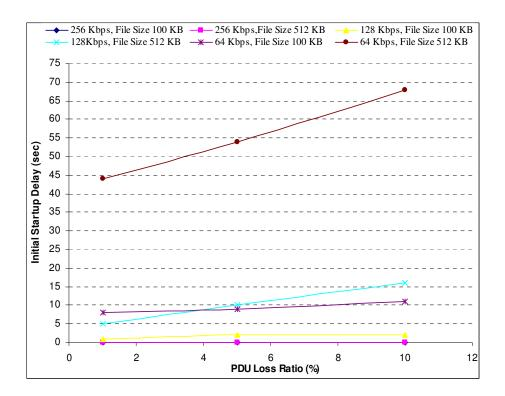
Figure 6.7 Initial startup delay for various PDU loss ratios.
