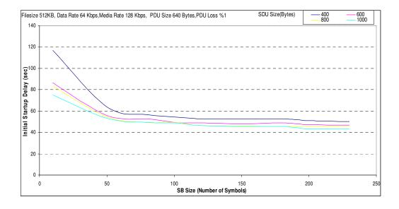
Figure A.28 Initial startup time analyses for Filesize 512KB, Data Rate 64 Kbps, PDU Size 640 Bytes, PDU Loss %1.
