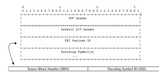
Figure 4.2 FEC payload ID in MBMS FLUTE.
