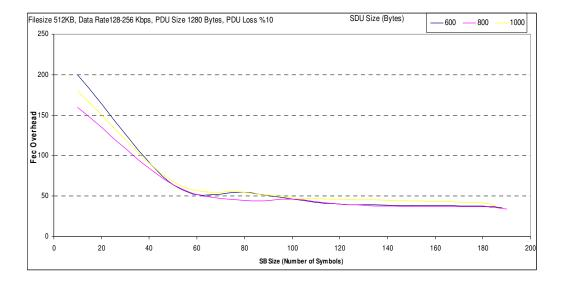
Figure A.6 Transmission cost analyses for Filesize 512KB, Data Rate 128-256 Kbps, PDU Size 1280 Bytes, PDU Loss %10.
