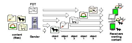
Figure 3.3 Four files described by one FDT instance.
