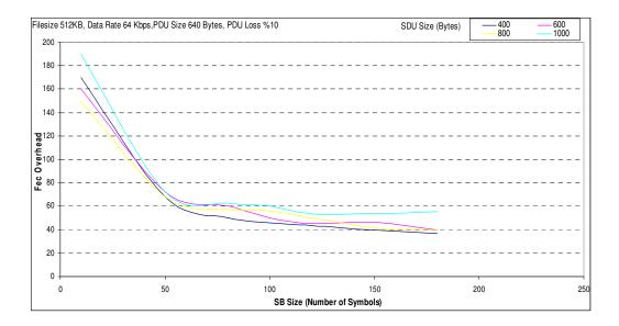
Figure A.12 Transmission cost analyses for Filesize 512KB, Data Rate 64 Kbps, PDU Size 640 Bytes, PDU Loss %10.
