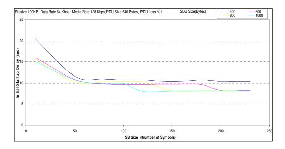
Figure A.19 Initial startup time analyses for Filesize 100KB, Data Rate 64 Kbps, PDU Size 640 Bytes, PDU Loss %1.
