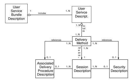
Figure 4.1 MBMS download delivery service description fragments (3GPP TSG 26.346, 2007).
