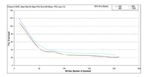
Figure A.11 Transmission cost analyses for Filesize 512KB, Data Rate 64 Kbps, PDU Size 640 Bytes, PDU Loss %5.
