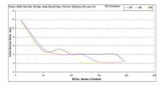
Figure A.18 Initial startup time analyses for Filesize 100KB, Data Rate 128 Kbps, PDU Size 1280 Bytes, PDU Loss %10.
