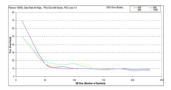
Figure A.7 Transmission cost analyses for Filesize 100KB, Data Rate 64 Kbps, PDU Size 640 Bytes, PDU Loss %1.
