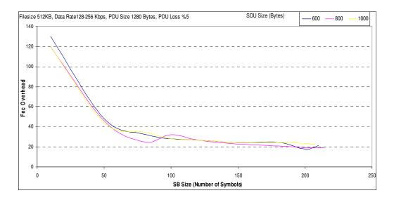
Figure A.5 Transmission cost analyses for Filesize 512KB, Data Rate 128-256 Kbps, PDU Size 1280 Bytes, PDU Loss %5.
