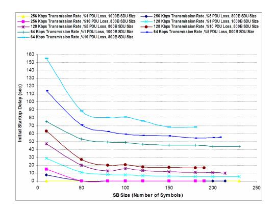
Figure 6.6 Initial startup delay analyses for 512 KB file.
