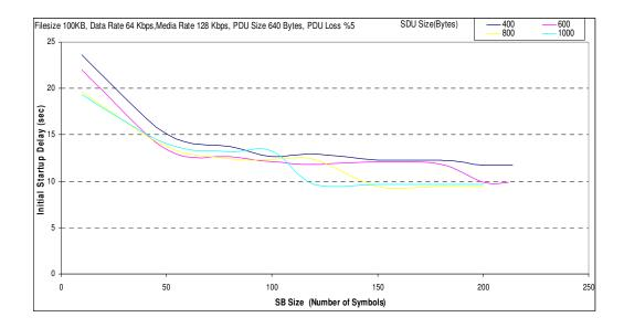
Figure A.20 Initial startup time analyses for Filesize 100KB, Data Rate 64 Kbps, PDU Size 640 Bytes, PDU Loss %5.
