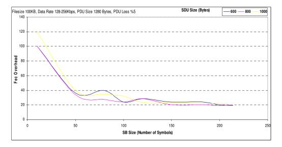
Figure A.2 Transmission cost analyses for Filesize 100KB, Data Rate 128-256 Kbps, PDU Size 1280 Bytes, PDU Loss %5
