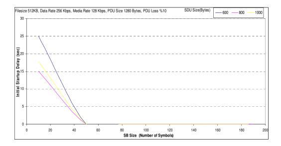
Figure A.24 Initial startup time analyses for Filesize 512KB, Data Rate 256 Kbps, PDU Size 1280 Bytes, PDU Loss %10.
