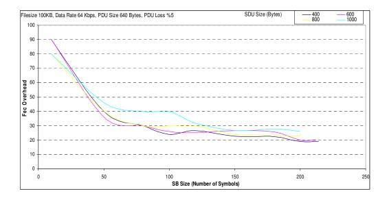
Figure A.8 Transmission cost analyses for Filesize 100KB, Data Rate 64 Kbps, PDU Size 640 Bytes, PDU Loss %5.
