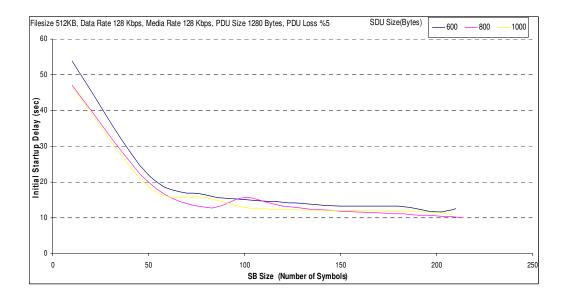
Figure A.26 Initial startup time analyses for Filesize 512KB, Data Rate 128 Kbps, PDU Size 1280 Bytes, PDU Loss %5.
