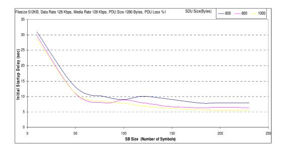
Figure A.25 Initial startup time analyses for Filesize 512KB, Data Rate 128 Kbps, PDU Size 1280 Bytes, PDU Loss %1.
