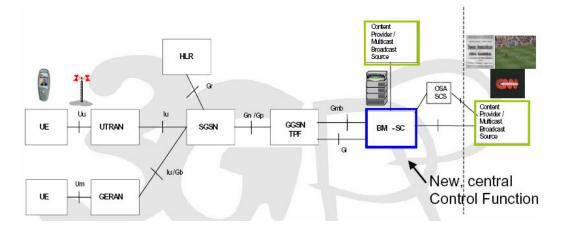
Figure 2.4 MBMS architecture as defined by 3GPP (3GPP TSG 26.346, 2007).
