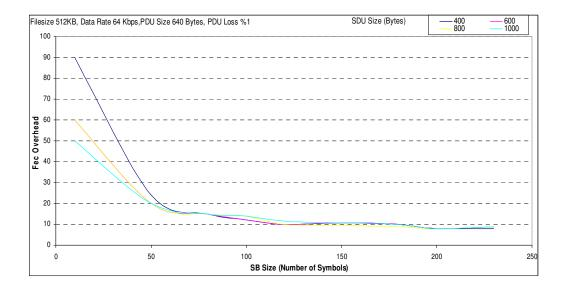
Figure A.10 Transmission cost analyses for Filesize 512KB, Data Rate 64 Kbps, PDU Size 640 Bytes, PDU Loss %1.
