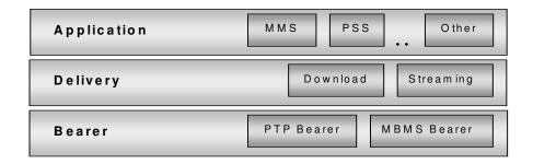
Figure 2.3 Functional layers for MBMS service delivery (3GPP TSG 26.346, 2007).
