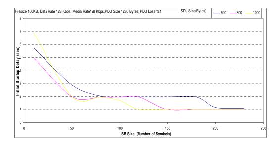
Figure A.16 Initial startup time analyses for Filesize 100KB, Data Rate 128 Kbps, PDU Size 1280 Bytes, PDU Loss %1.
