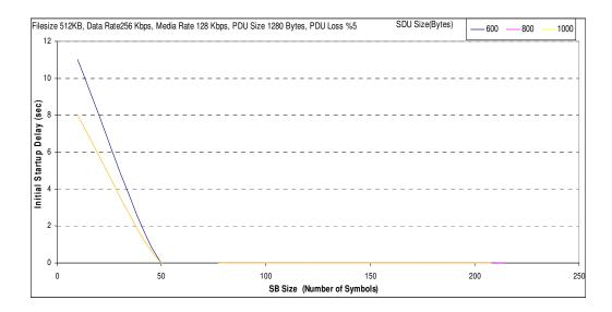
Figure A.23 Initial startup time analyses for Filesize 512KB, Data Rate 256 Kbps, PDU Size 1280 Bytes, PDU Loss %5.
