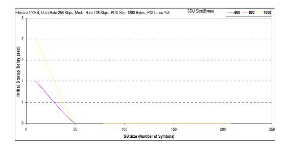
Figure A.14 Initial startup time analyses for Filesize 100KB, Data Rate 256 Kbps, PDU Size 1280 Bytes, PDU Loss %5.
