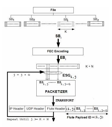
Figure 5.2 System model for the legacy download delivery.
