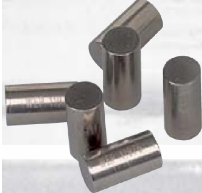
Figure 4.7 Cylindrical ingots used to prepare the test samples.
