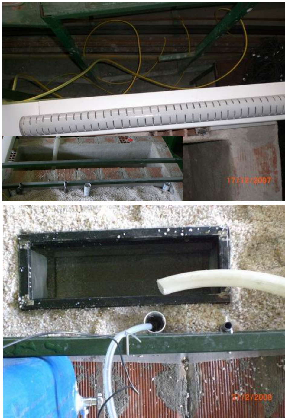
Figure A.21 Placement of the pipes and the box to give tracer into the channel
