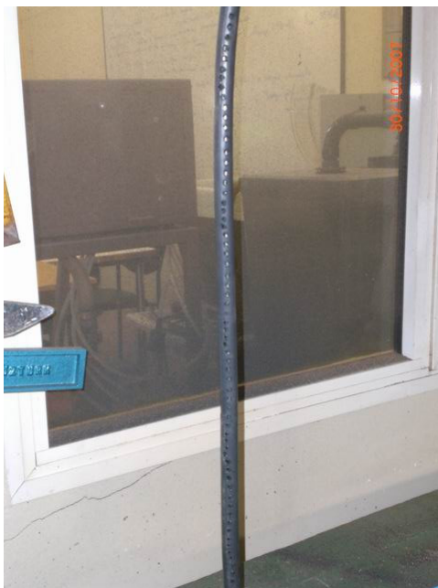
Figure A.17 Preparation of the perforated plastic pipes
