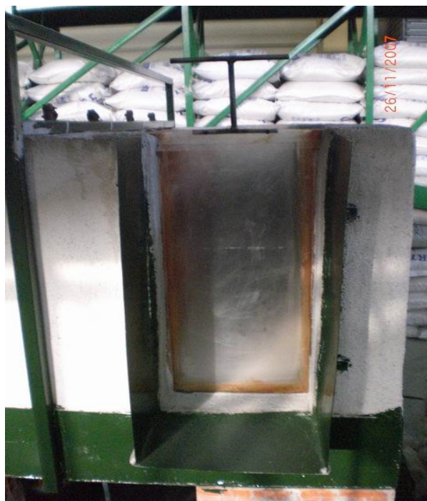
Figure A.16 The water supply tank and the gate of the downstream reservoir
