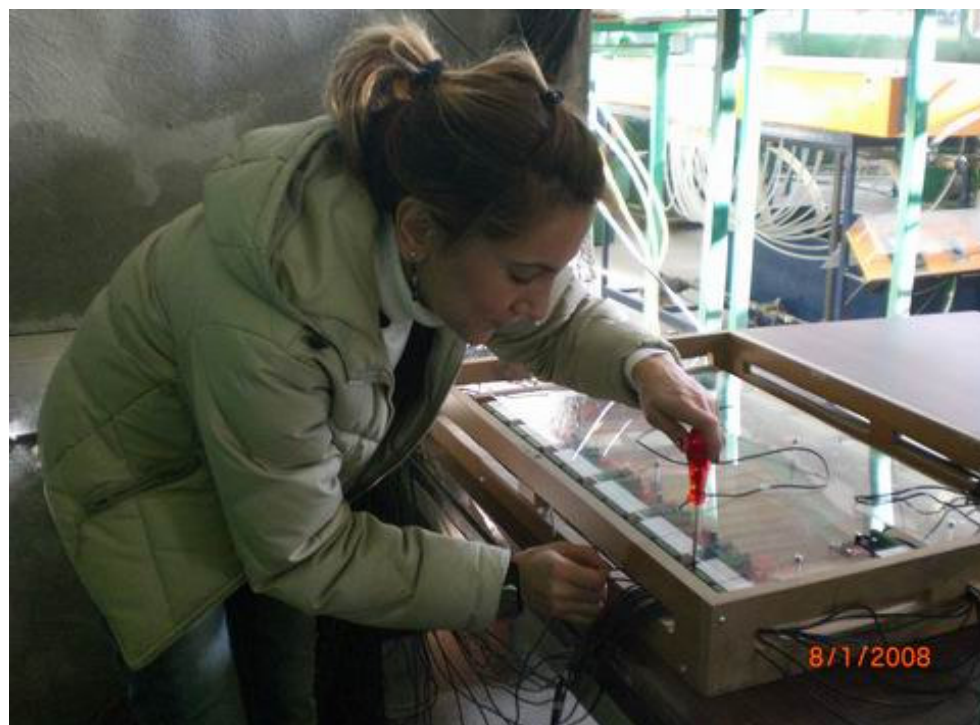
Figure A.29 Mounting and connection of the copper wires
