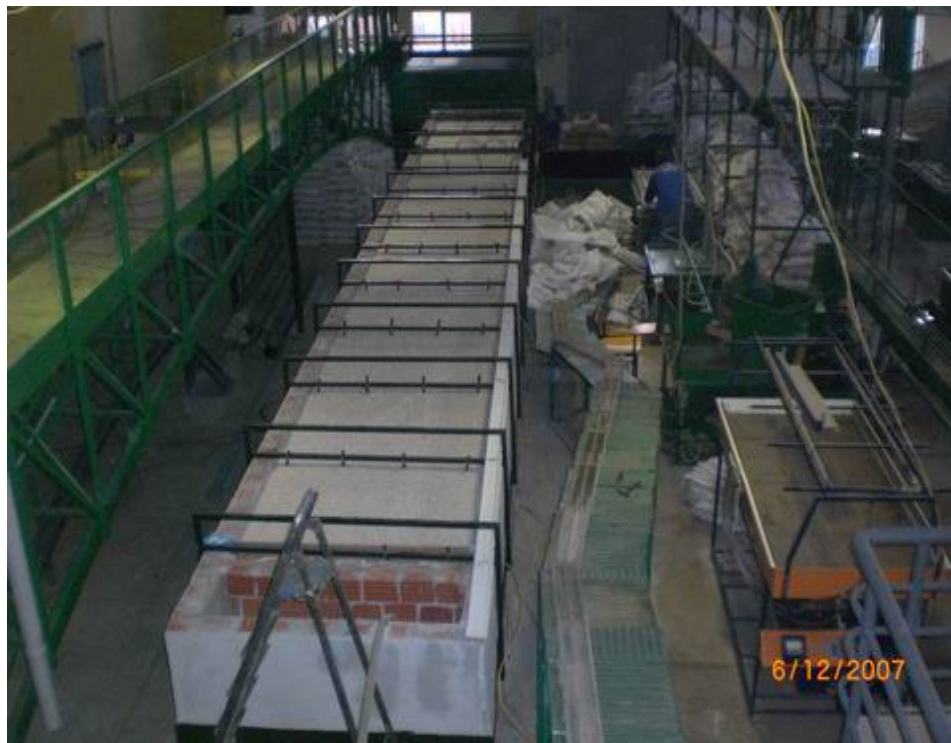
Figure A.22 Filling of the channel with coarse sand
