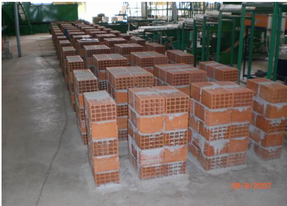
Figure A.1 Constructions of the brick piers
