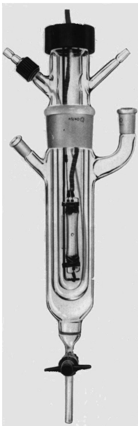
Figure 3.10 125 W lamp, quartz-walled immersion well reactor
