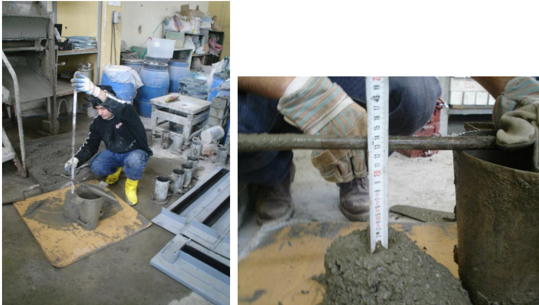
Figure 4.26 (c) Slump tests
