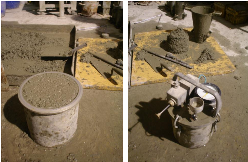
Figure 4.26 (b) Air content test
