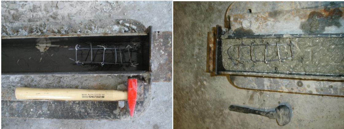
Figure 4.32 Reinforcement at the head of the model pile for conventional concrete (c) and steel fiber reinforced concrete (sfrc)
