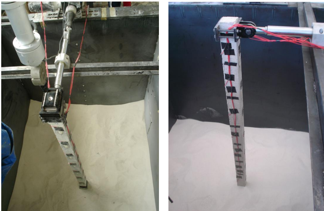
Figure 4.39 Model pile placement into the test container
