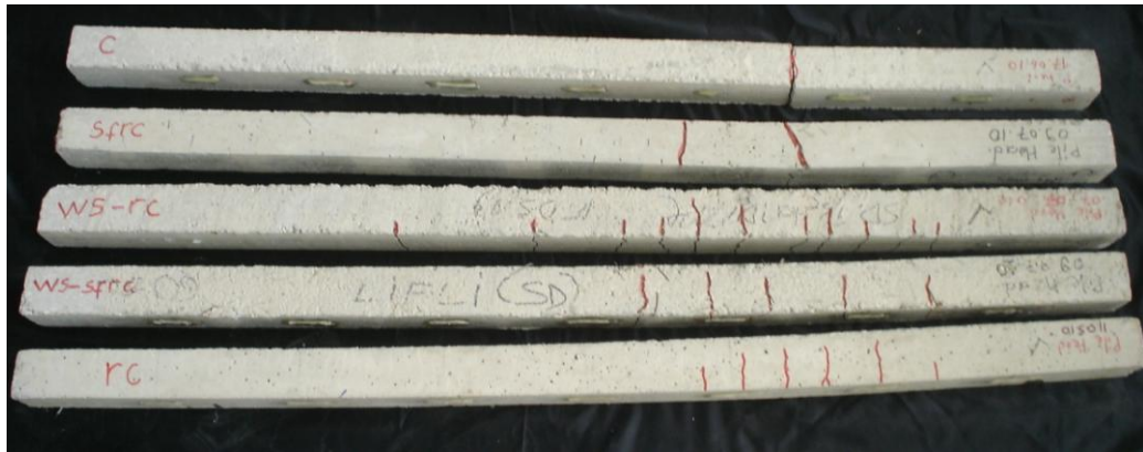
Figure 5.33 Damaged model piles after the tests, 4mm/min
