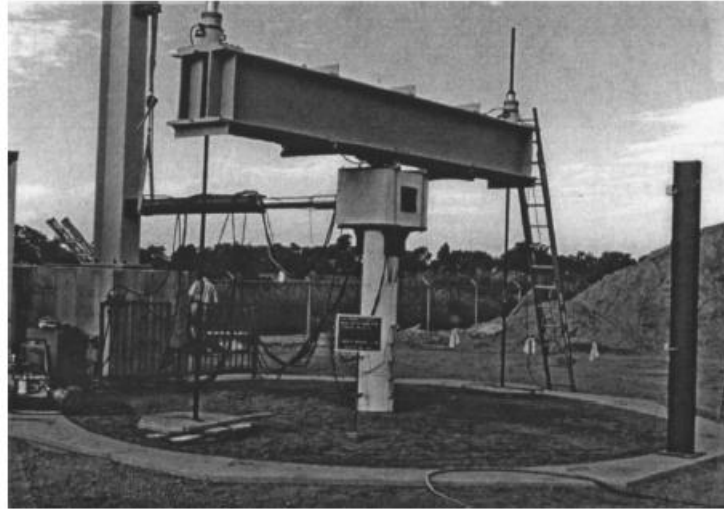
Figure 2.35 Soil-reinforced concrete pile test set up (Chai & Hutchinson, 2002)
