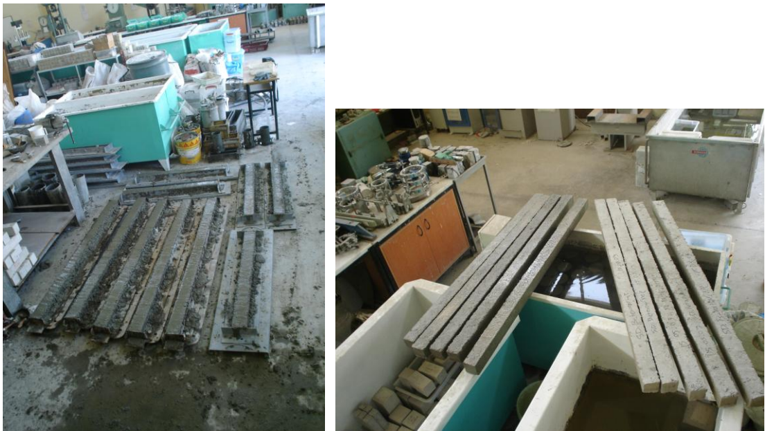
Figure 4.35 Cast and cured model piles
