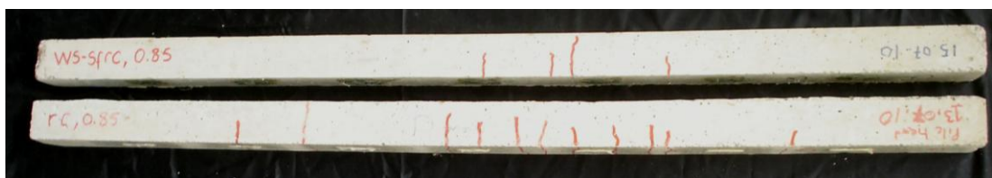
Figure 5.44 Damaged model piles after the test, 0.85 mm/min
