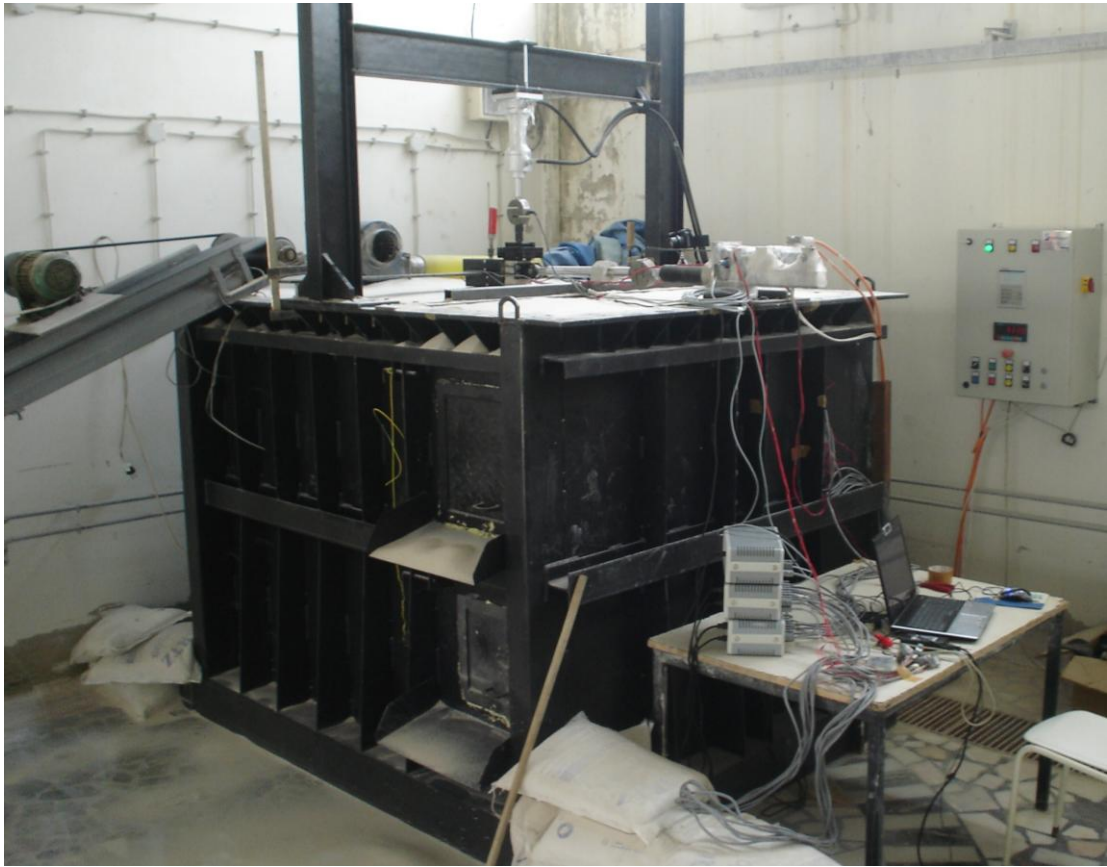
Figure 4.8 Soil-pile interaction test set-up
