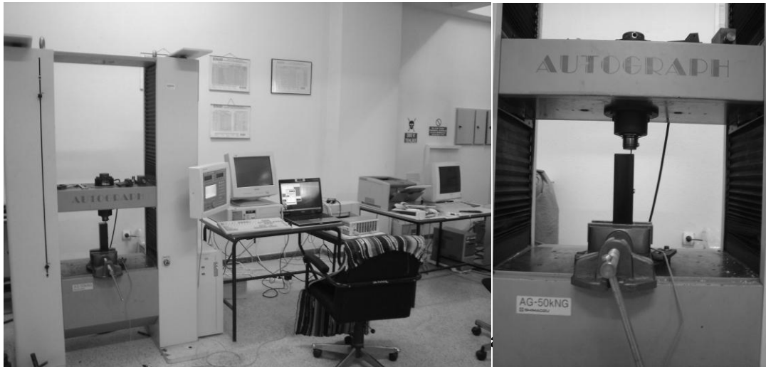
Figure 4.21 Calibration of deformation transducers
