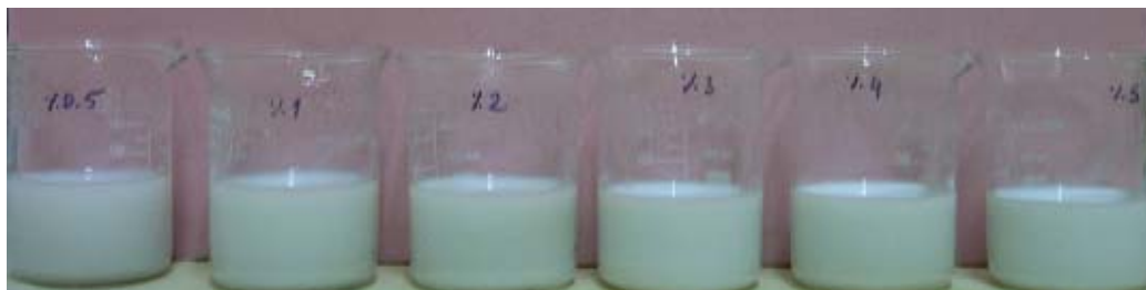
Figure 4.4 Photograph showing a set of produced nanofluids with volume fraction of alumina from 0.5 to 5 vol %.
