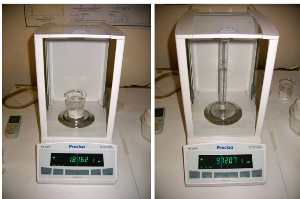
Figure 4.2 Measuring the mass of the particles and liquids by mass balance.
