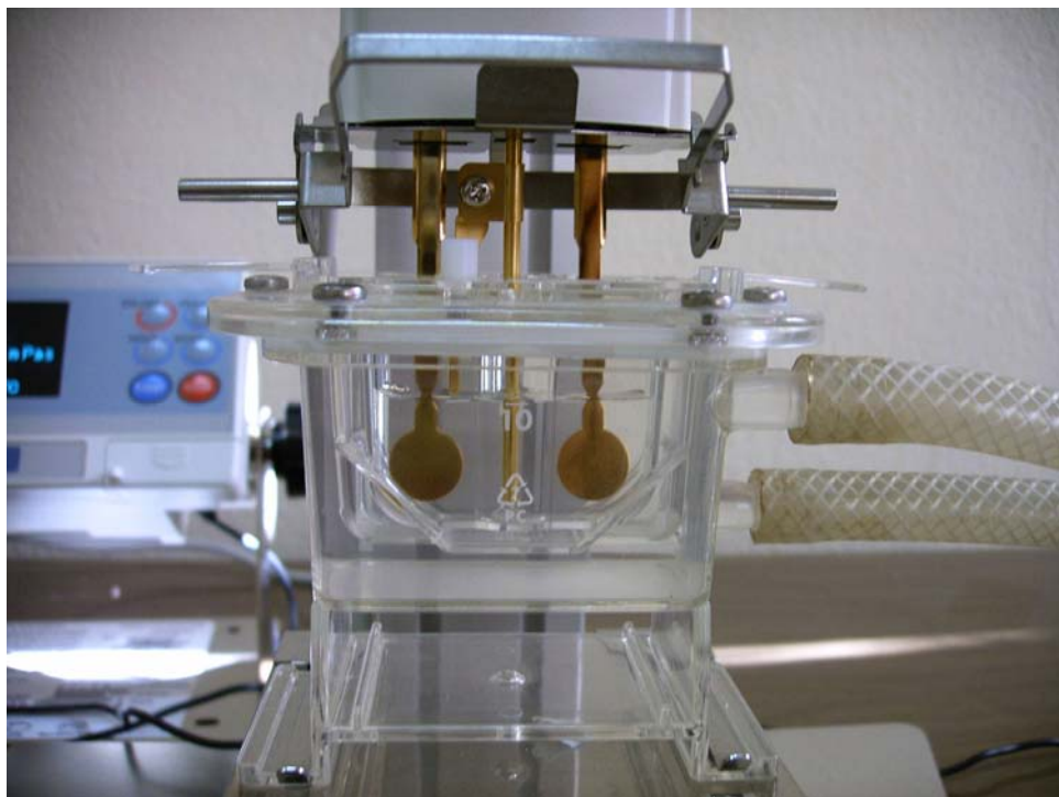
Figure 6.3 Vibrator (sensor plates) and water jacket
