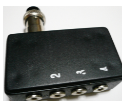
Figure 4.4 Photo of Four Channel microphone apparatus.
