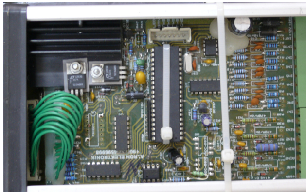
Figure 4.4 Control unit and Drivers located in a box
