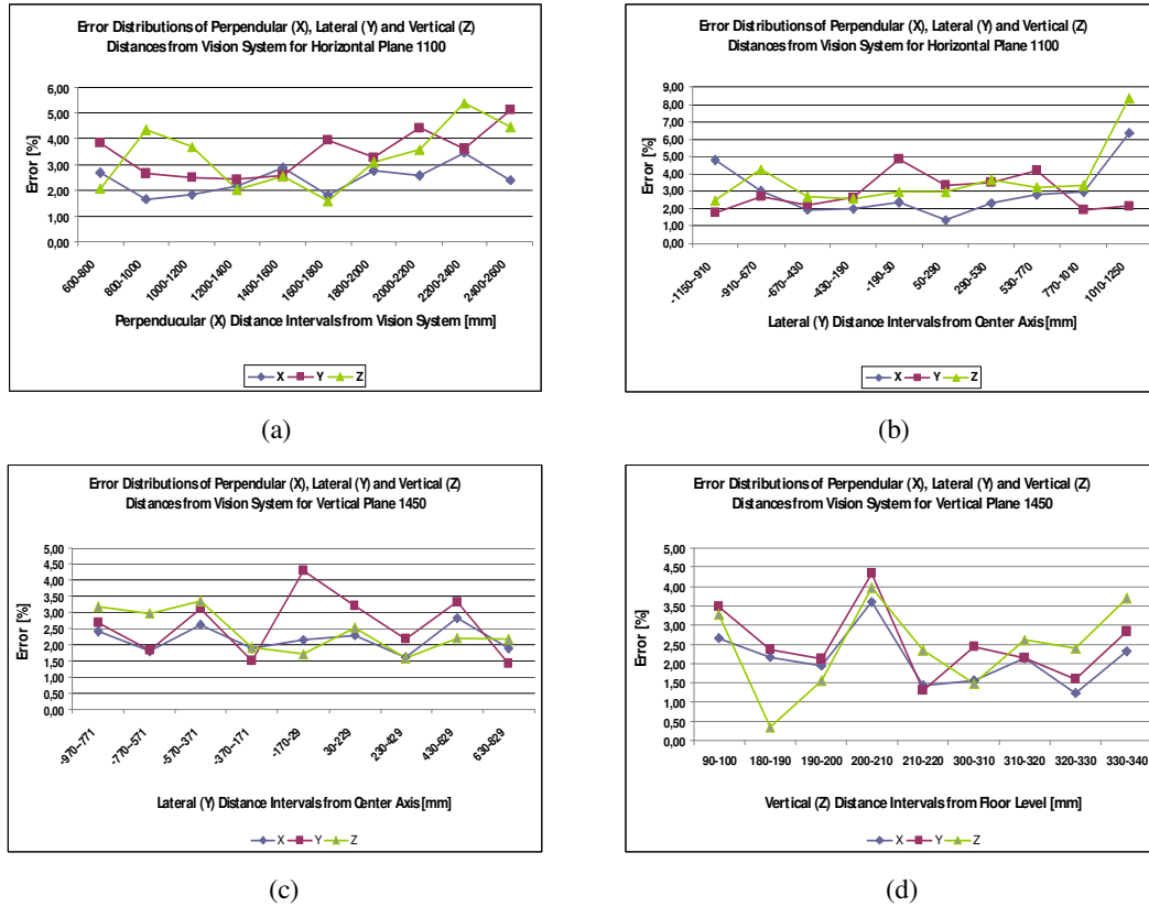
Figure 7.9 Error distributions of horizontal plane 1100 for X (a) and Y (b) intervals; and of vertical plane 1450 for Y (c) and Z (d) intervals
