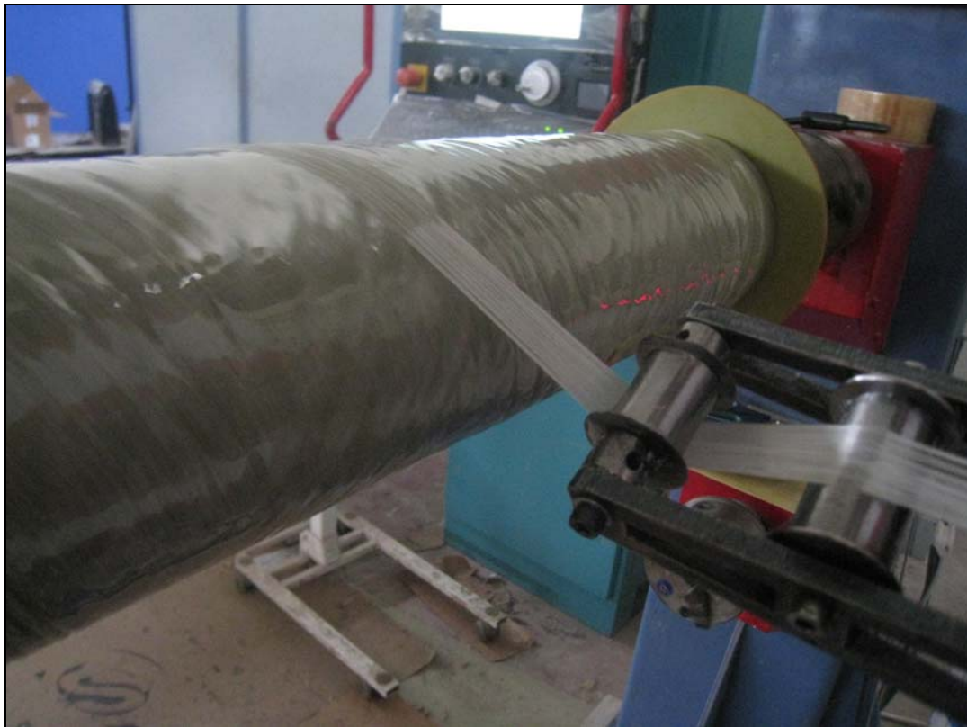
Figure 3.1 CNC filament winding machine and composite pipe
