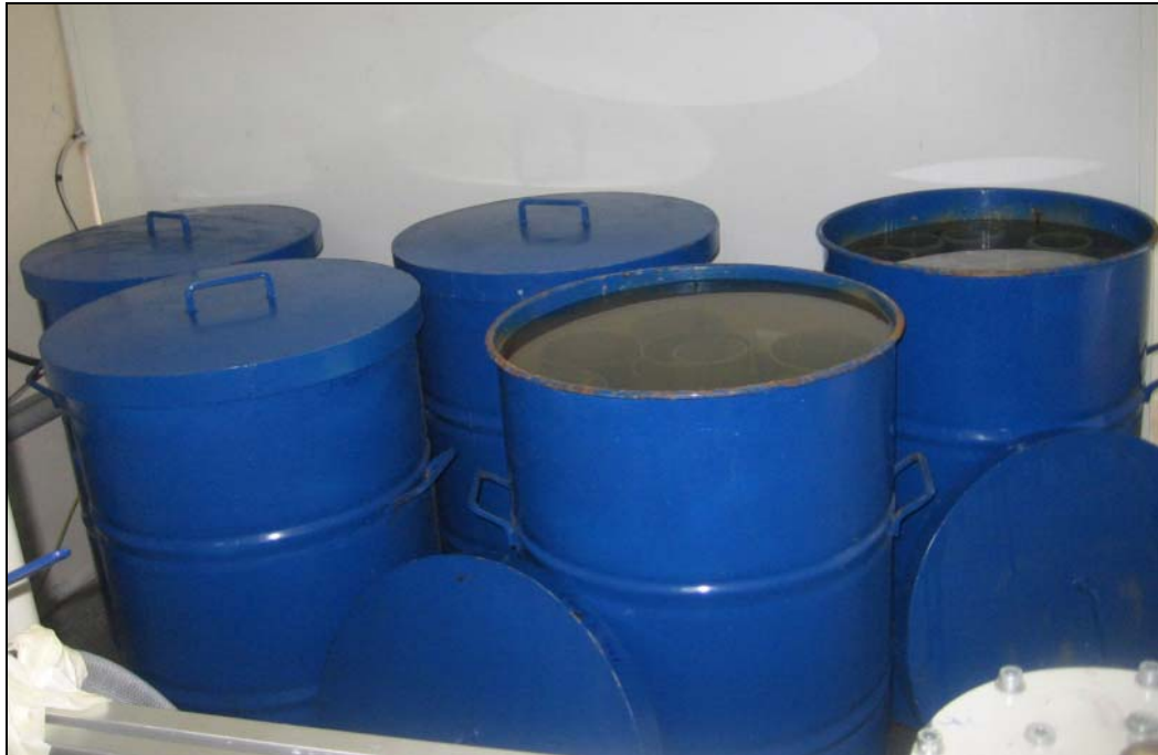
Figure 3.2 Photo of specimens immersed in seawater
