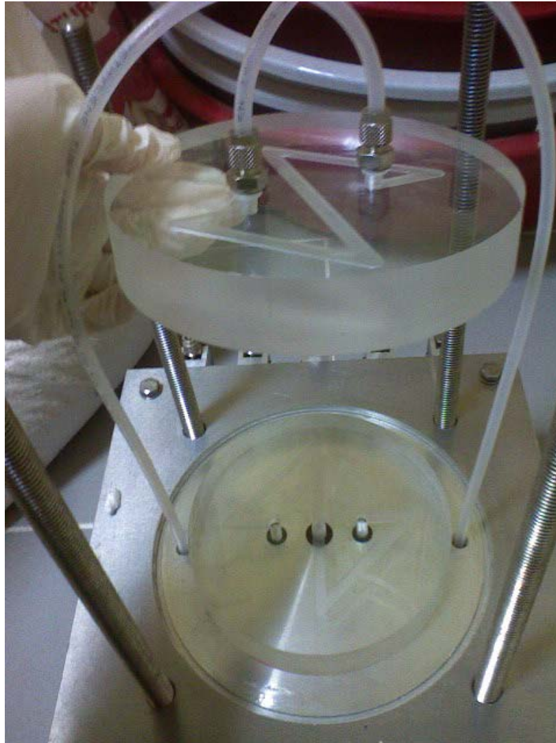
Figure 3.8 A view of the top and bottom plexiglass caps and the tube connections
