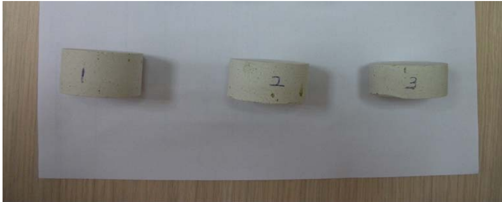
Figure 3.13 Zeolite blocks used in the hydraulic conductivity tests
