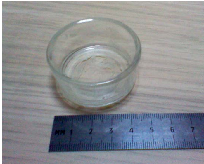
Figure 5.5 Glass mold having a volume of 25 cm 3
