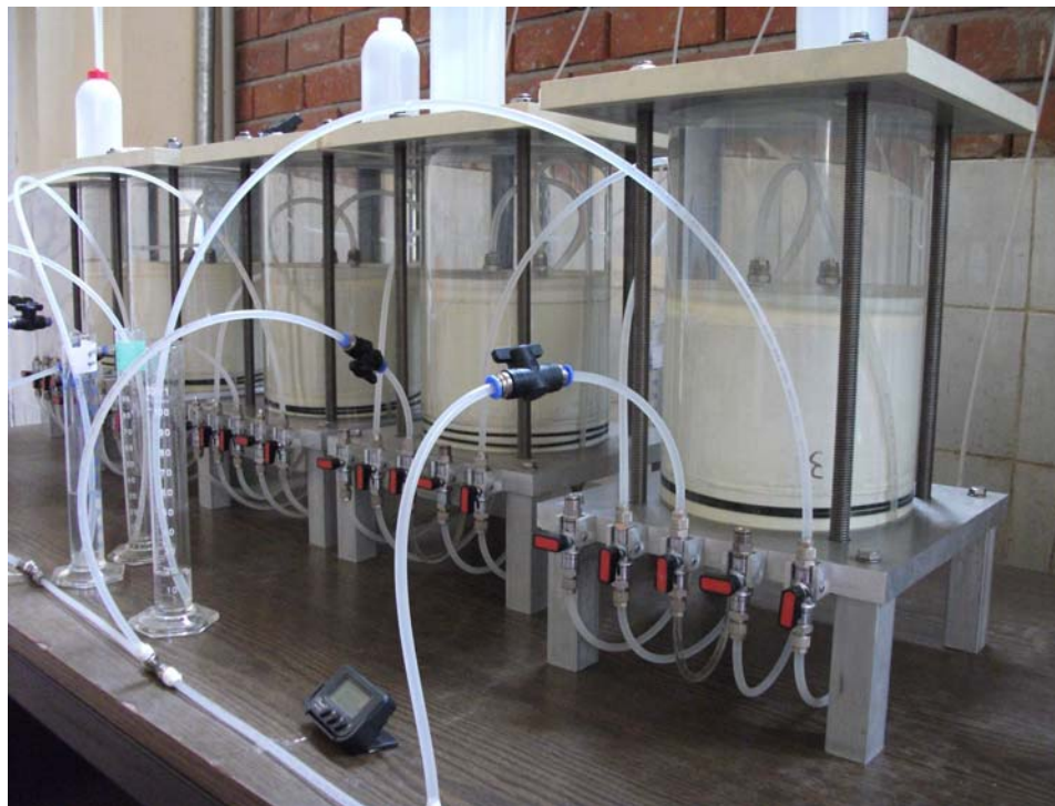
Figure 3.7 Tube connections and flexible wall permeameters through which permeation continues
