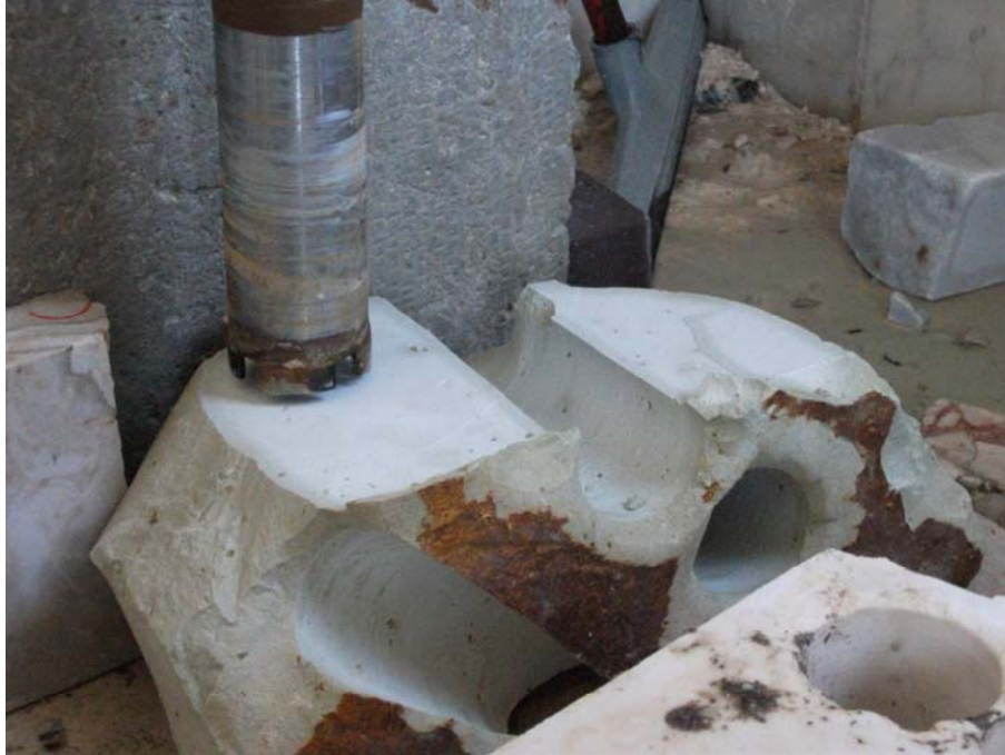
Figure 3.11 Sampling stage of zeolite blocks from different directions
