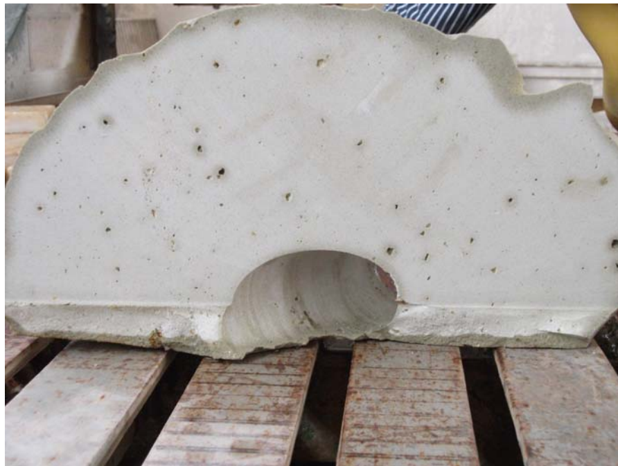
Figure 3.12 Large pores in zeolite block section
