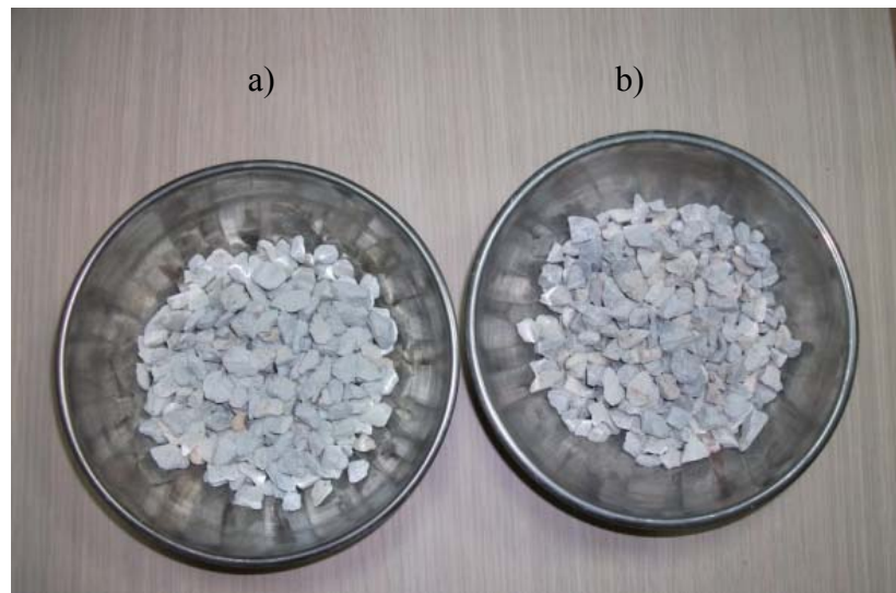
Figure 5.4 Coarse a) zeolite and b) sand samples used in determining the water content distribution tests
