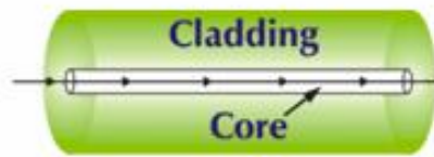
Figure 2.4 Schematic representation of single mode step index fiber.
