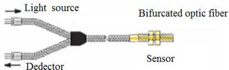
Figure 2.7 Schematic structure of a bifurcated optical fiber.
