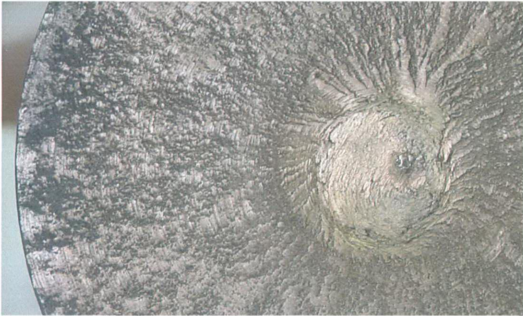
Figure A3 Final fracture zone
