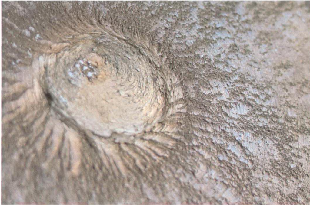
Figure A9 Final fracture zone with shear lips
