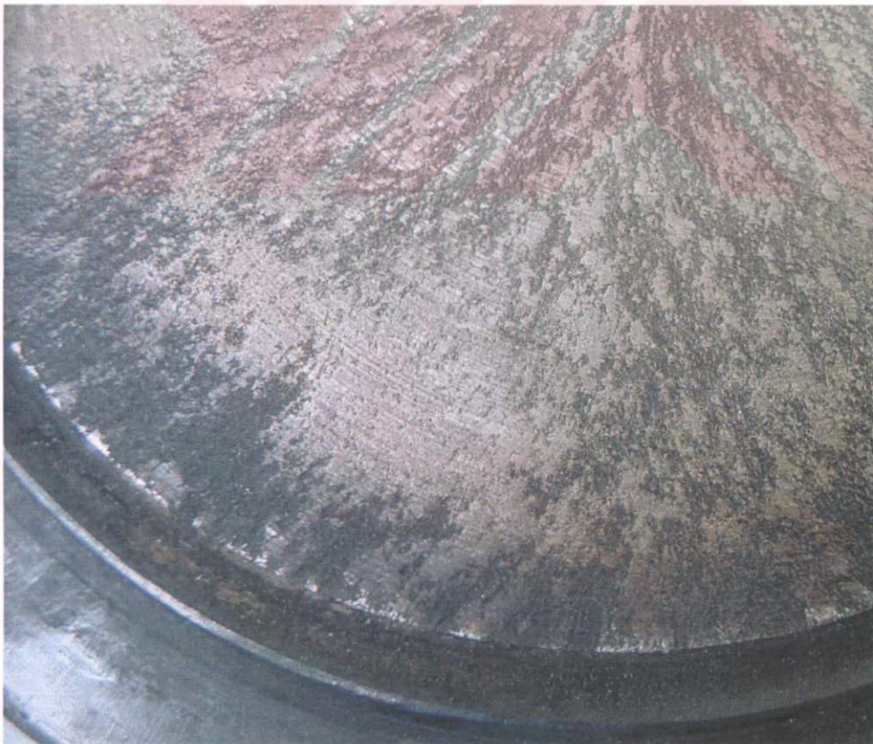
Figure A4 Fibrous zone and beachmarks
