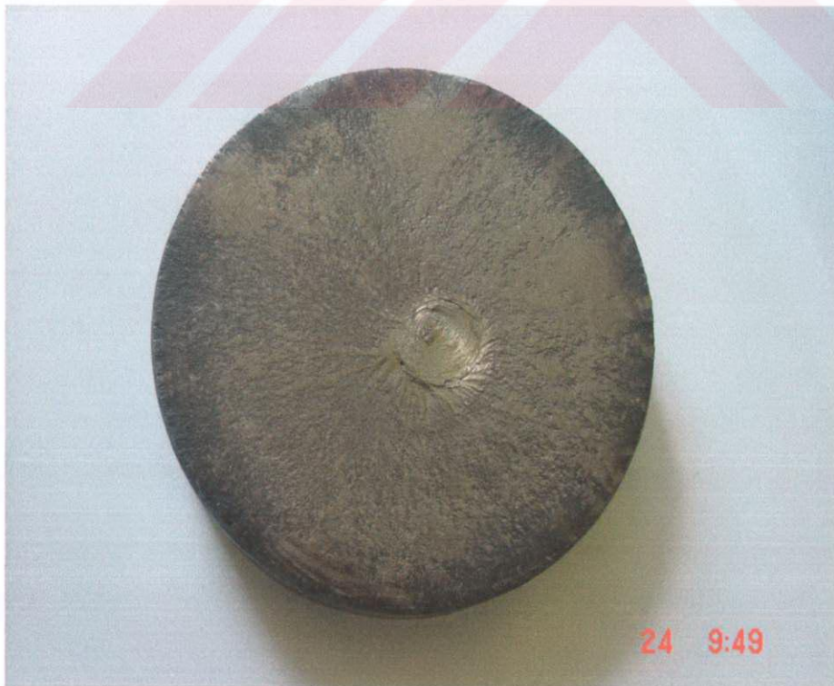
Figure A2 View of the fracture surface (lower side)
