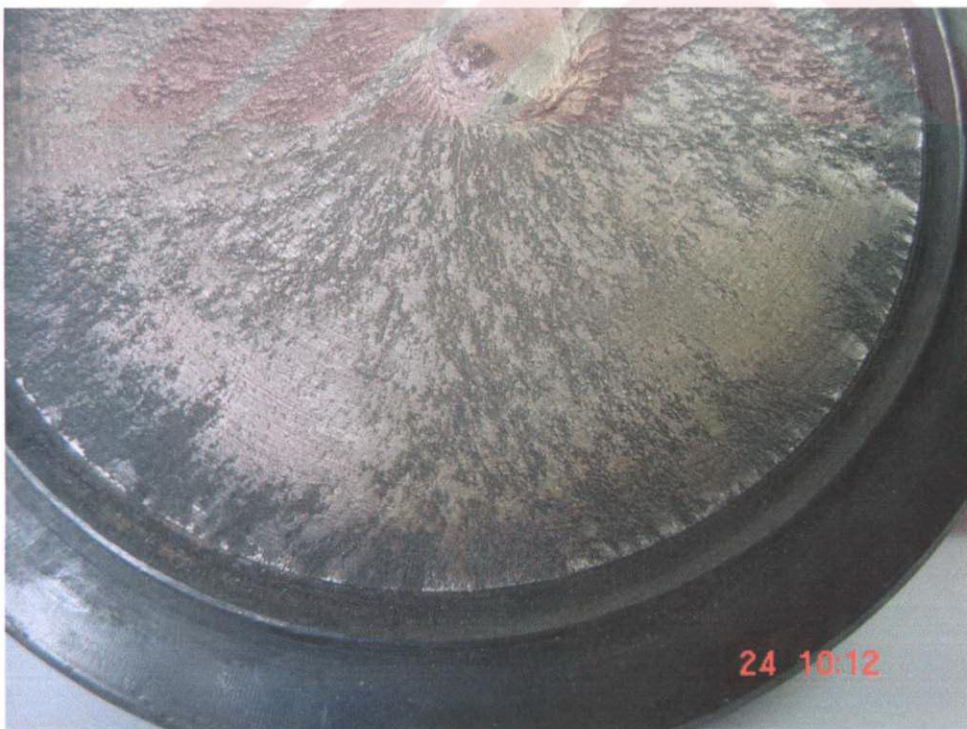
Figure A6 Fibrous zones and radial zones
