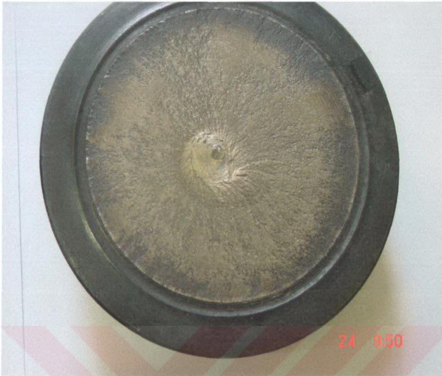
Figure A1 View of the fracture surface (upper side)
