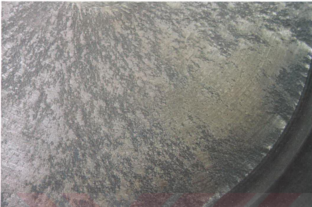
Figure A7 Radial zones showing crack advance direction
