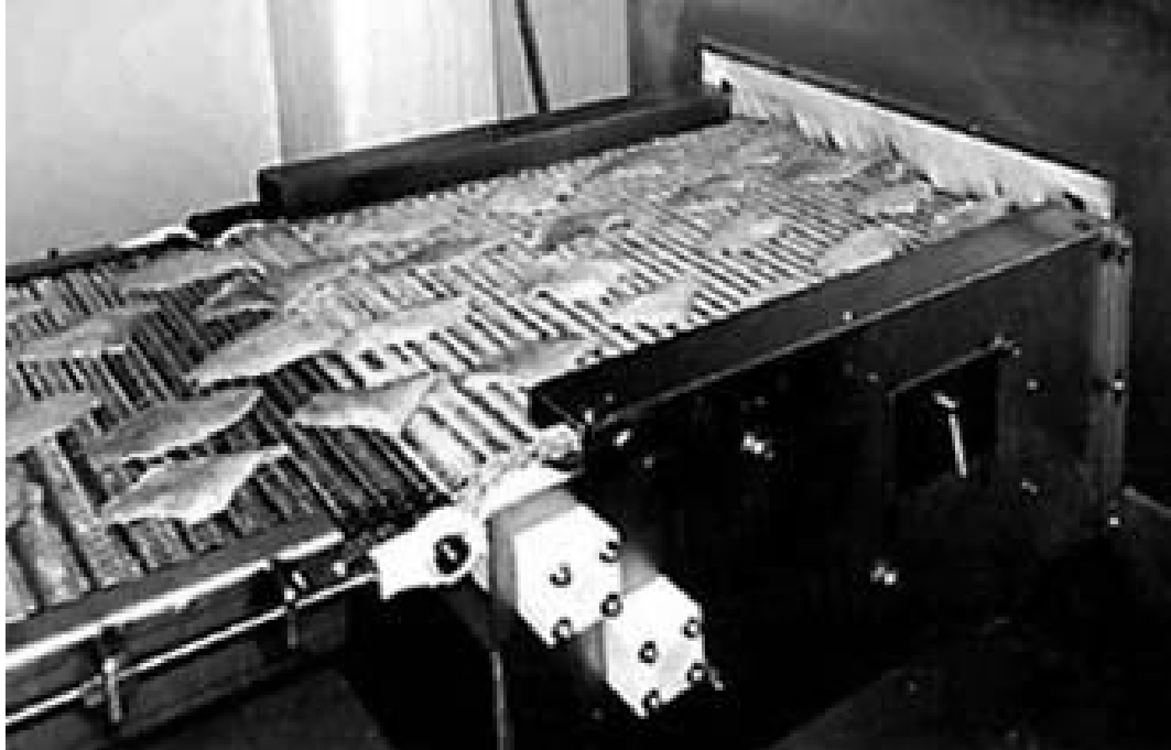
Figure 5.12 Freezing fish in a spiral belt freezer tunnel
