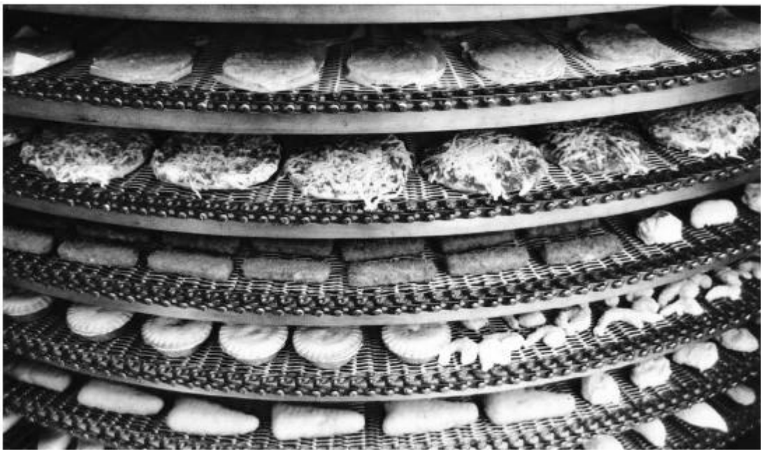
Figure 5.13 Freezing food in a spiral belt freezer tunnel
