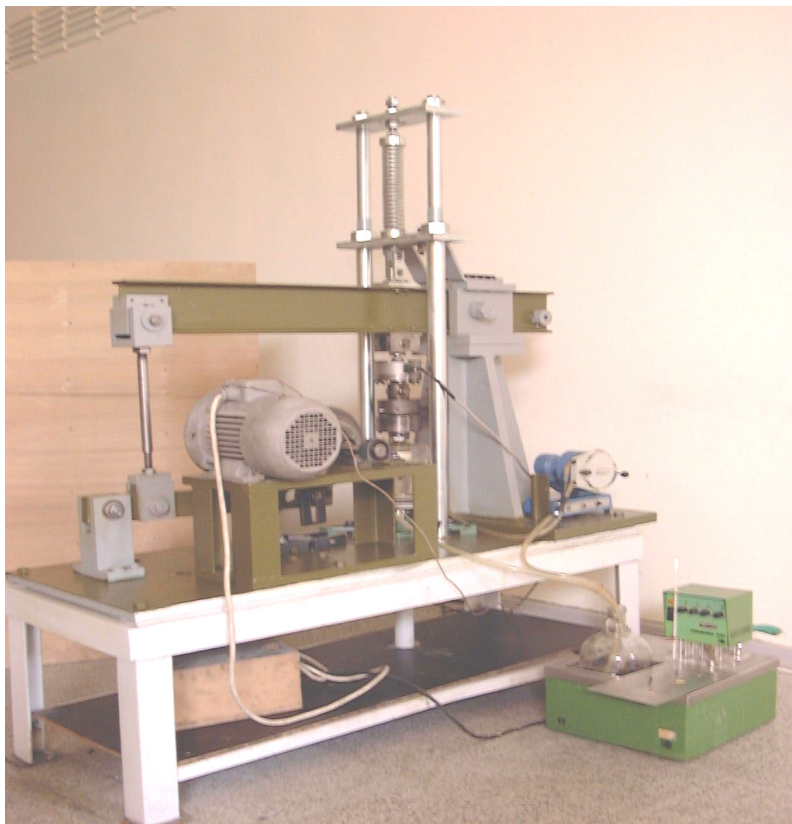
Figure 4.2. Front and back view of the double cantilever beams bending fatigue machine.
