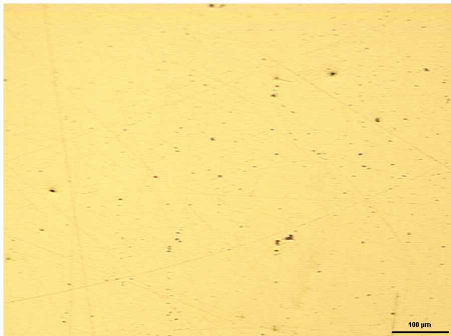
Figure 5.18. Micro structure of the 316L Stainless Steel used for the Hip prosthesis.
