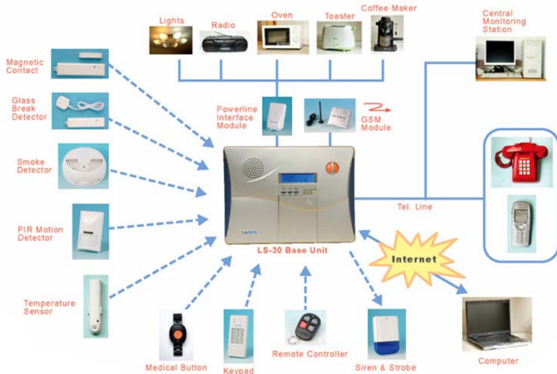
Figure 1.2 A sample home automation system.
