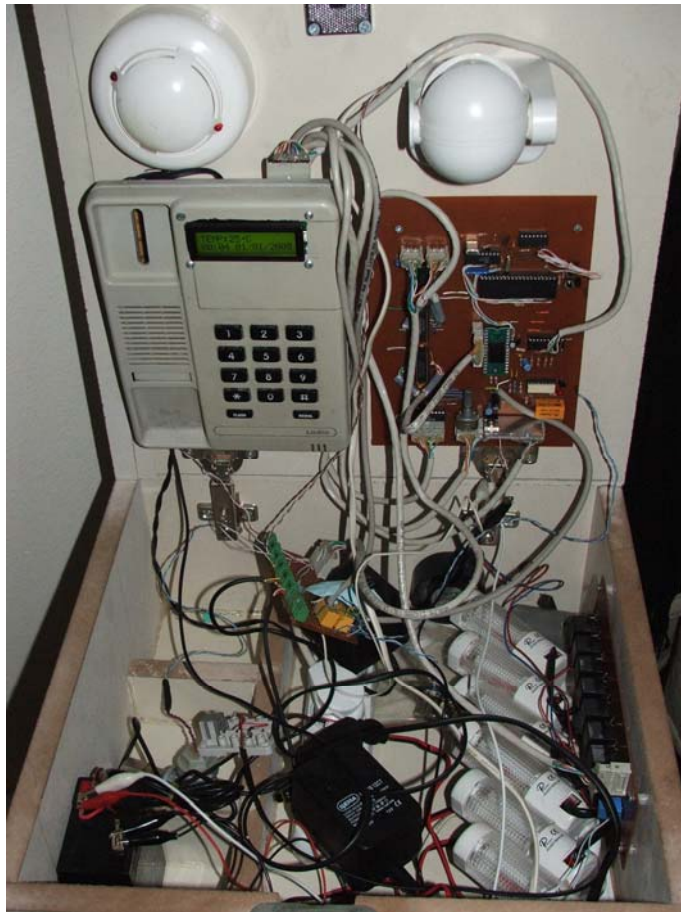
Figure 3.1 Designed Telephone Controlled Home Automation.
