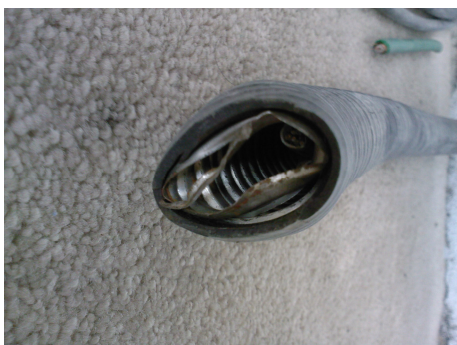
Figure 3.21 Cross section of underground cable
