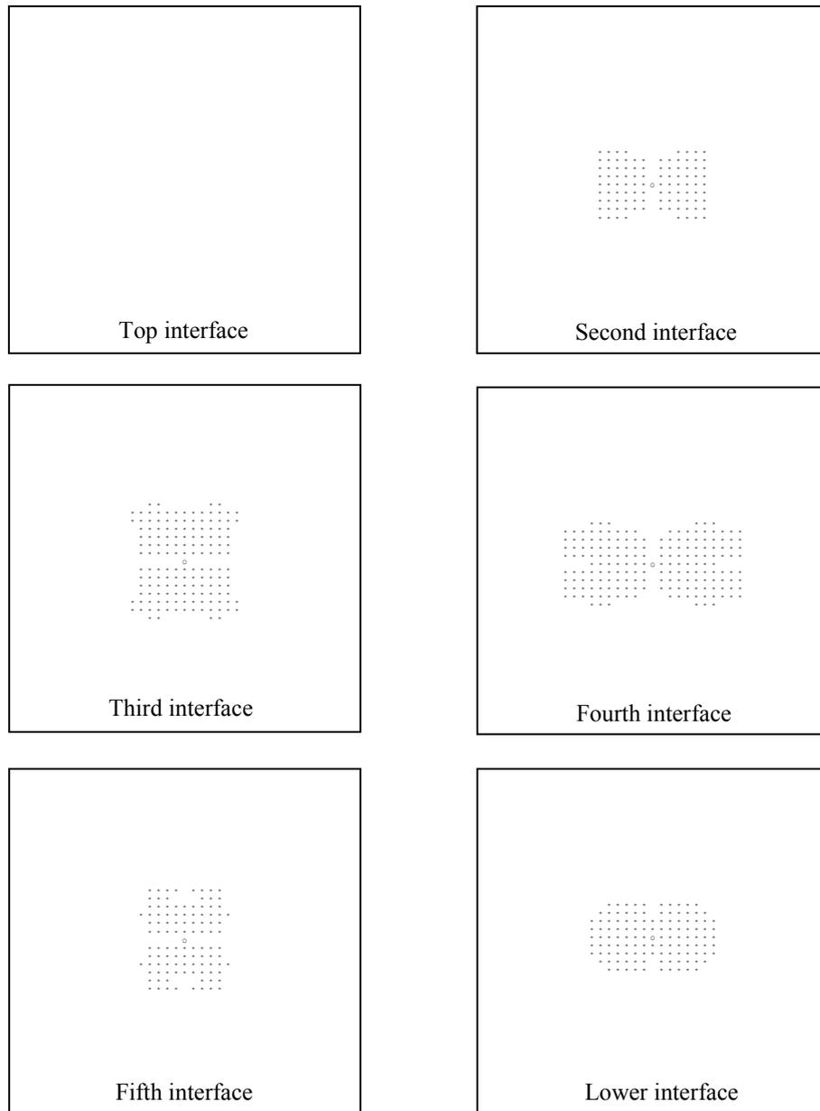
Figure 4.34 Delamination areas between interfaces of 150x150 mm square (10J)
