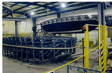
**Top and bottom mold RTM boat hull.**
