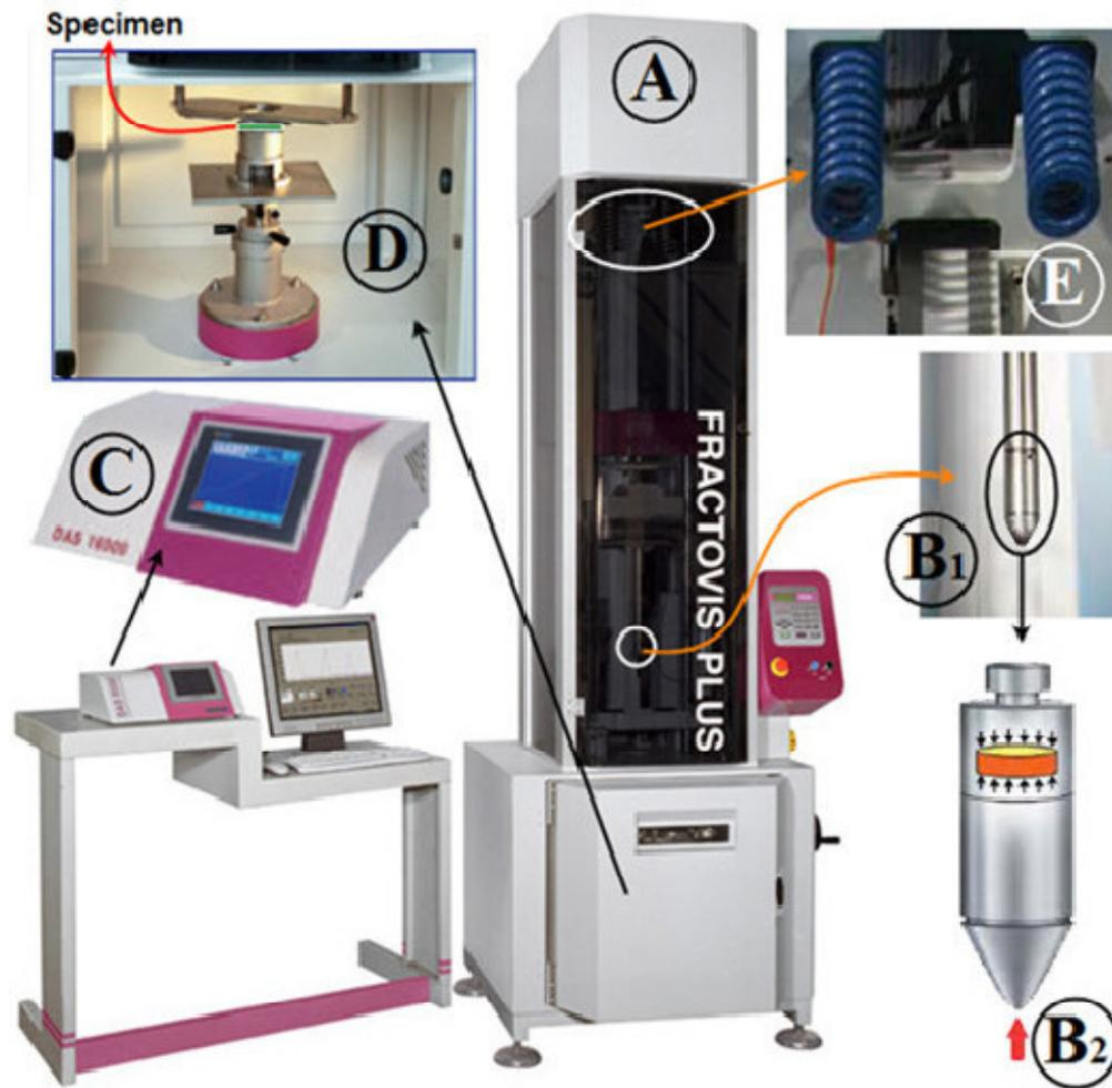
Figure 4.1 Fractovis Plus low velocity impact test machine
