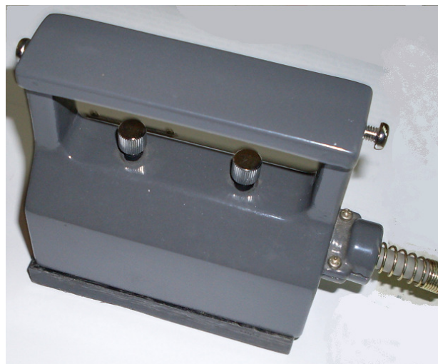
Figure 5.21 Shotherm QTM thermal conductivity meter probe with test specimen under
