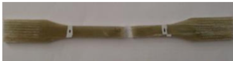
Figure 5.9 Tensile test specimen of E-glass fiber reinforced PP after test
