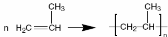
Figure 2.8 Polymerization of propylene to polypropylene (Harper, 2000)
