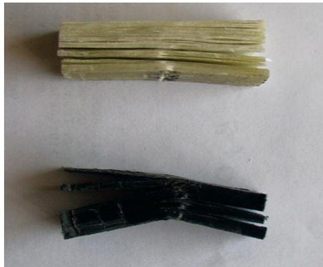
Figure 5.15 Impact test specimens after tests (E - glass and carbon fiber reinforced PP composites)
