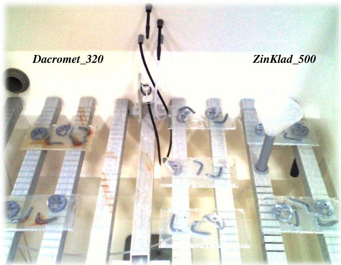
Figure 4.31 Appearance of Dacromet_320 and ZinKlad_500 samples after 248 hours NSS test
