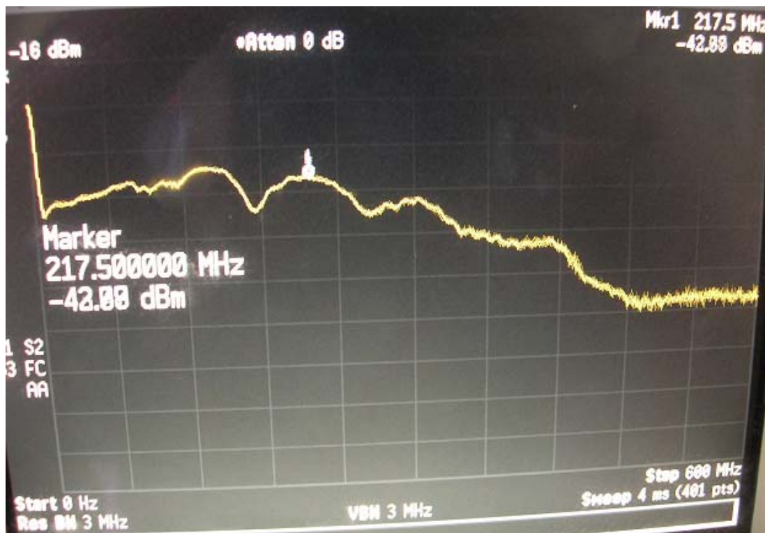
Figure 3.8 Spectrum analyzer output of transmitted signal
