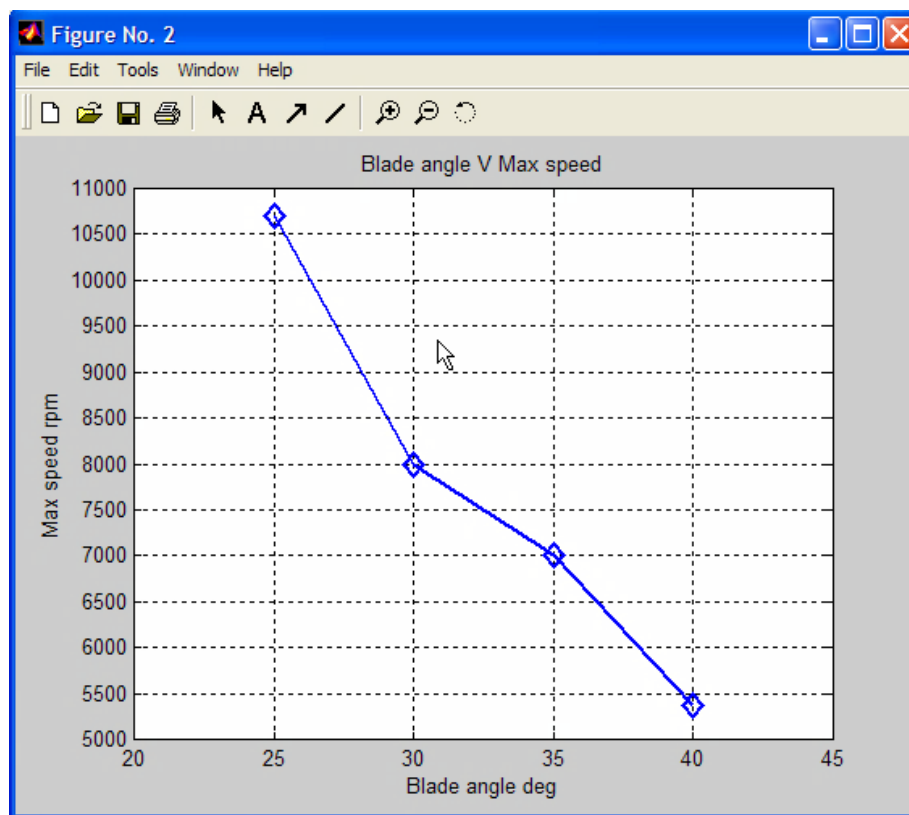
Figure 4.6 Max rpm for various blade angles.
