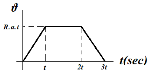
Figure 9.3 Trapezoidal velocity profile for the head's linear motion
