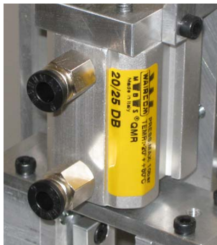
Figure 9.11 Selected pneumatic cylinder for gripper holding
