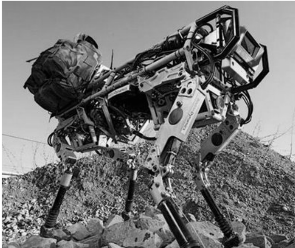
Figure 6.7 Boston Dynamics “BigDog” billed as the most advanced quadruped robot on Earth, which is able to carry up four packs of military equipment on awkward terrain unsuitable for vehicles. BigDog is powered by an engine that drives a hydraulic actuation system
