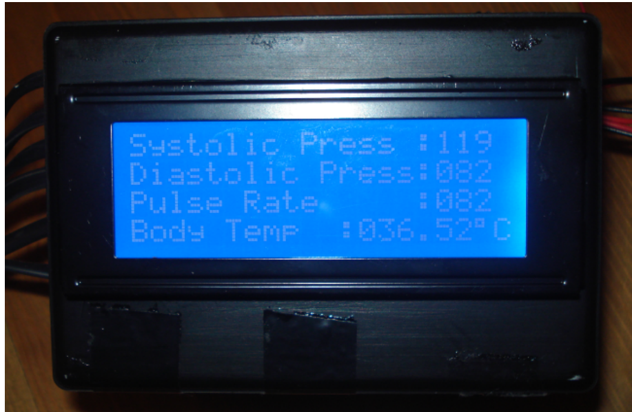
Figure 5.12-a First measurement results on the LCD of the transmitter part after set values were changed
