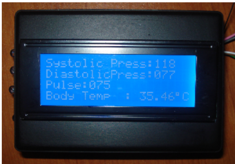
Figure 5.8-b Measurement results on the LCD of the receiver part after the 3rd measurement
