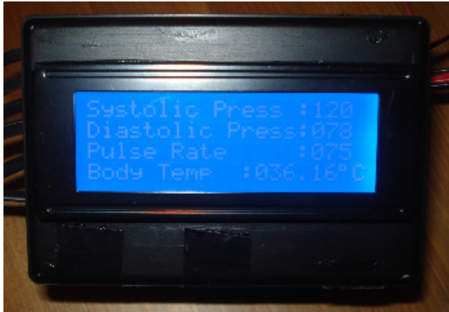
Figure 5.10-a Measurement results on the LCD of the transmitter part after the 5th measurement
