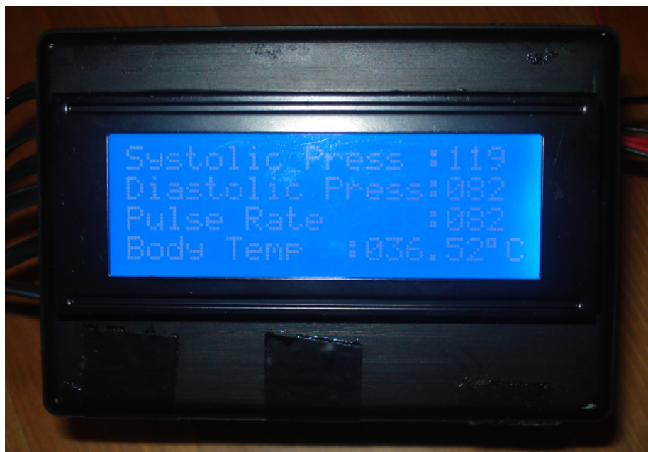
Figure 5.13-a Second measurement results on the LCD of the transmitter part after set values were changed
