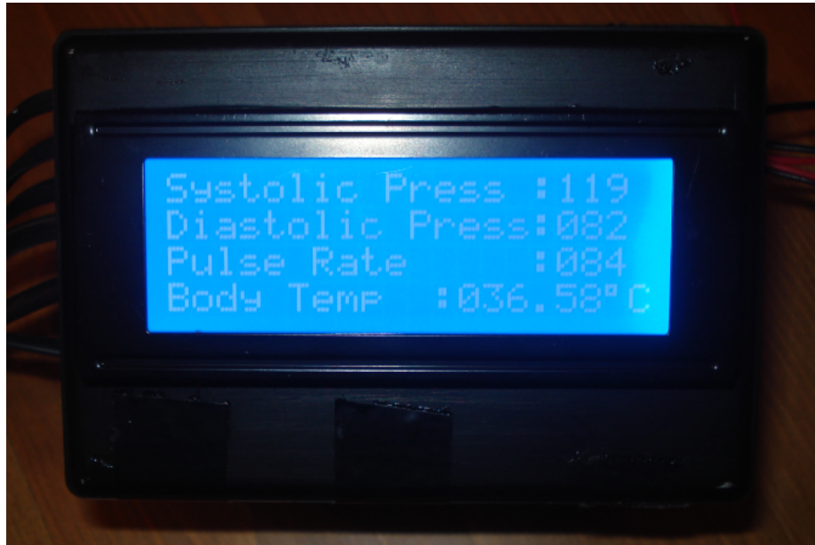
Figure 5.14-a Third measurement results on the LCD of the transmitter part after set values were changed
