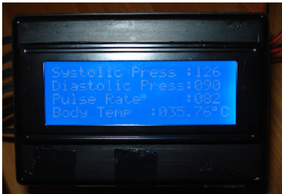
Figure 5.17-a Second measurement results on the LCD of the transmitter part after changing the set values in each step
