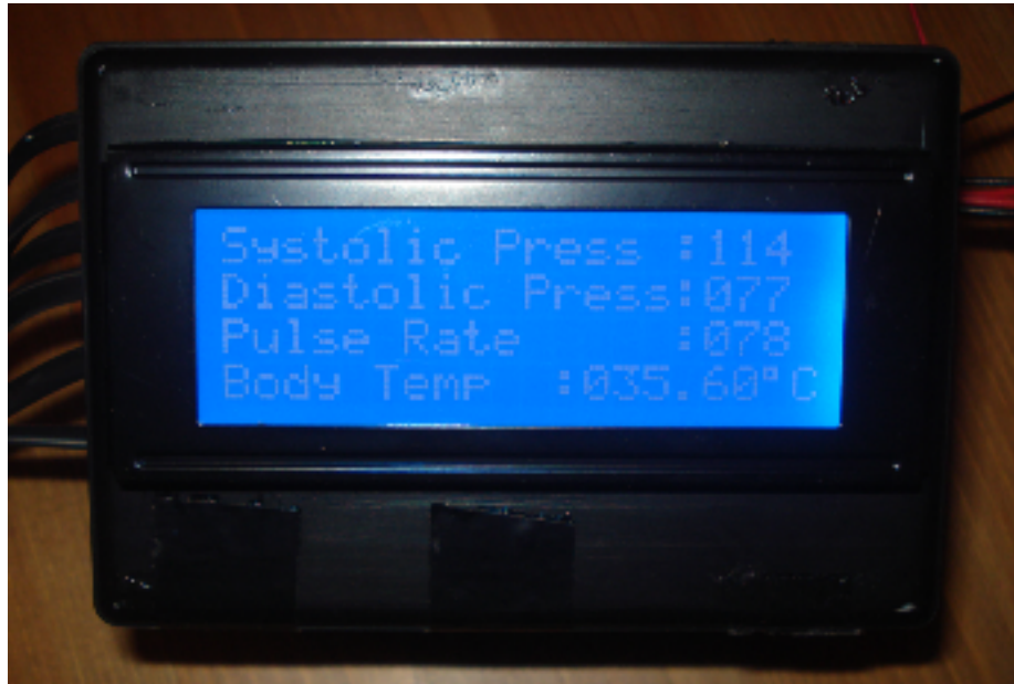
Figure 5.7-a Measurement results on the LCD of the transmitter part after the 2nd measurement
