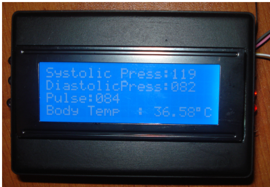
Figure 5.14-b Third measurement results on the LCD of the receiver part after set values were changed
