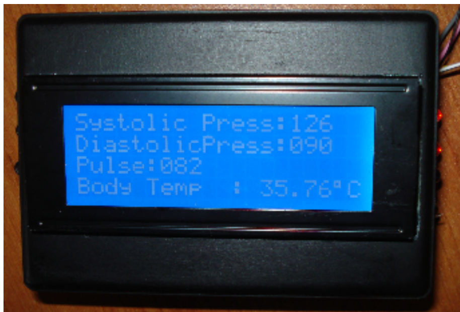
Figure 5.17-b Second measurement results on the LCD of the receiver part after changing the set values in each step
