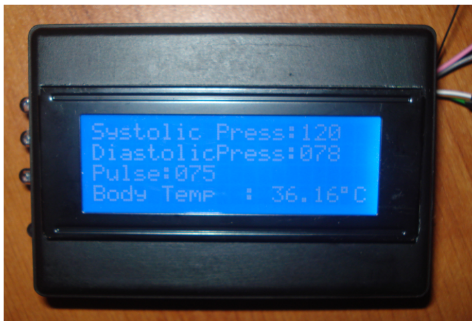
Figure 5.10-b Measurement results on the LCD of the receiver part after the 5th measurement
