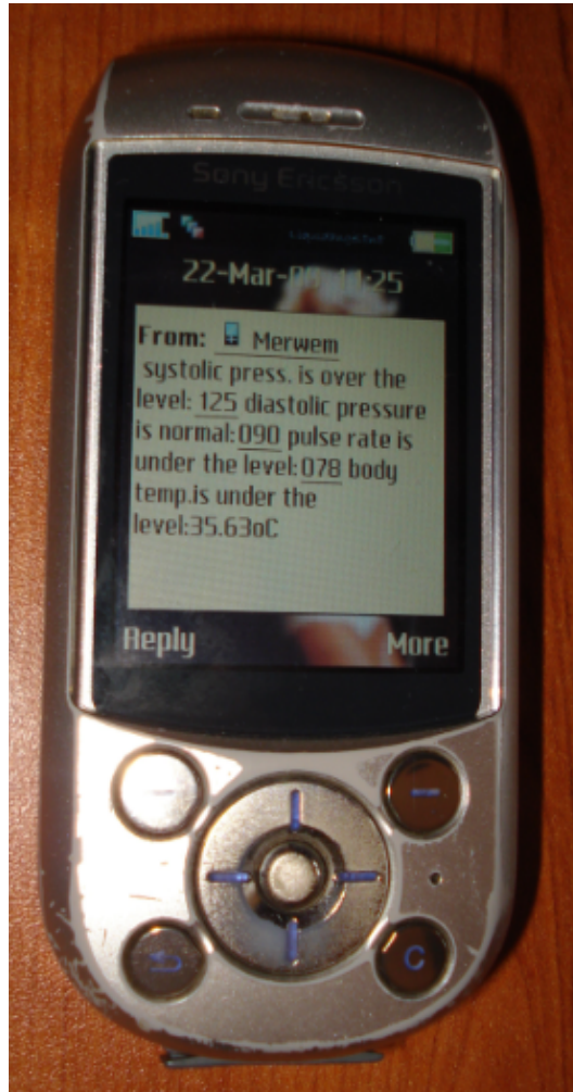
Figure 5.16-d First measurement results on the mobile phone after set values were exceeded
