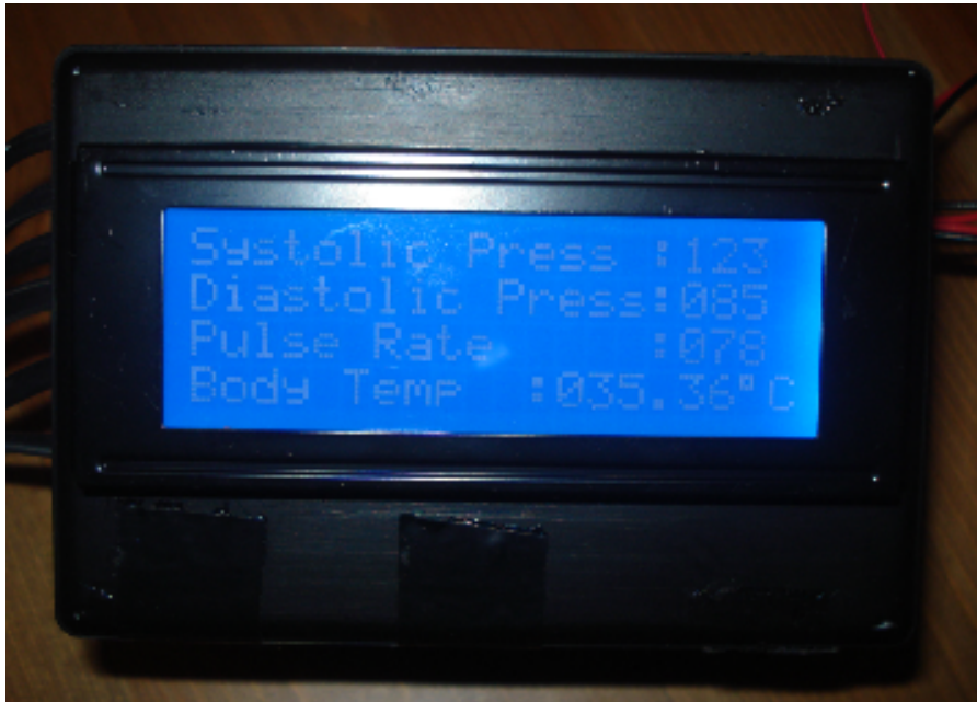
Figure 5.5-a Measurement results on the LCD of the transmitter part when “START” button was pushed
