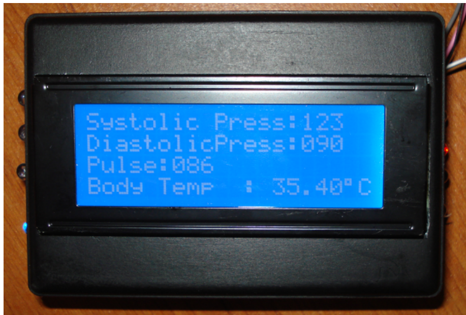
Figure 5.21-b Sixth measurement results on the LCD of the receiver part after changing the set values in each step
