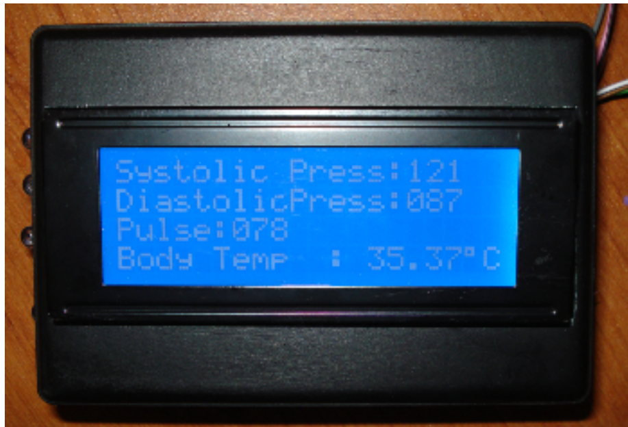
Figure 5.20-b Fifth measurement results on the LCD of the receiver part after changing the set values in each step
