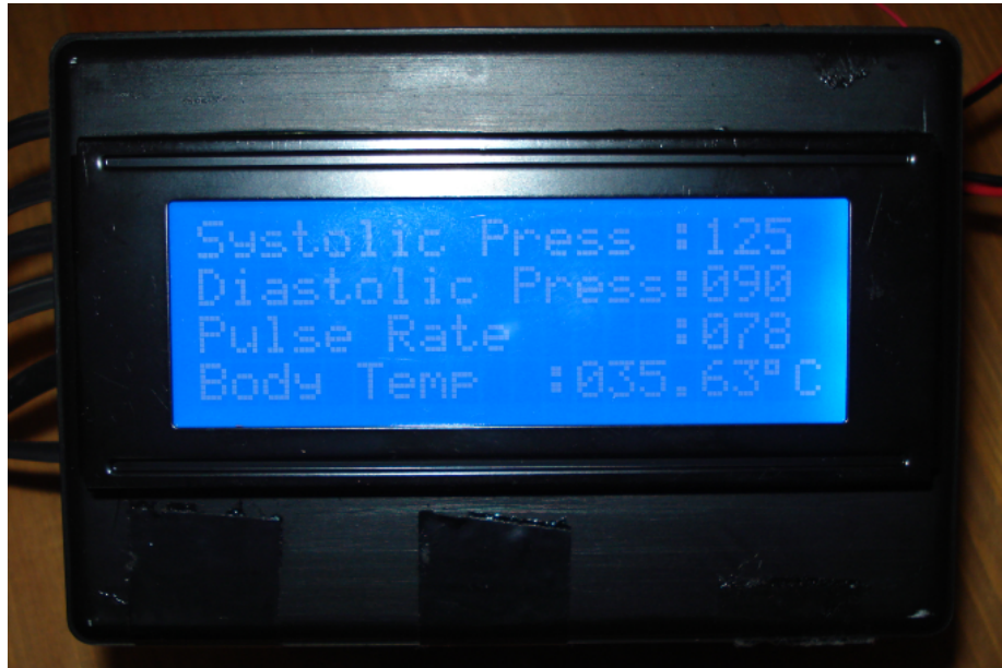
Figure 5.16-a First measurement results on the LCD of the transmitter part after changing the set values in each step
