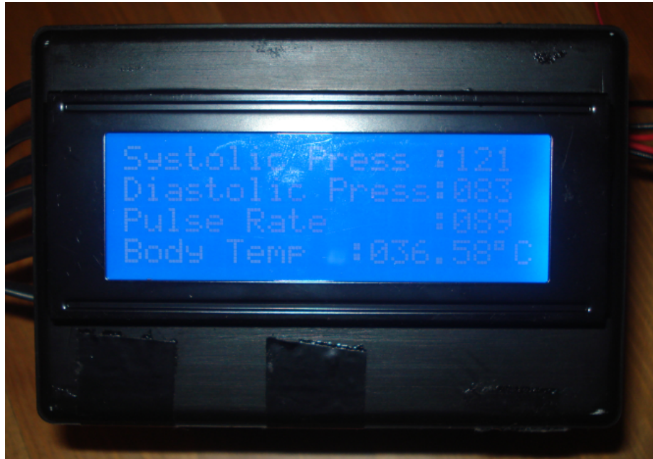
Figure 5.15-a Fourth measurement results on the LCD of the transmitter part after set values were changed
