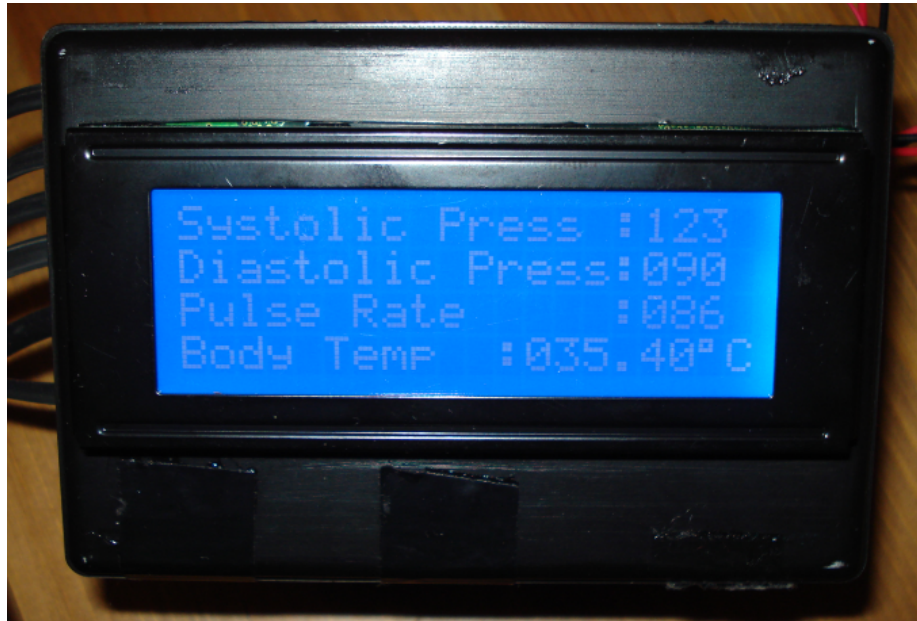
Figure 5.21-a Sixth measurement results on the LCD of the transmitter part after changing the set values in each step
