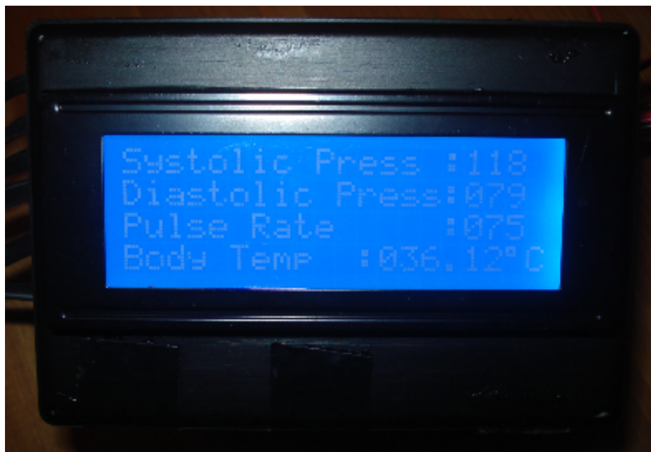
Figure 5.9-a Measurement results on the LCD of the transmitter part after the 4th measurement
