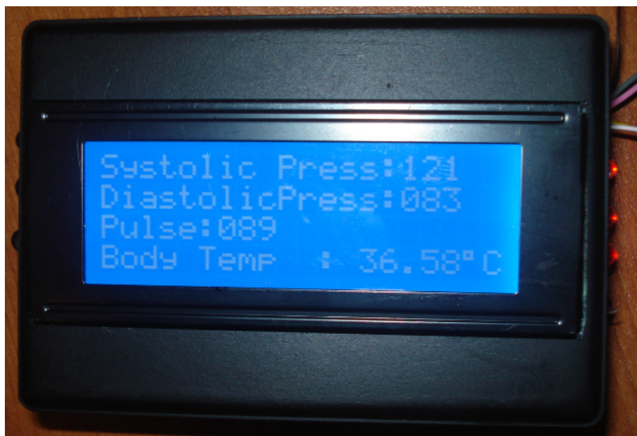
Figure 5.15-b Fourth measurement results on the LCD of the receiver part after set values were changed
