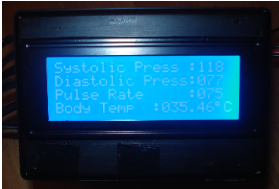
Figure 5.8-a Measurement results on the LCD of the transmitter part after the 3rd measurement
