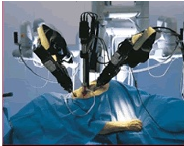
Figure 2.4 The da Vinci robot consisting of two manipulation arms and one camera arm (Mantas J.G. & Petropoulu S.G., 2005)
