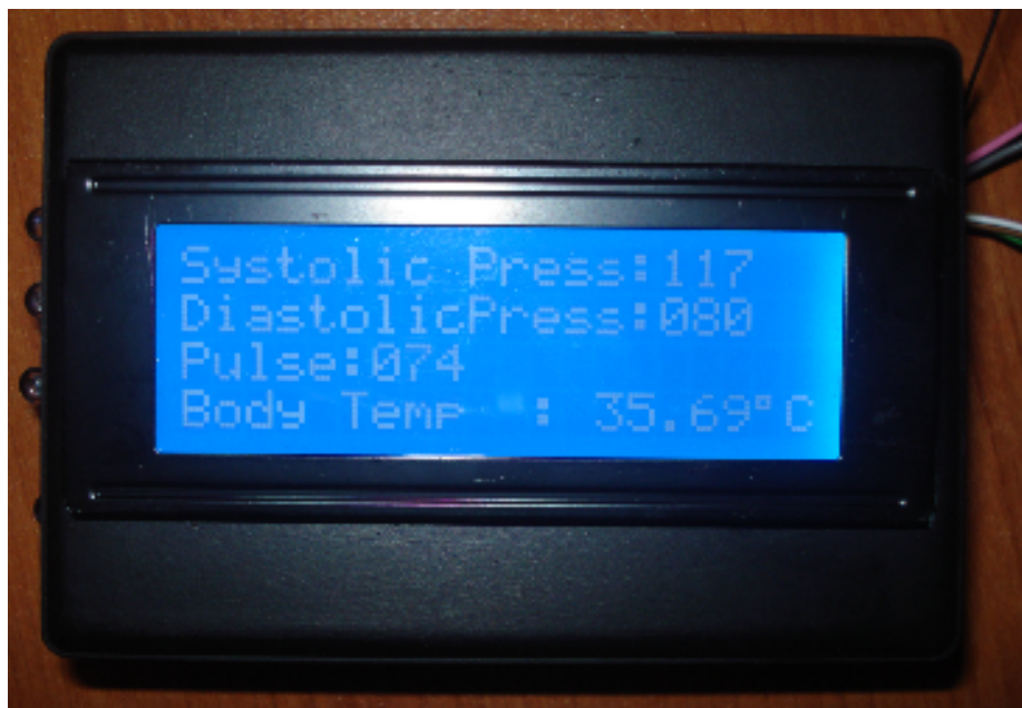
Figure 5.6-b Measurement results on the LCD of the receiver part after the 1st measurement
