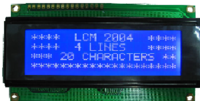
Figure 3.16 Four lines, twenty characters liquid crystal display
