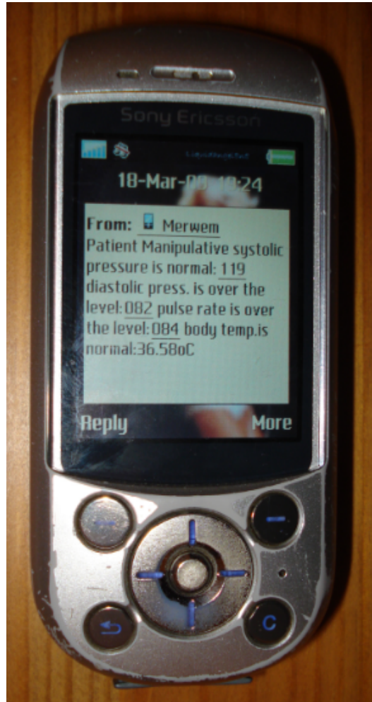
Figure 5.14-d Third measurement results on the mobile phone after the values were exceeded
