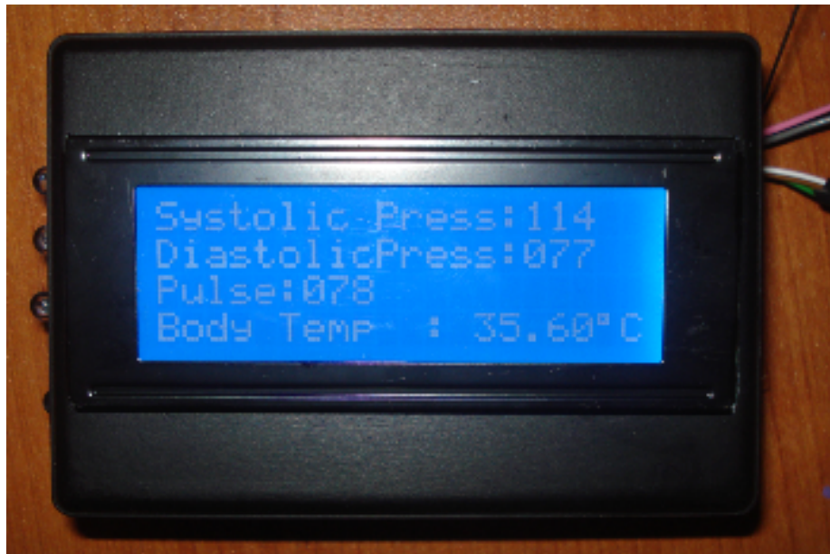
Figure 5.7-b Measurement results on the LCD of the receiver part after the 2nd measurement
