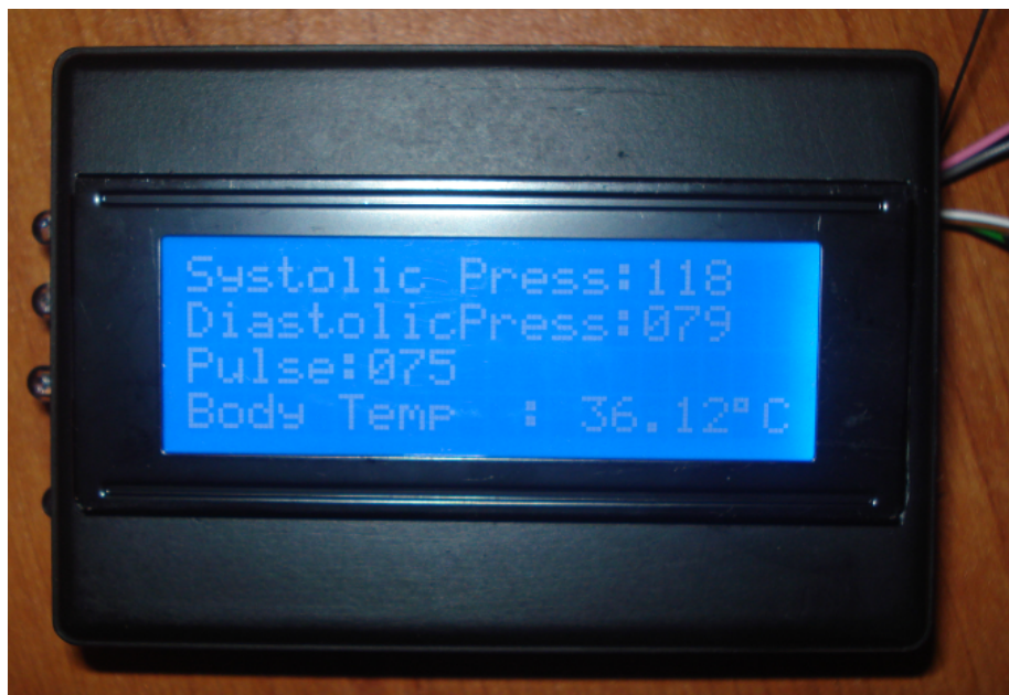
Figure 5.9-b Measurement results on the LCD of the receiver part after the 4th measurement
