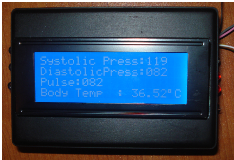
Figure 5.13-b Second measurement results on the LCD of the receiver part after set values were changed
