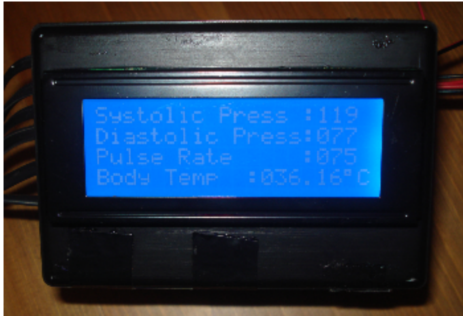
Figure 5.11-a Measurement results on the LCD of the transmitter part after the 6th measurement
