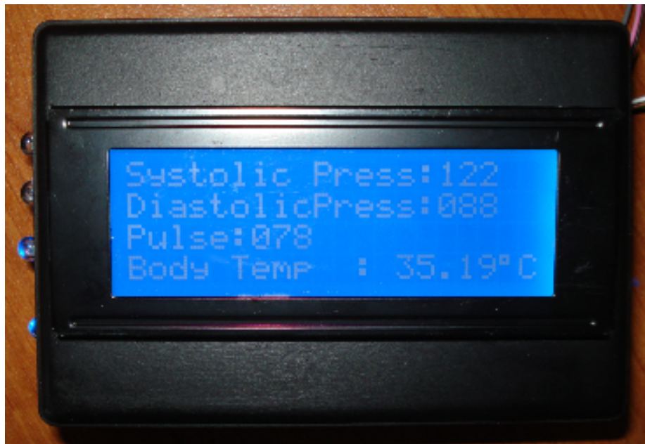
Figure 5.18-b Third measurement results on the LCD of the receiver part after changing the set values in each step
