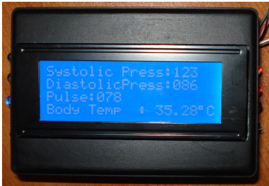
Figure 5.19-b Fourth measurement results on the LCD of the receiver part after changing the set values in each step
