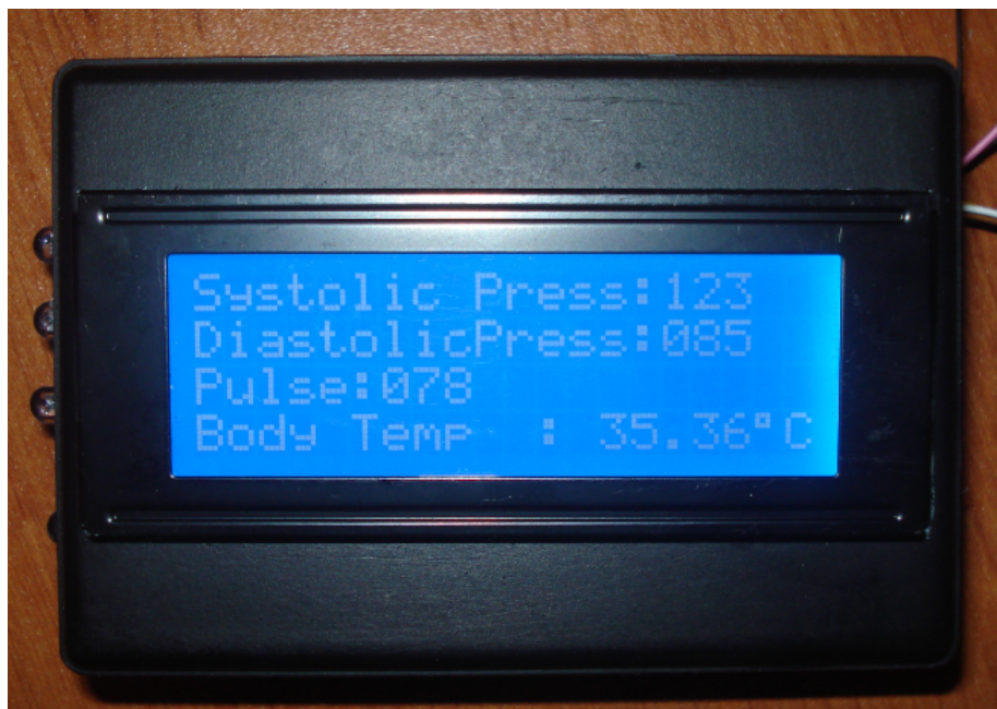
Figure 5.5-b Measurement results on the LCD of the receiver part when “START” button was pushed
