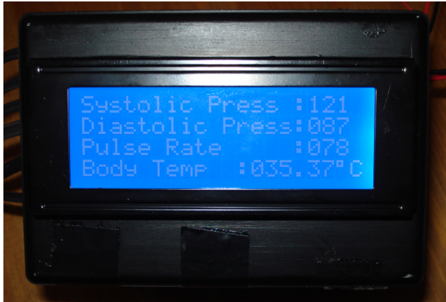
Figure 5.20-a Fifth measurement results on the LCD of the transmitter part after changing the set values in each step
