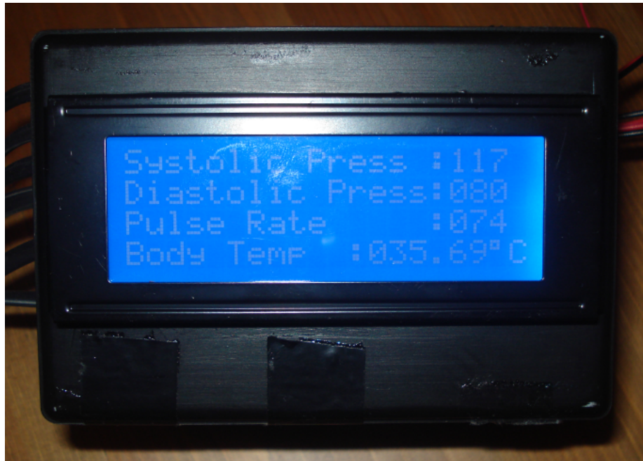
Figure 5.6-a Measurement results on the LCD of the transmitter part after the 1st measurement
