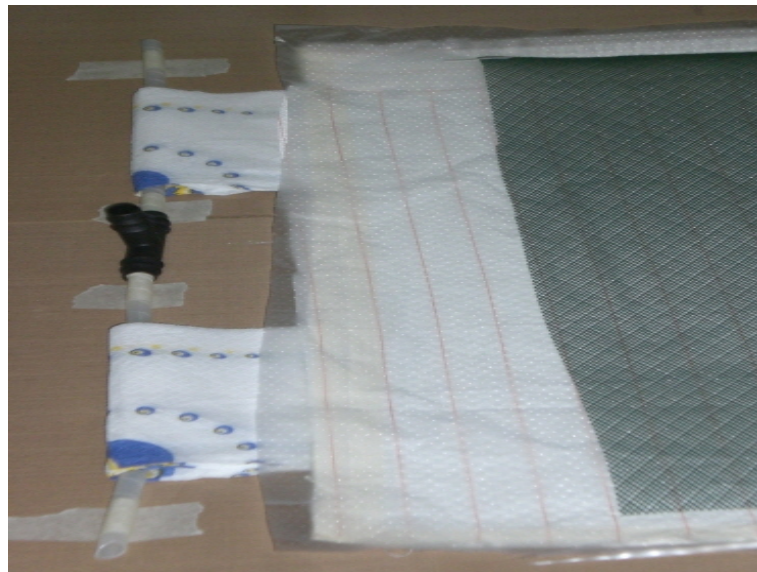
Figure 4.14 “T” pipe and spiral hoses placed on the table
