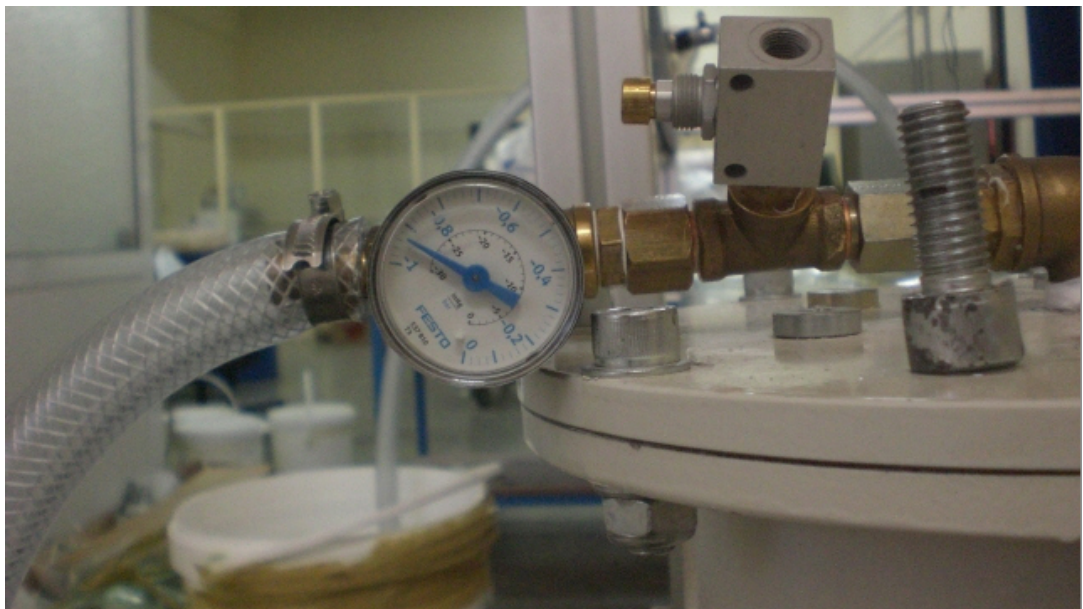
Figure 4.22 Vacuum pressure indicator
