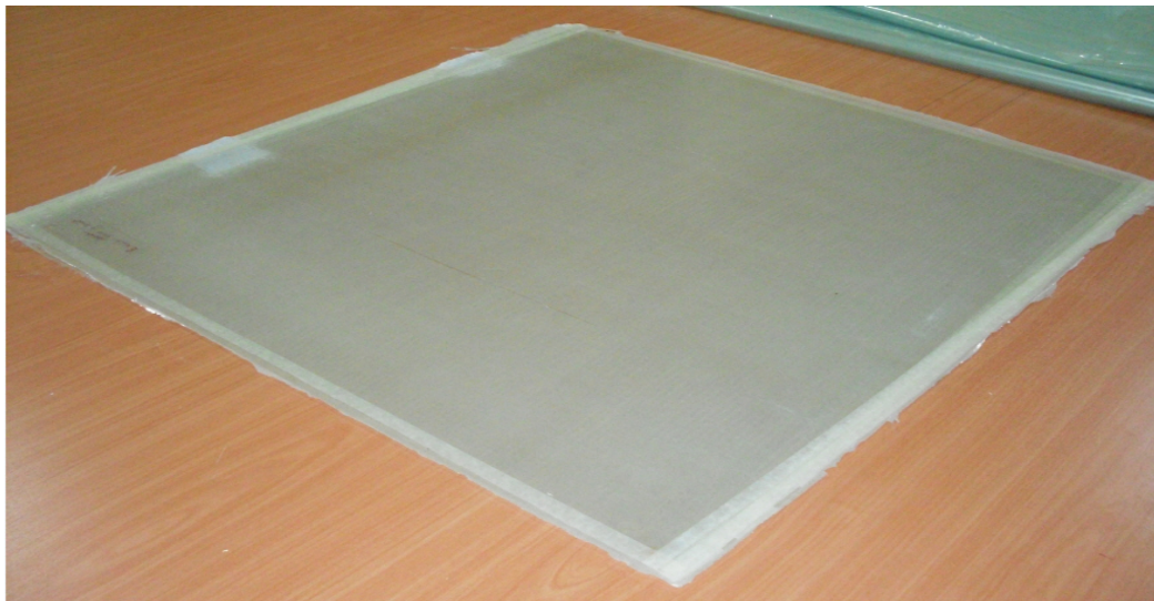
Figure 4.27 The final appearance of the composite plate that is manufactured by VARIM method
