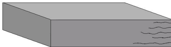
Figure 3.4 Laminate splitting in a laminated composite
