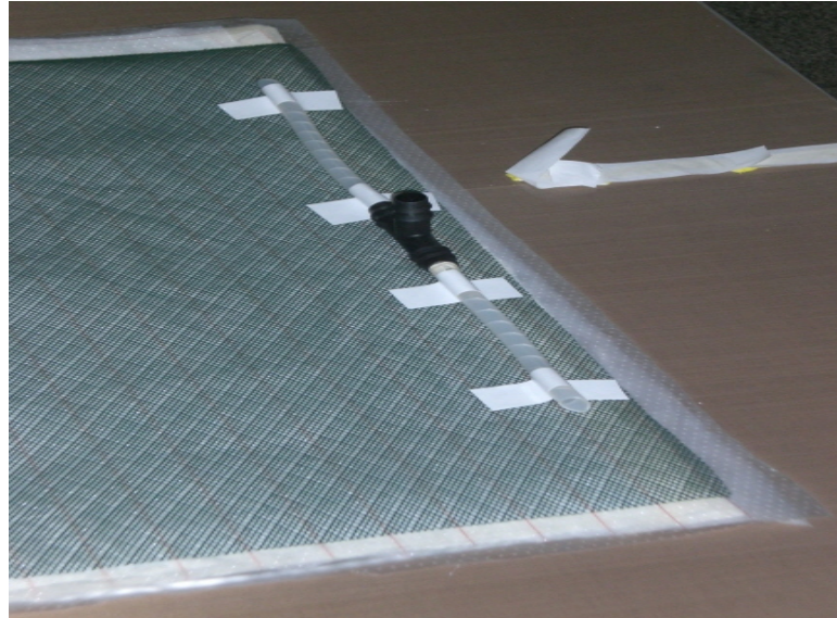
Figure 4.13 The T pipe and spiral hoses placed on the right part of resin distribution medium.
