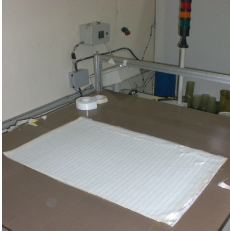
Figure 4.9 Peel ply placed on fiber plies
