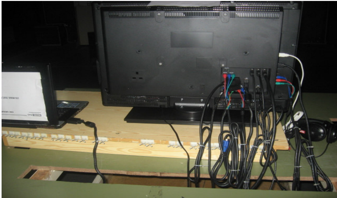
Figure 3.10 All ports are terminated with suitable cables in EN 55022
