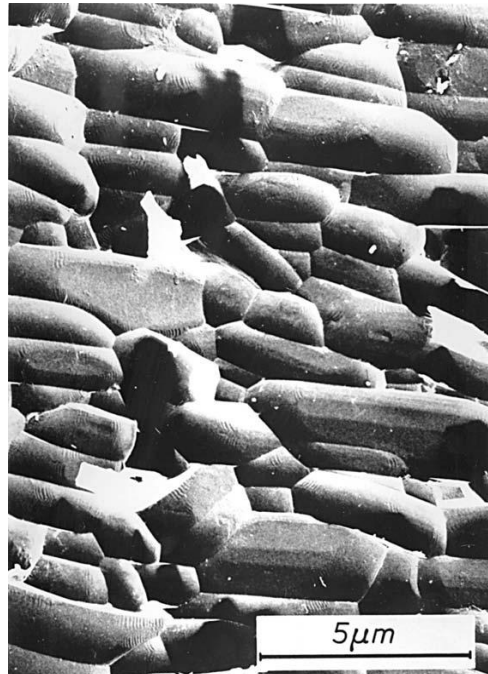
Figure 2.23 Microstructure of an oriented barium hexaferrite (Moulson & Herbert, 2003)
