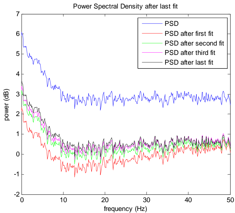
Figure 3.14 Power Spectral Density after each fitting operation for the first thirty seconds of the sleep recording data with the length of 7 hours.
