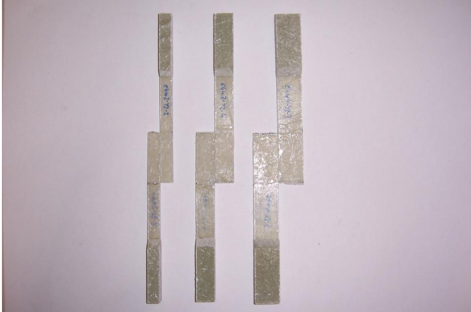
Şekil 6.50 E4W2-Y2, E4W3-Y2, E4W4-Y2 hasar tipleri
