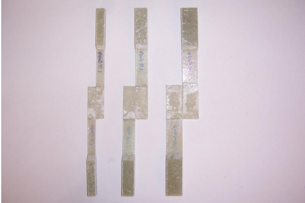
Şekil 6.8 E4W2-Y1, E4W3-Y1, E4W4-Y1 hasar tipleri
