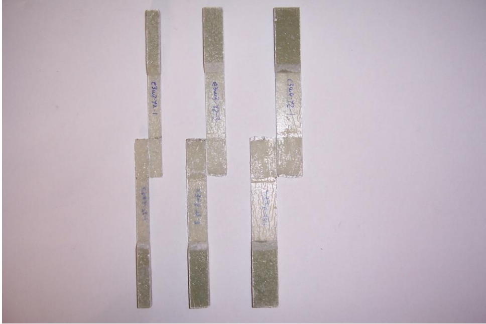
Şekil 6.48 E3W2-Y2, E3W3-Y2, E3W4-Y2 hasar tipleri
