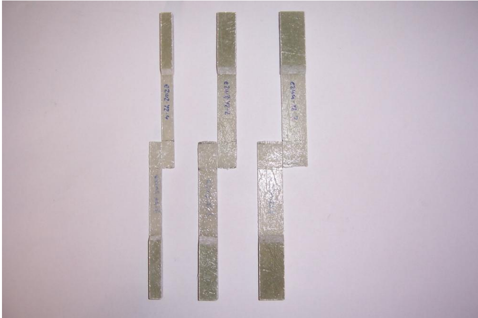
Şekil 6.46 E2W2-Y2, E2W3-Y2, E2W4-Y2 hasar tipleri
