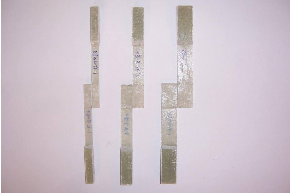
Şekil 6.6 E3W2-Y1, E3W3-Y1, E3W4-Y1 hasar tipleri
