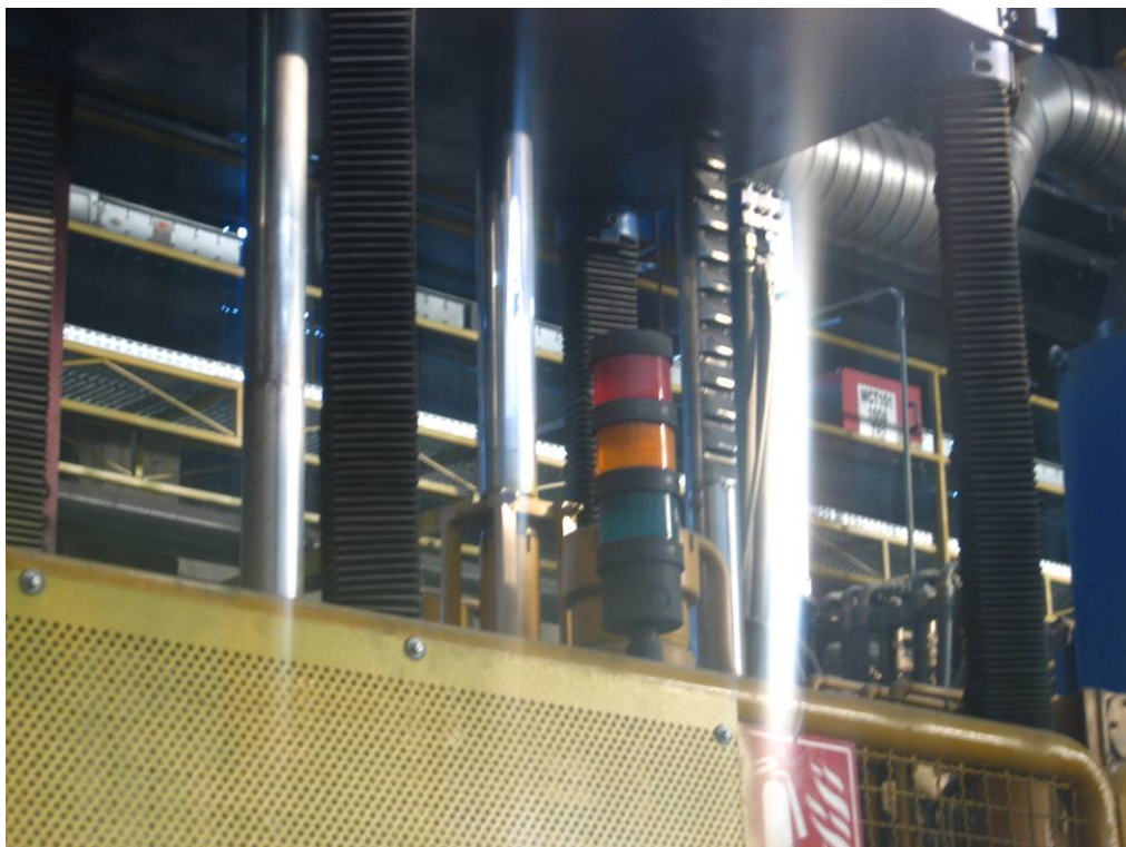
Figure 5.13 Three degree lightening system showing level of metal inside bench
