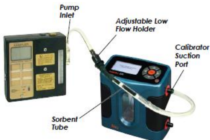
Figure 3.10 Example of the flow controller connection to sampling system
