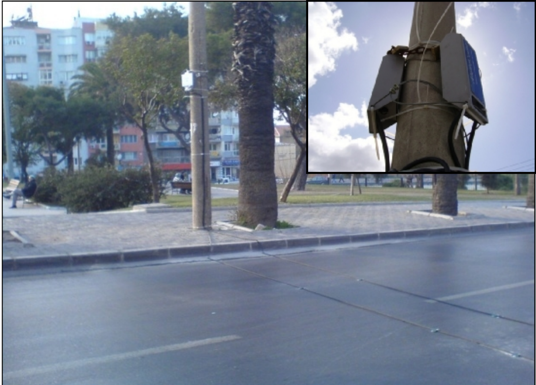
Figure 4.1 The portable vehicle classifier system placed on a road surface.
