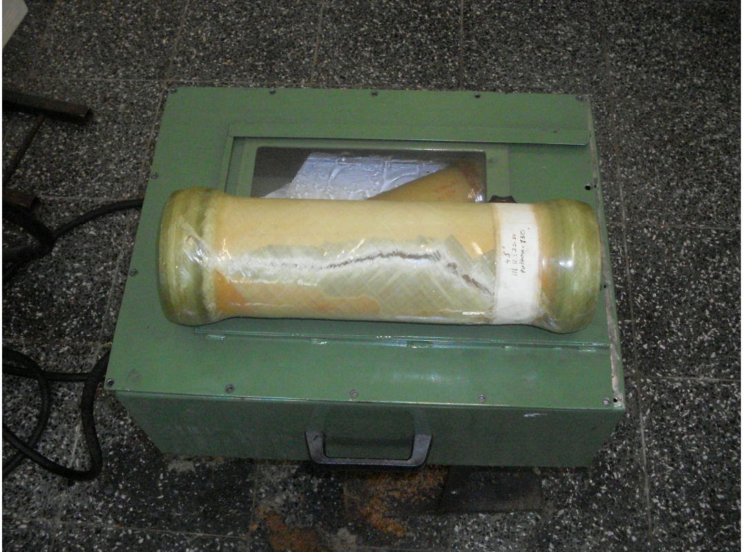
Figure 7.8 Fiber breakage damage mechanism
