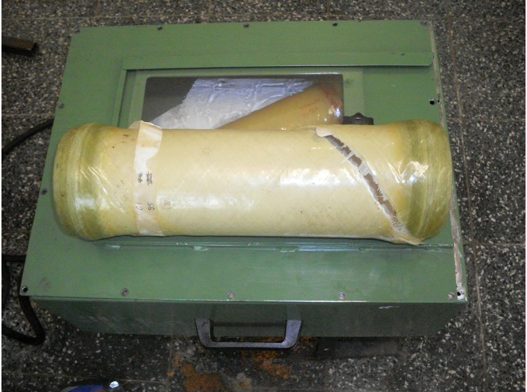
Figure 7.6 Fiber breakage damage mechanism
