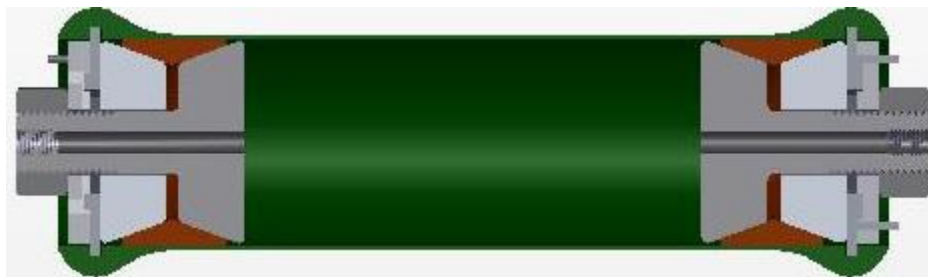
Figure 6.3 Closed-end internal pressure test apparatus.
