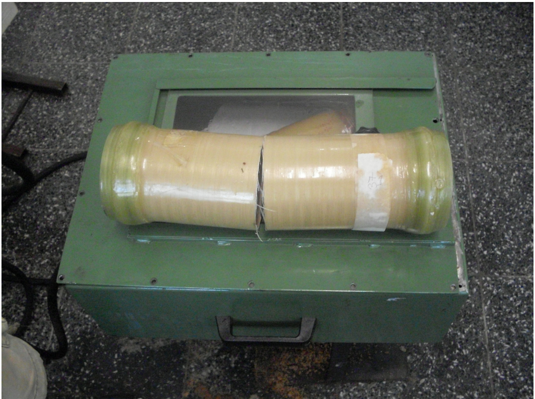
Figure 7.7 Fiber breakage damage mechanism
