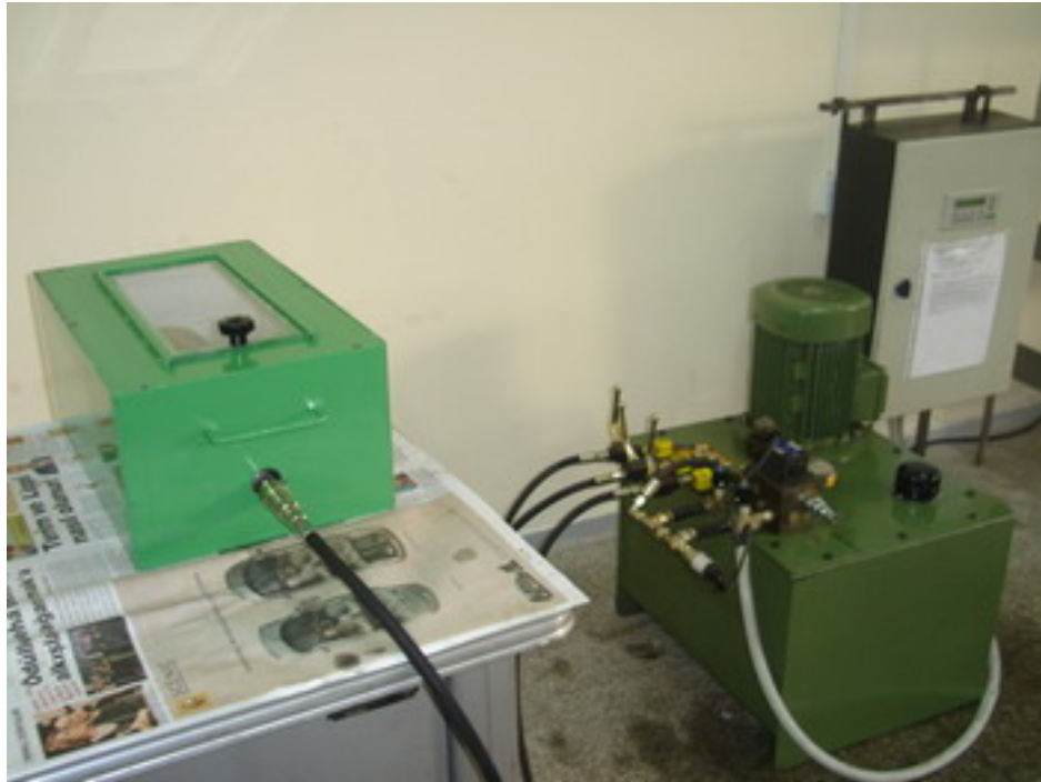
Figure 6.6 A PLC controlled servo-hydraulic testing machine.
