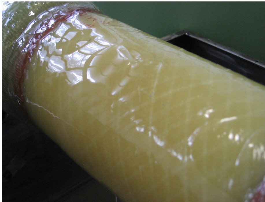
Figure 4.19 Jet I state of fatigue loading of composite pipe.
