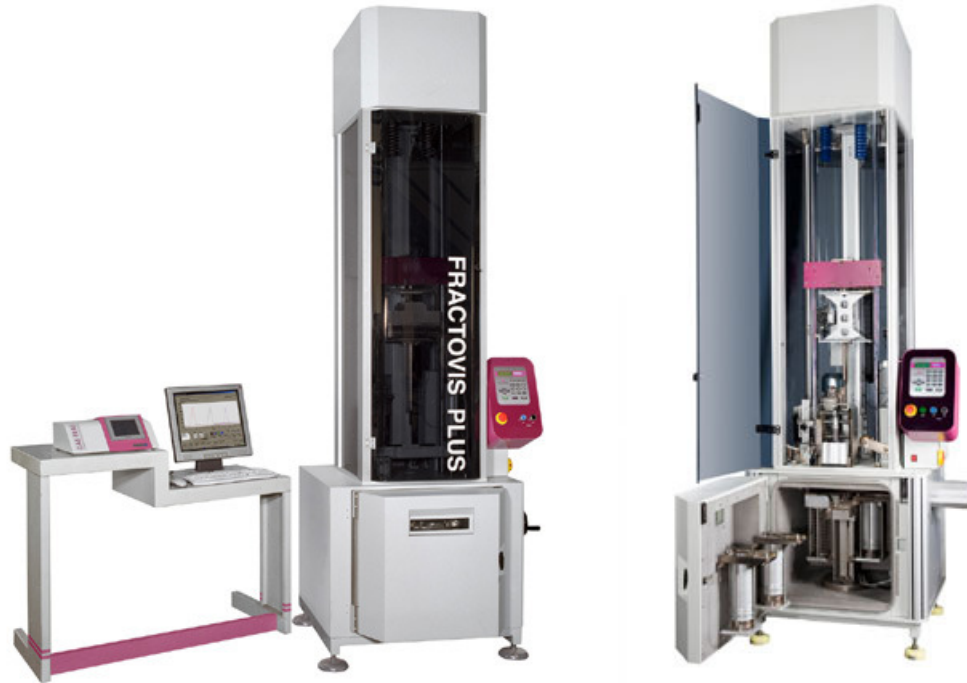
Figure 3.6 The Caest-Fractovis Plus impact machine (and inside outlook).
