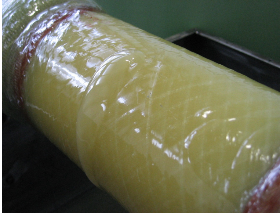
Figure 4.18 Strong leakage state of fatigue loading of composite pipe.
