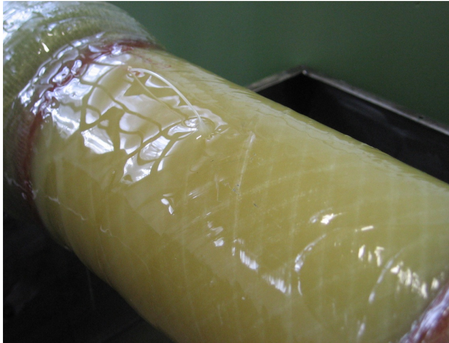
Figure 4.20 Jet II state of fatigue loading of composite pipe.
