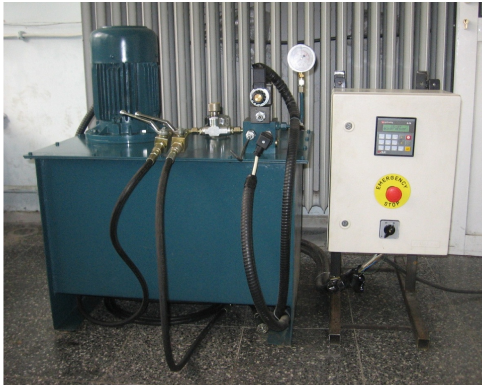
Figure 3.9 PLC controlled servo-hydraulic testing machine.
