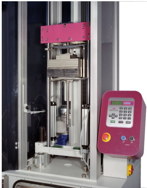
Figure 3.7 Impactor and crosshead mass.
