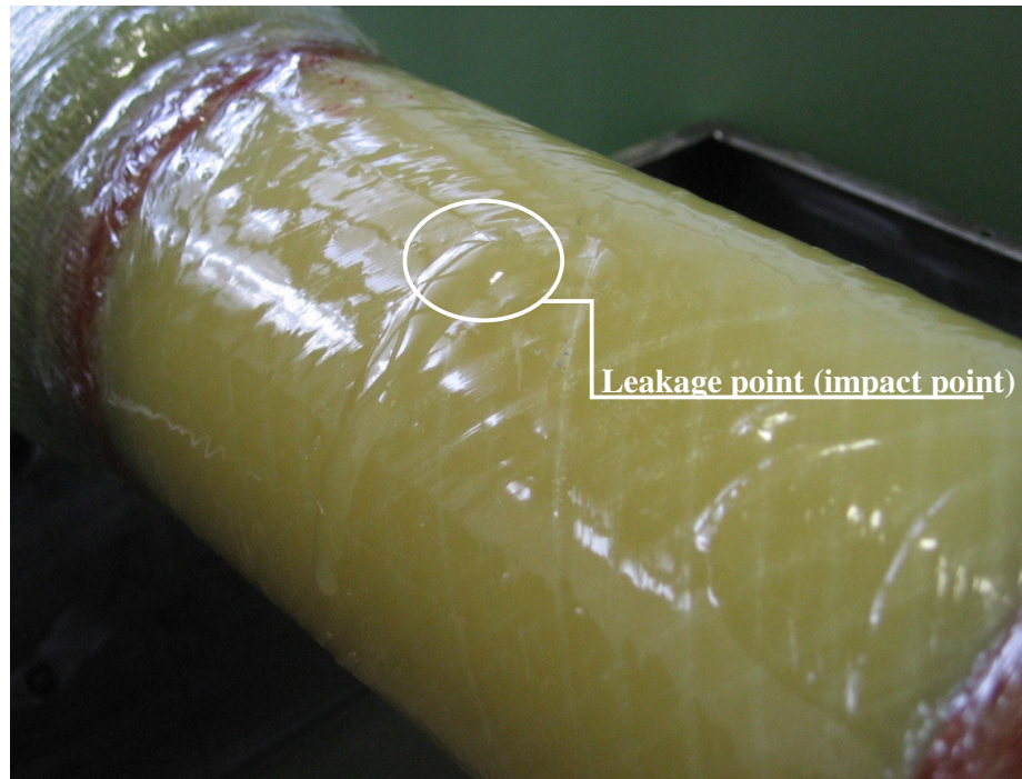
Figure 4.16 Leakage state of fatigue loading of composite pipe.
