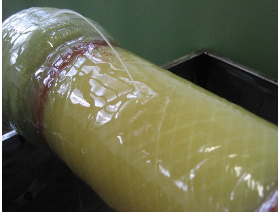
Figure 4.22 Jet IV state of fatigue loading of composite pipe.
