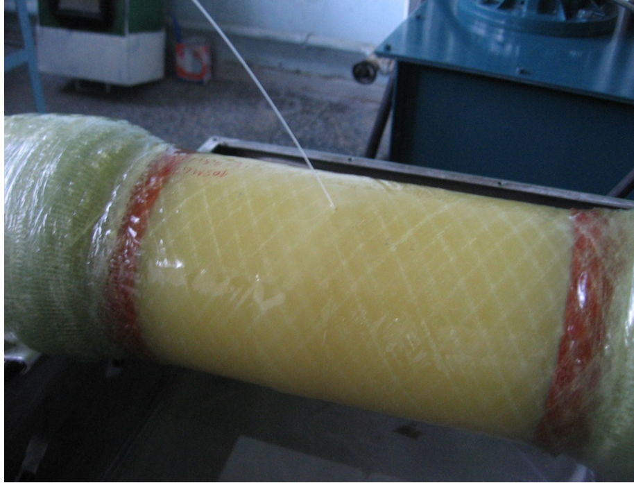
Figure 4.24 Eruption state of fatigue loading of composite pipe.
