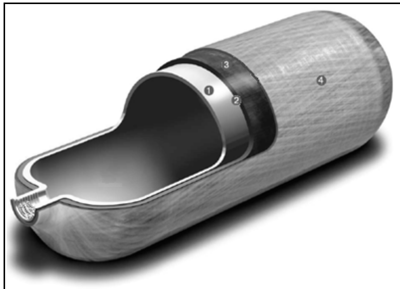
Figure 2.1 Example of universal filament wound composite pressure vessels.
