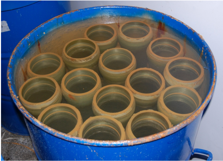
Figure 3.3 FW-GFRP pipes under simulated sea water condition.
