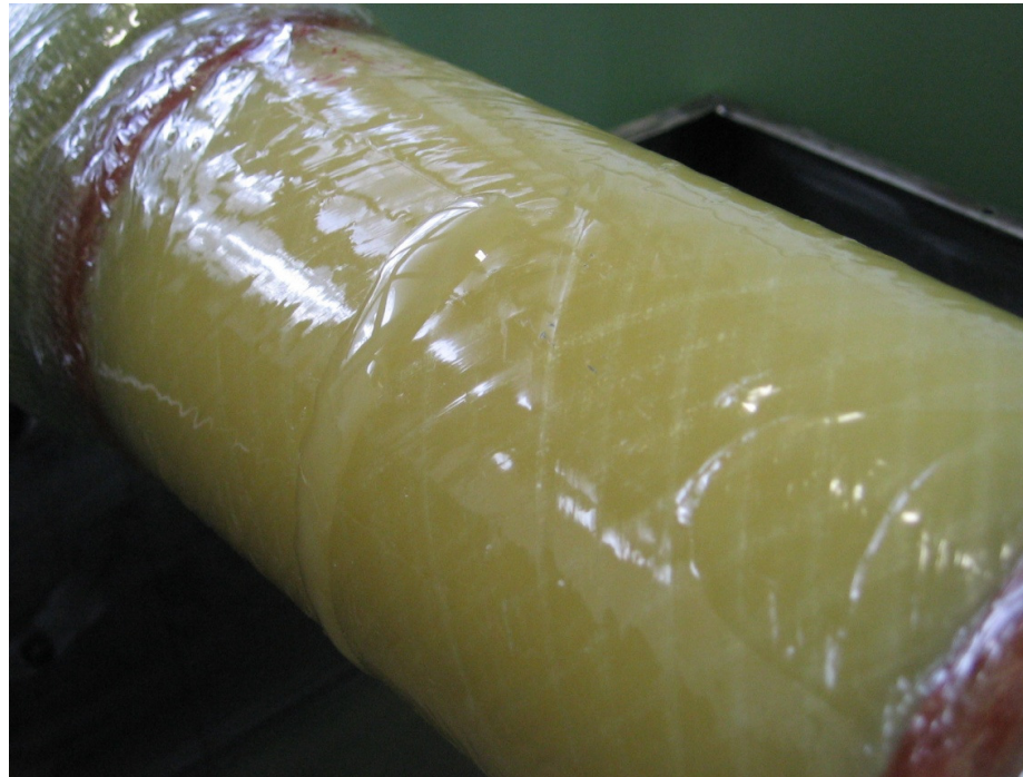
Figure 4.17 Advanced leakage state of fatigue loading of composite pipe.
