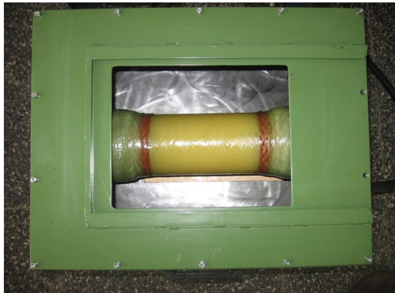
Figure 3.14 A protective test box.
