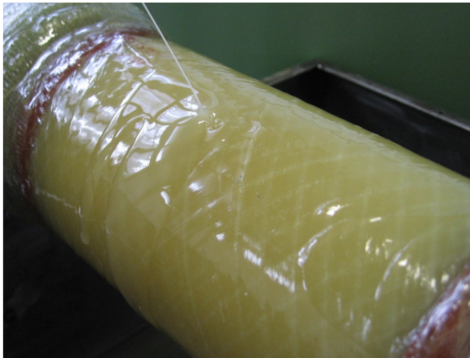
Figure 4.23 Exact jet state of fatigue loading of composite pipe.
