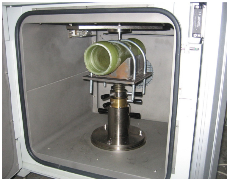
Figure 3.8 V-block test fixture and specimen for impact.
