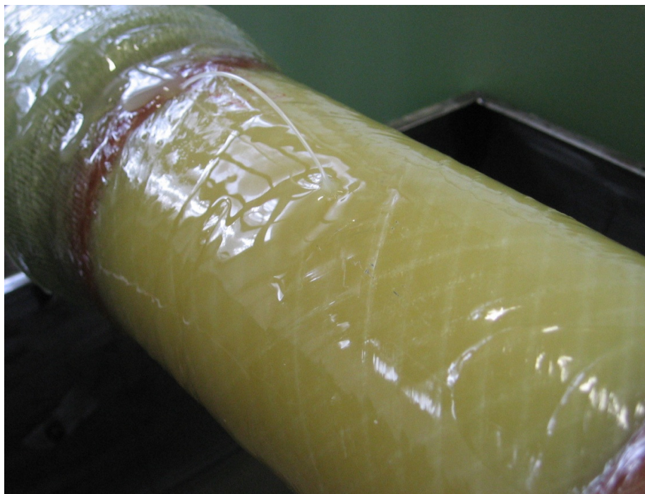
Figure 4.21 Jet III state of fatigue loading of composite pipe.
