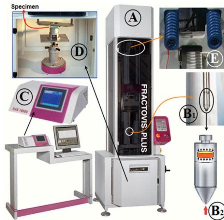
Figure 4.1 Fractovis Plus Low velocity impact tester (A) and its equipments; impactor nose (B 1 ), piezoelectric impactor nose (B 2 ), Data Acquisition System (DAS) (C), the specimen clamp mechanism (D), and the springs (E). (E. Erbil, Impact Loading in Laminated Composites 2008, Dokuz Eylul University)
