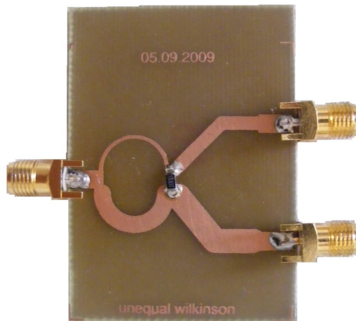
Figure 4.16 The 1:2 unequal Wilkinson power divider
