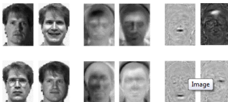
Figure 1.4 Some original (left), PCA (center) and ICA (right) basis images (Deniz, Castrillion & Hernandez, 1999)
