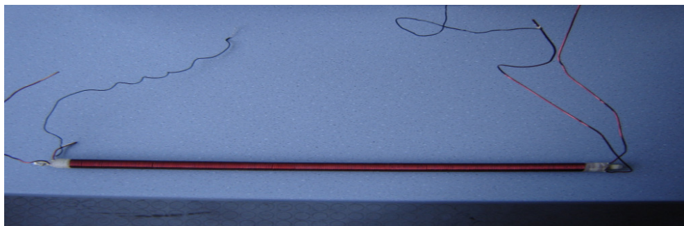
Figure 3.7. Transmission line filter comprised of over and over wounded Solenoid coil.
