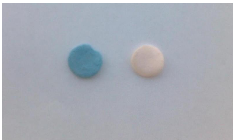
Figure 3.1 Cibacron Blue and Congo Red attached poly(HEMA) cryogelic pellets.
