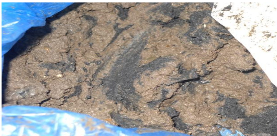
Figure 5.1 Sludge cake sample after centrifuge decantor dewatering unit
