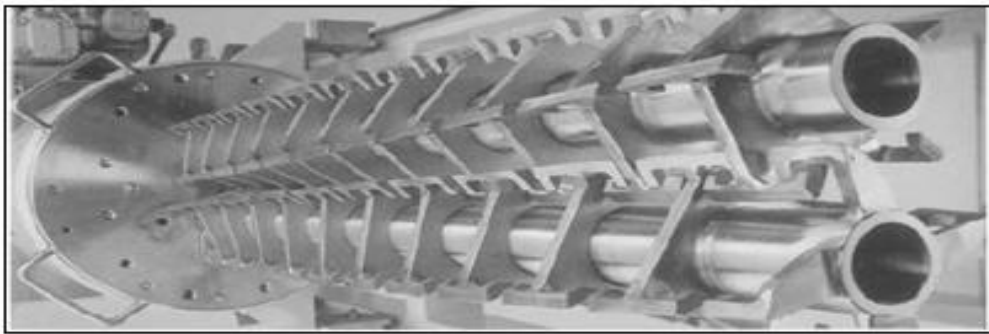
Figure 3.21 Kneading and self-cleaning disc dryer—twin shafts (Chen et al., 2002).
