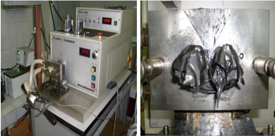
Figure 4.2 General view Brabender Plasticorder W30/The mixing chamber and the rotors after the mixing process of the composite. (Tavman et al., 2008)
