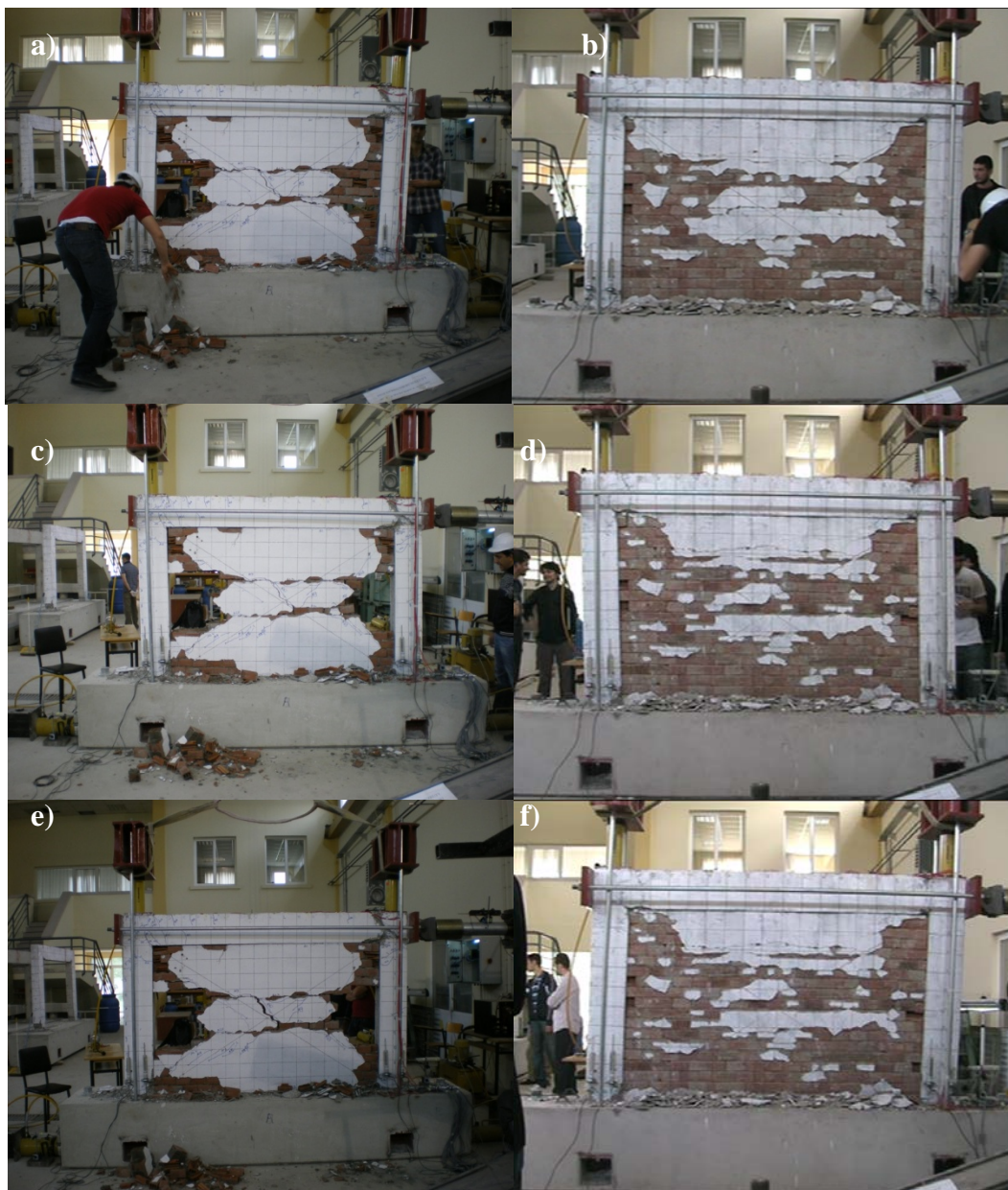
Figure 4.13 Observed damages at specific levels of drift ratio: a) Locked brick frame at -3% drift, b) Standard brick frame at -3% drift, c) Locked brick frame at 3.5% drift, d) Standard brick frame at 3.5% drift, e) Locked brick frame at -3.5% drift, f) Standard brick frame at -3.5% drift
