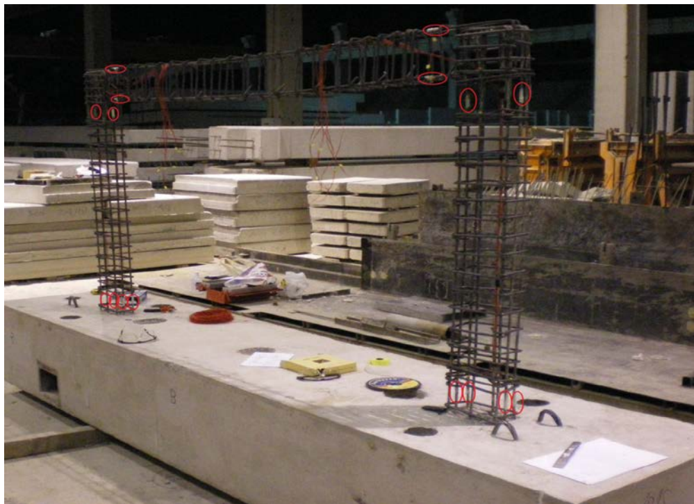
Figure 3.14 Reinforcements were applied strain gauge
