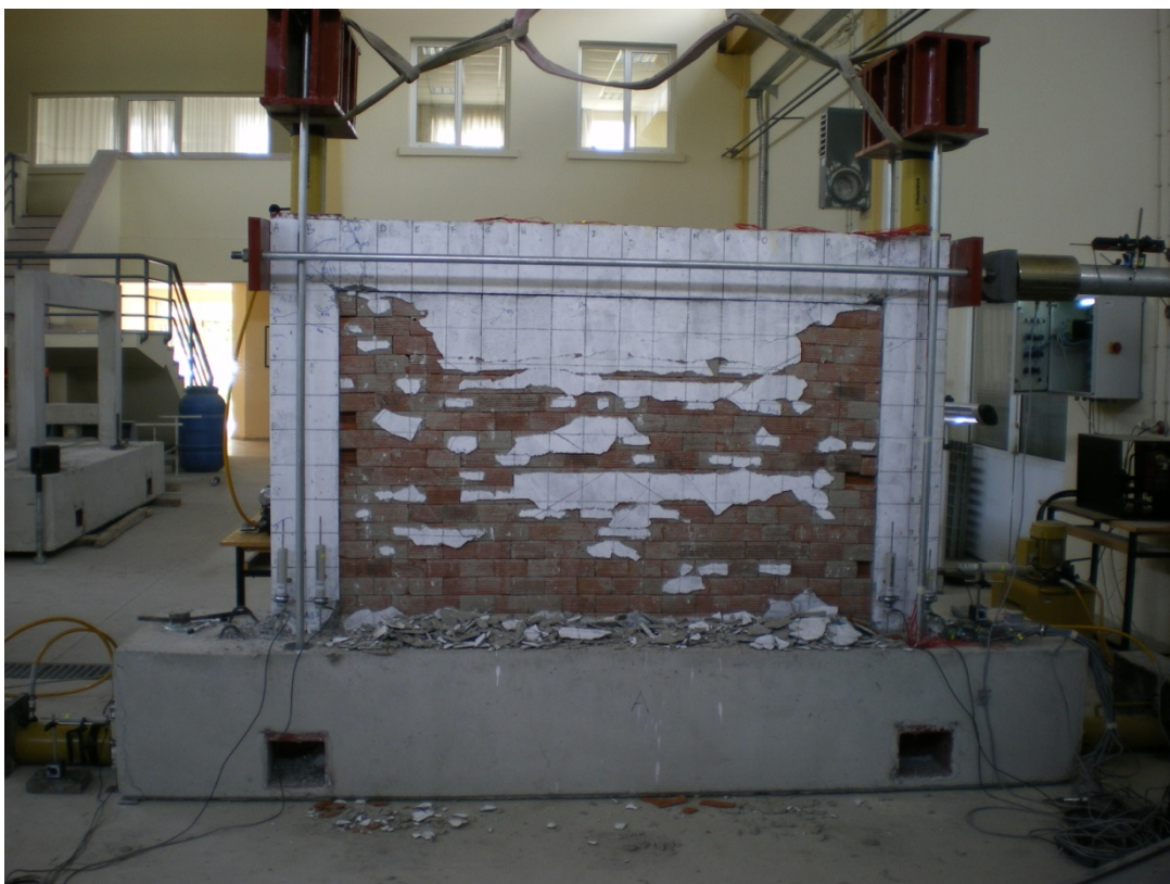
Figure 4.6 Final form of locked brick frame at the final stage
