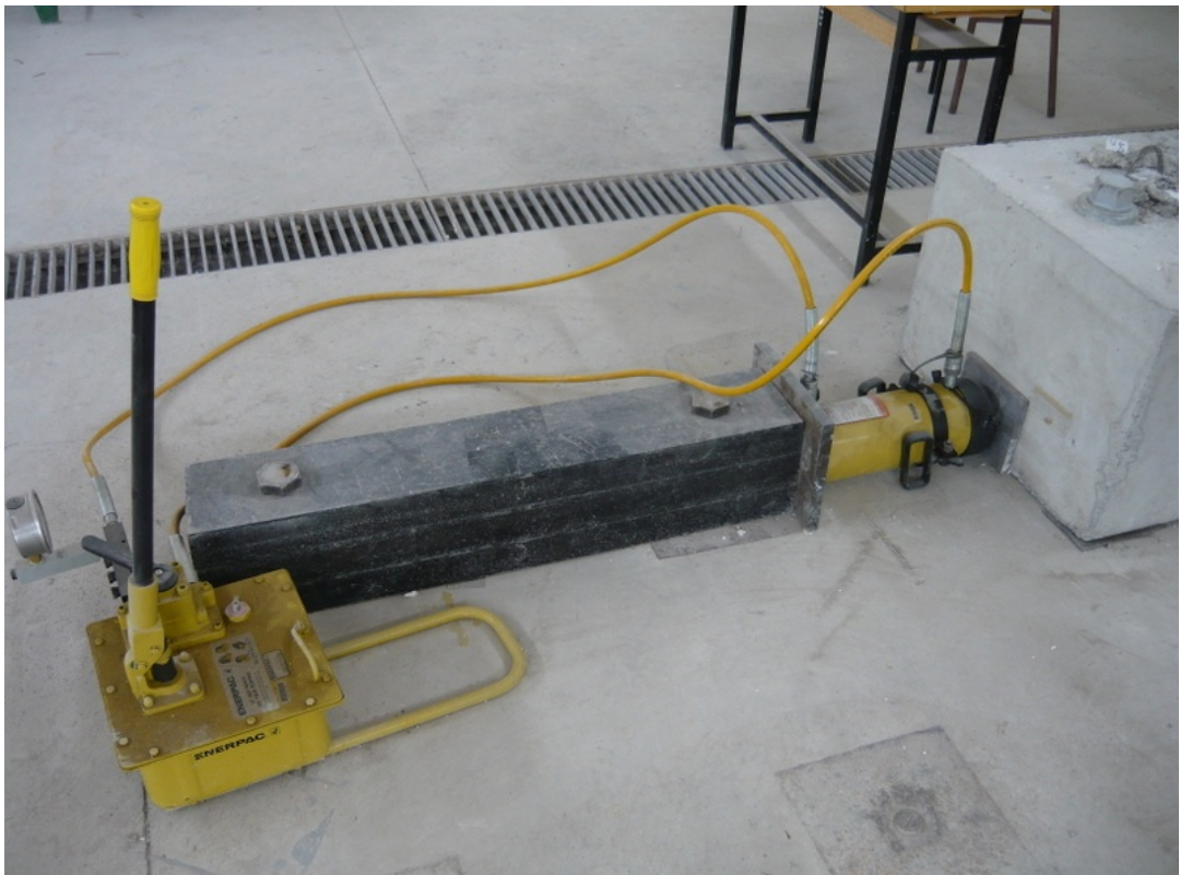
Figure 3.25 Hydraulic rams which constrain foundation
