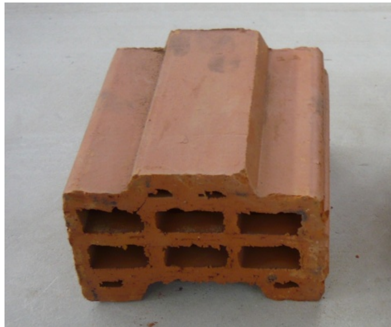
Figure 3.6 Locked brick with a scale of \frac{1}{2}
