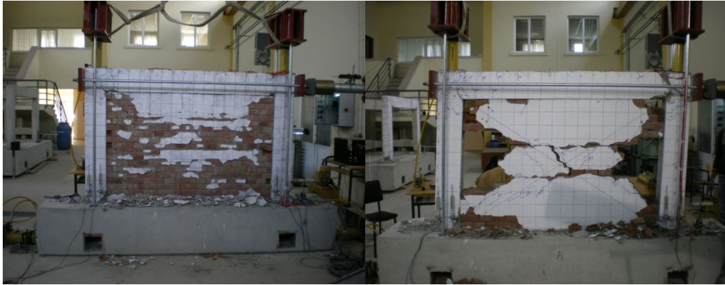
Figure 4.14 Observed damages at specific levels of drift ratio: a) Locked brick frame at the end of the test, b) Standard brick frame at the end of the test
