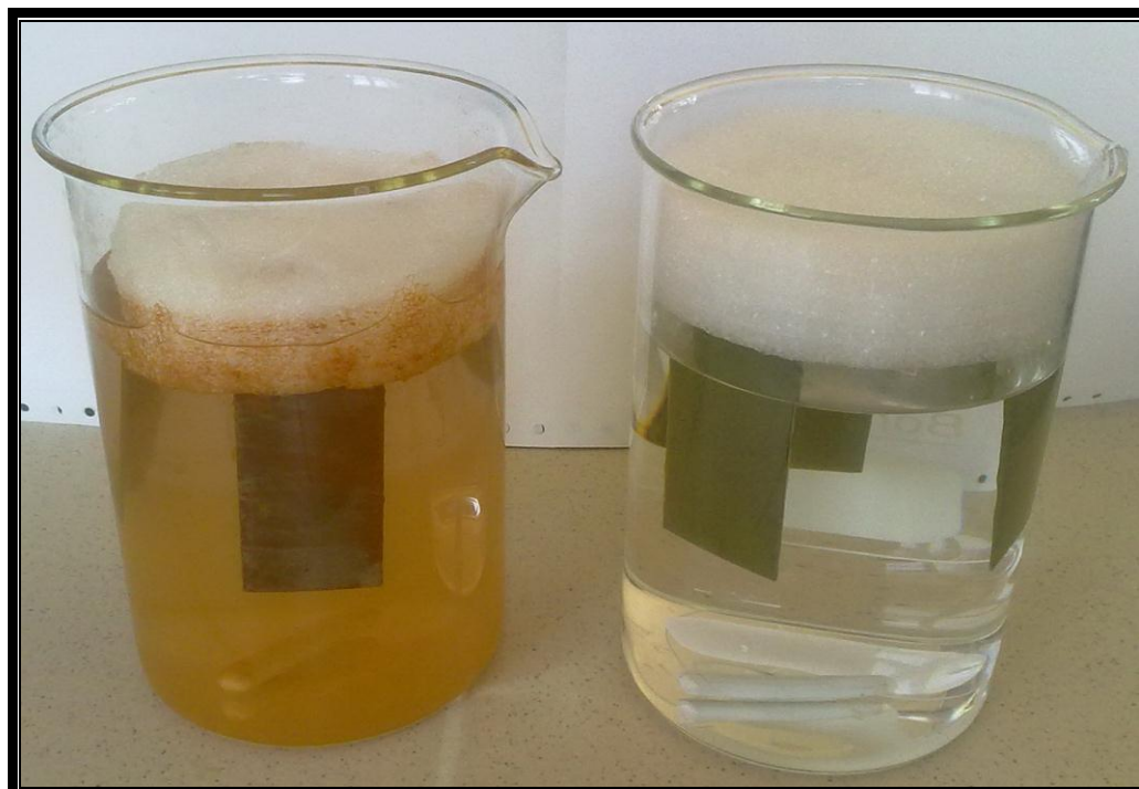
Figure 3.43 The results of the metal (left) and lanolin based material covered (right) metal surfaces which exposed to artificial seawater after the 4 hours expectation time.
