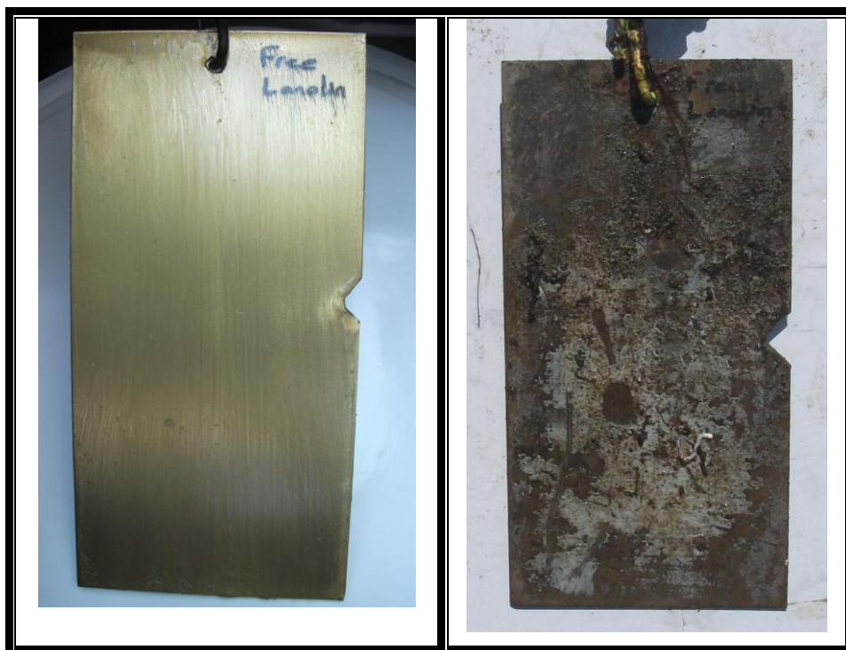
Figure 3.32 The metallic plates (Free lanolin based material) exposed in Zeytinburnu coast 2 months immersion, left: before immersion, right: after 2 months.
