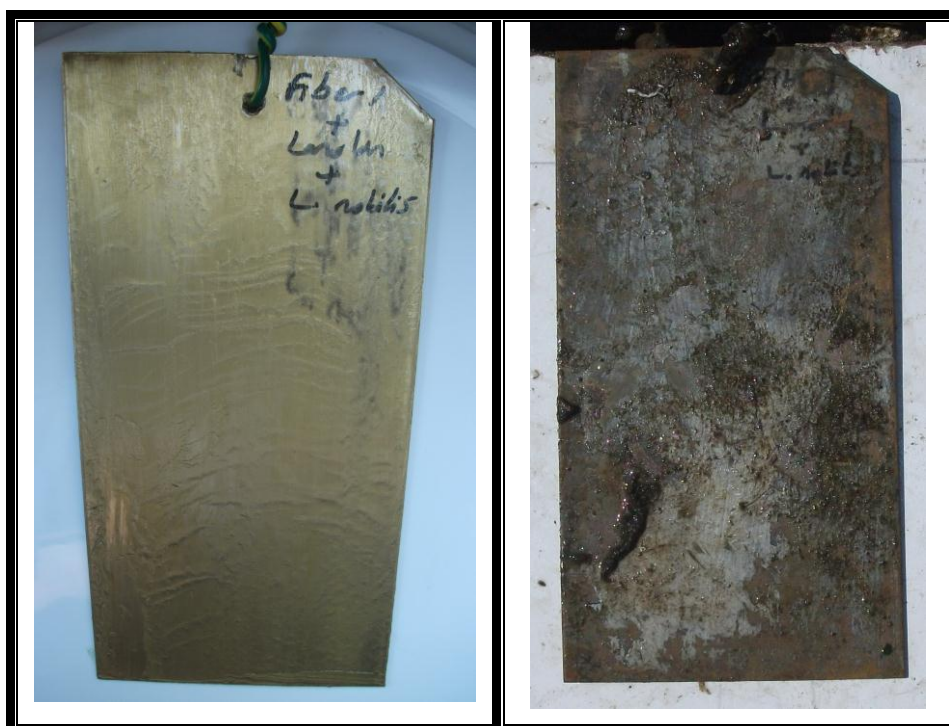
Figure 3.36 The metallic plates (Lanolin based material, Fiber 1 and L.nobilis extract) exposed in Zeytinburnu coast 2 months immersion, left: before immersion, right: after 2 months.
