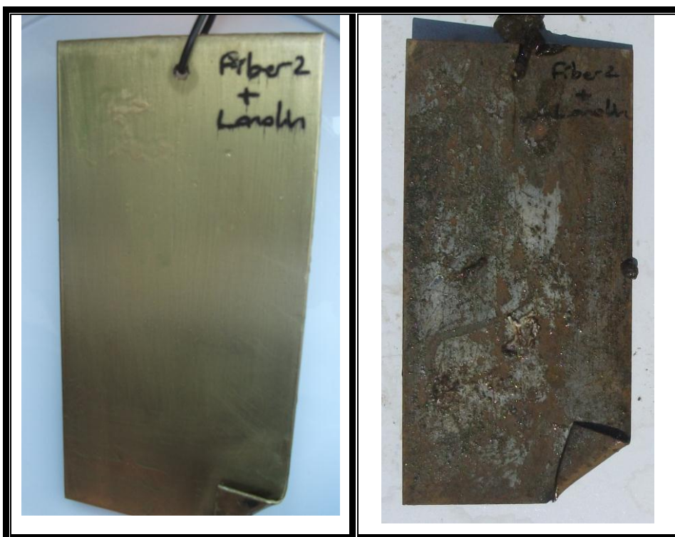
Figure 3.38 The metallic plates (Lanolin based material and Fiber 2) exposed in Zeytinburnu coast 2 months immersion, left: before immersion, right: after 2 months.
