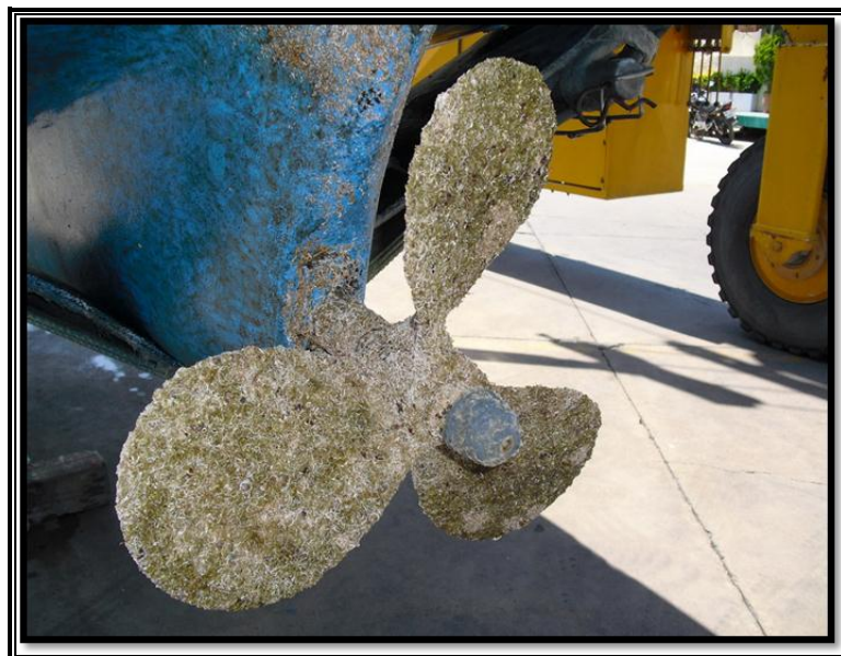
Figure 1.9 A ship's propeller which exposed to fouling (Photo: Levent Çavaş).
