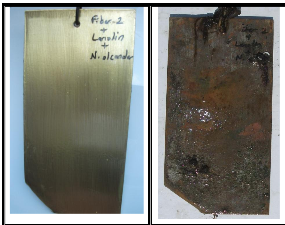
Figure 3.40 The metallic plates (Lanolin based material, Fiber 2 and N.oleander extract) exposed in Zeytinburnu coast 2 months immersion, left: before immersion, right: after 2 months.
