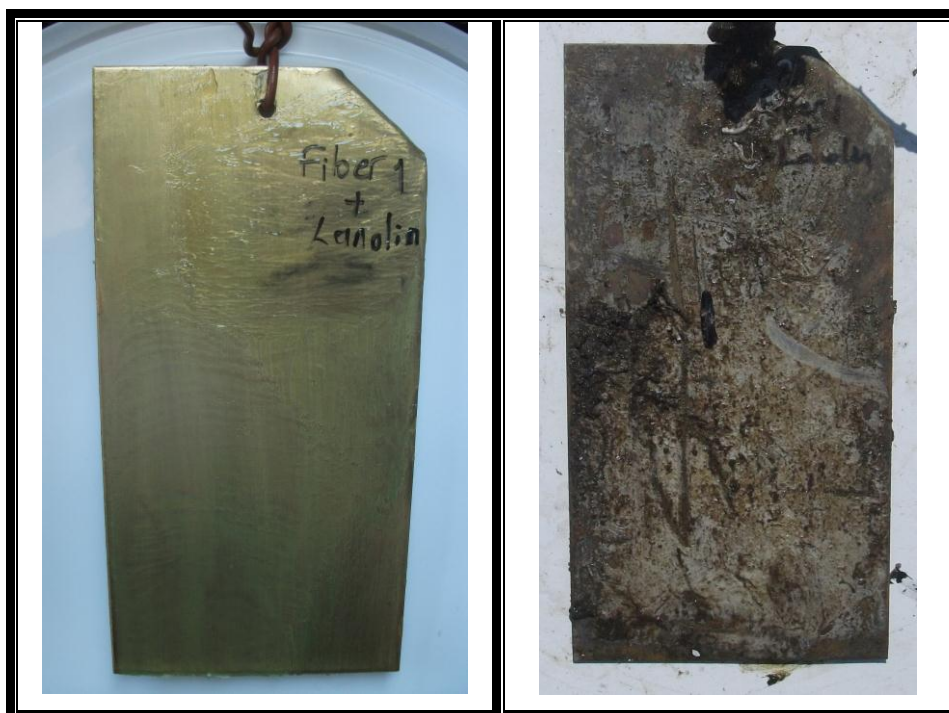
Figure 3.35 The metallic plates (Lanolin based material and Fiber 1) exposed in Zeytinburnu coast 2 months immersion, left: before immersion, right: after 2 months.
