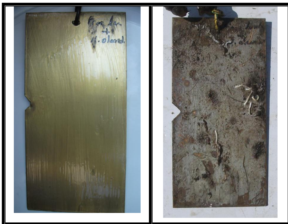
Figure 3.34 The metallic plates (Lanolin based material and N.oleander extract) exposed in Zeytinburnu coast 2 months immersion, left: before immersion, right: after 2 months.
