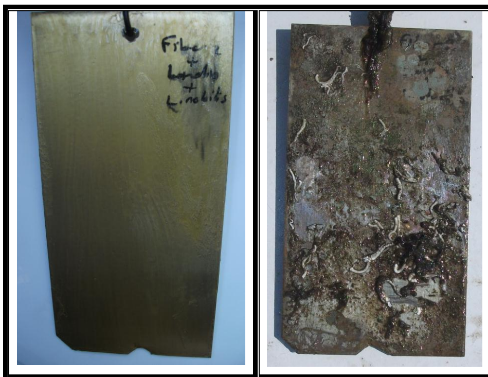
Figure 3.39 The metallic plates (Lanolin based material, Fiber 2 and L.nobilis extract) exposed in Zeytinburnu coast 2 months immersion, left: before immersion, right: after 2 months.
