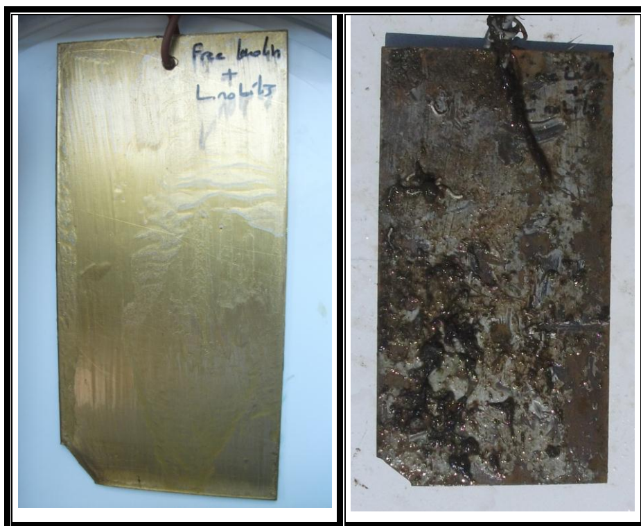
Figure 3.33 The metallic plates (Lanolin based material and L.nobilis extract) exposed in Zeytinburnu coast 2 months immersion, left: before immersion, right: after 2 months.
