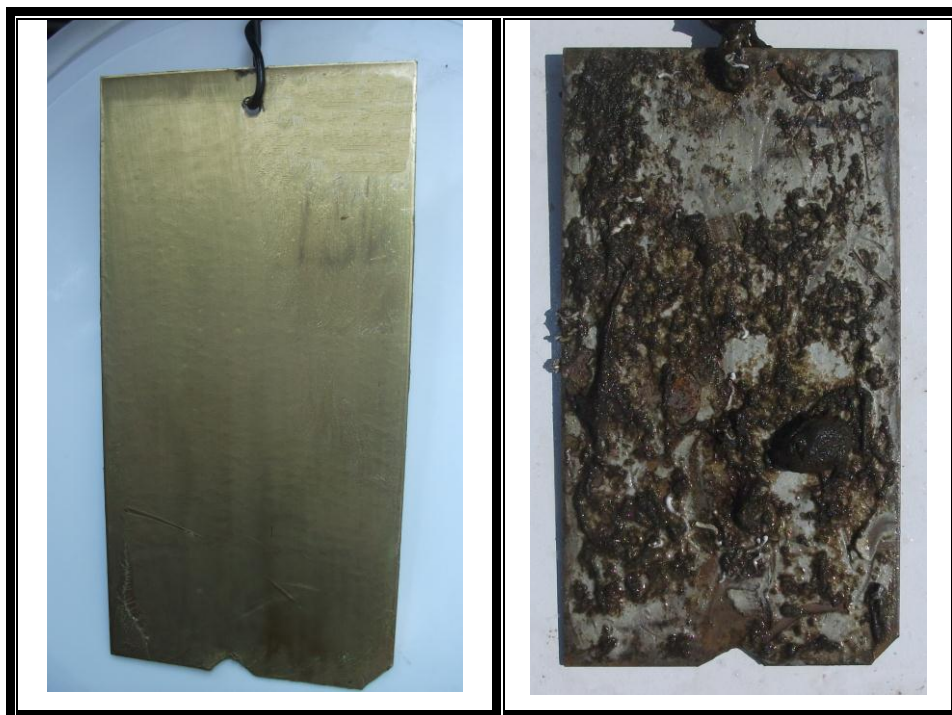
Figure 3.31 The metallic plates (Control group) exposed in Zeytinburnu coast 2 months immersion, left: before immersion, right: after 2 months.
