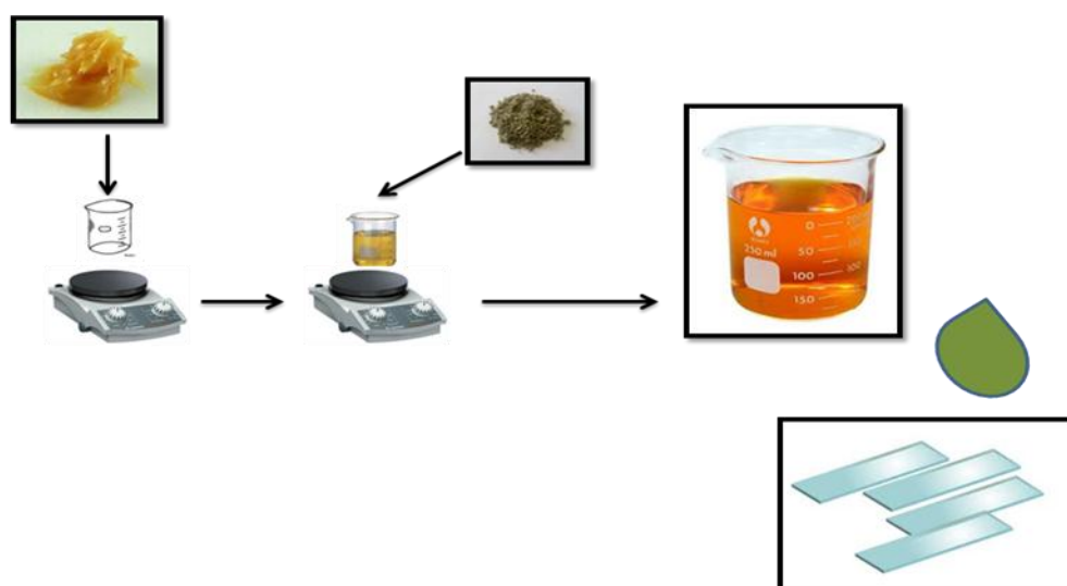
Figure 2.3 Preparation of the fibre reinforced lanolin based material.
