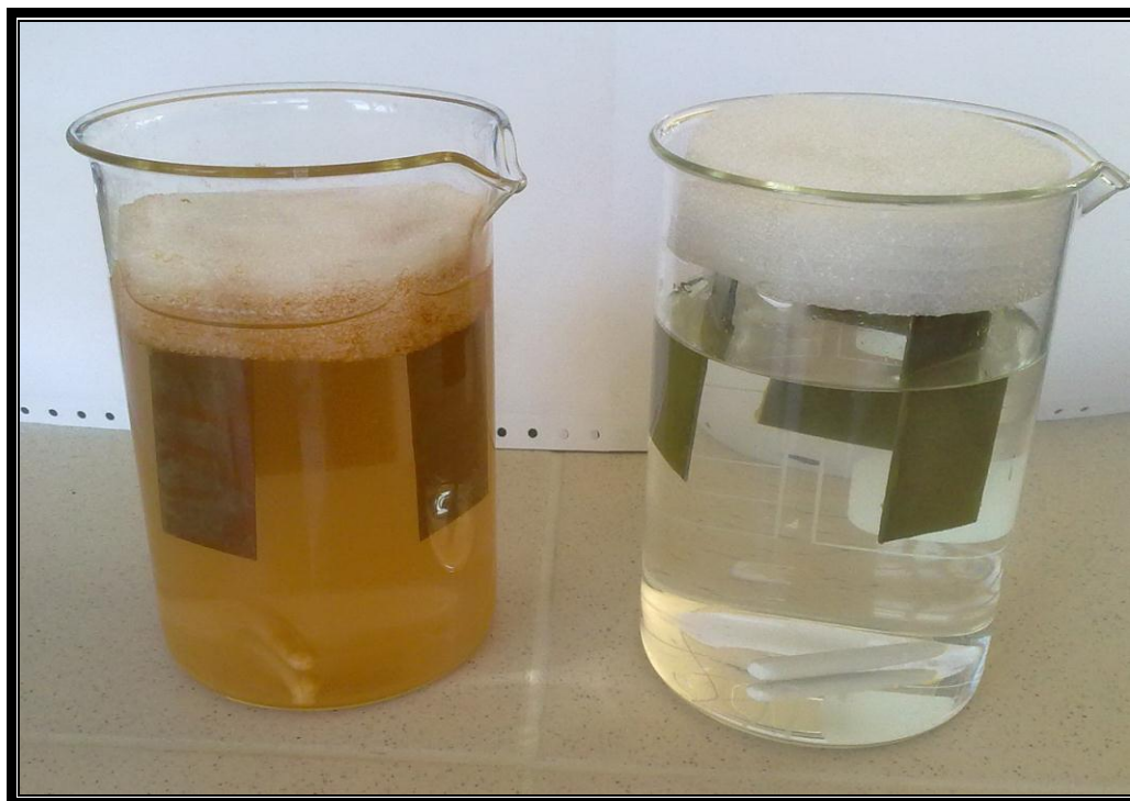
Figure 3.44 The image of the metal (left) and lanolin based material covered (right) metal surfaces which exposed to artificial seawater after the 6 hours expectation time.
