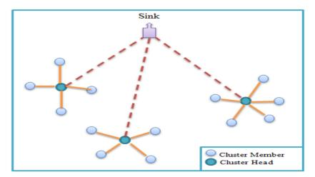
Figure 4.11 Hierarchical cluster-based architecture in WSNs
