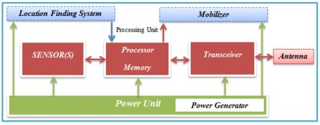
Figure 1.3 General hardware architecture of a sensor node
