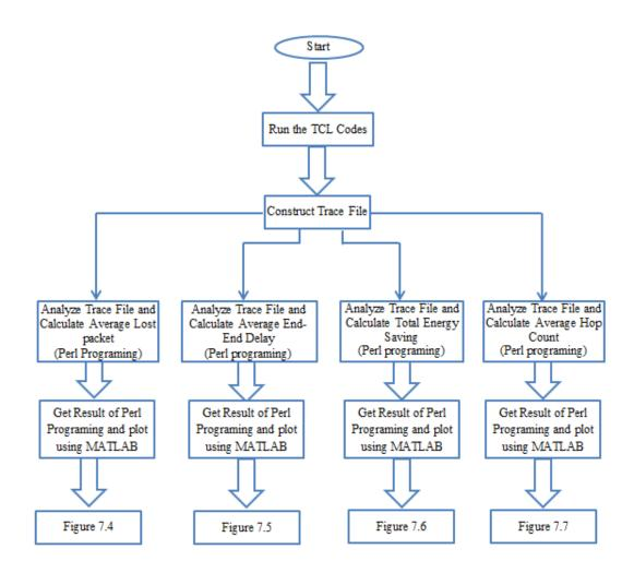
Figure 7.3 Block diagram describes Simulation flow
