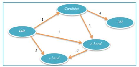
Figure 4.5 State transitions for the FLOC clustering algorithm
