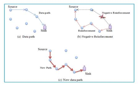
Figure 5.5 Negative reinforcement
