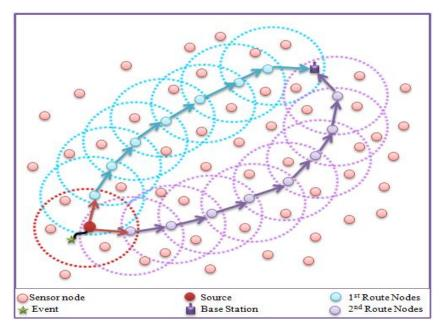
Figure 6.3 Routing Phase in TWELGossiping
