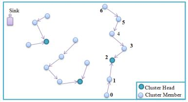
Figure 4.12 Chain structures of PEGASIS
