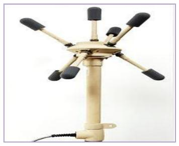
Figure 3.5 Boomerang sniper detection system (Akyildiz & Canvuran, 2010)
