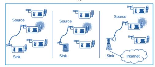
Figure 2.2 shows the sources and the main types of sinks.
