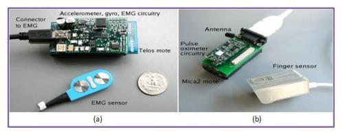
Figure 3.6 Medical sensor nodes used in CodeBlue: (a) Telos mote with EMG sensor and (b) Mica2 mote with pulse oximeter sensor
