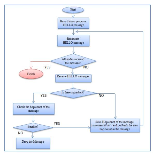
Figure 6.2 flowchart of TWELGossiping Network Initialization phase
