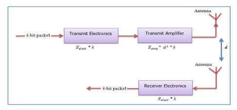
Figure 7.1 Schematic diagram of the first order radio model equation
