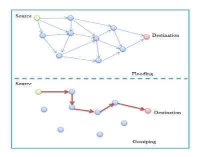
Figure 5.8 forwarding mechanism of both Flooding and Gossiping
