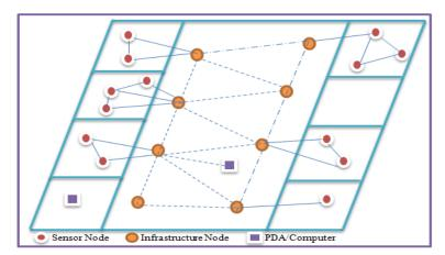
Figure 3.7 Code Blue architecture in a hospital setting (redrawn from (Akyildiz & Canvuran, 2010))
