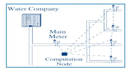
Figure 3.8 Non-intrusive Autonomous Water Monitoring System (NAWMS) Architecture
