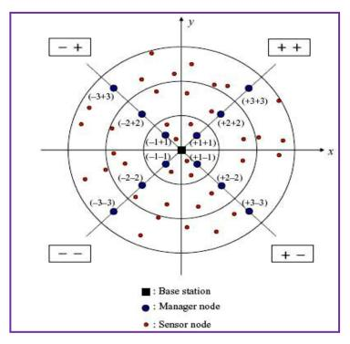
Figure 5.6 Locations of the nodes based on 2-dimensional (x, y) Coordinates
