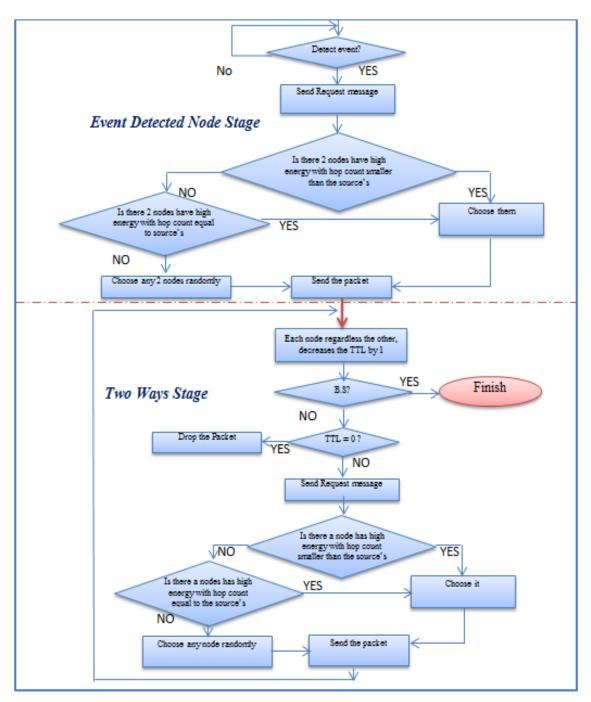
Figure 6.4 flow chart of Routing Phase in TWELGossiping
