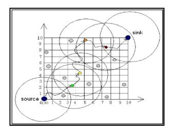
Figure 5.10 Schematic of Data Routing in LGossiping
