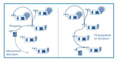
Figure 2.6 A mobile sink moves through a sensor network
