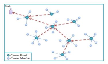
Figure 4.13 Hierarchical architecture of TEEN and APTEEN
