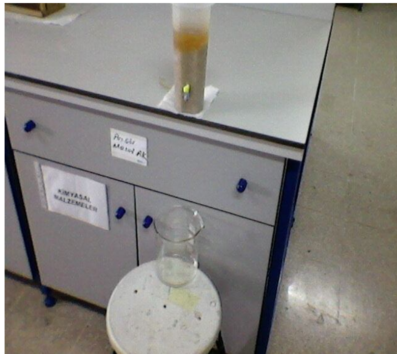
Figure 4.8 Filtration of flocs after EC process.
