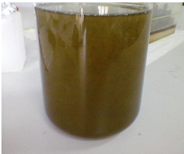
Figure 5.3 The EC effluent water in yellowish color.
