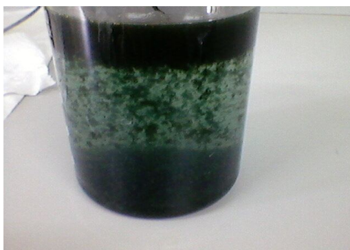
Figure 5.11 With the addition of NaCl into the As(V) solution formation of dark green flocs were observed in the EC.
