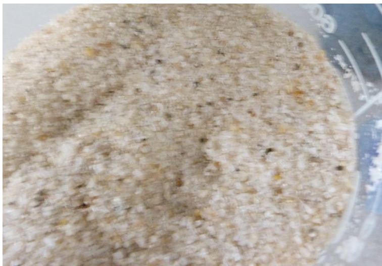
Figure 4.5 Quartz sand was used in the filtration process.
