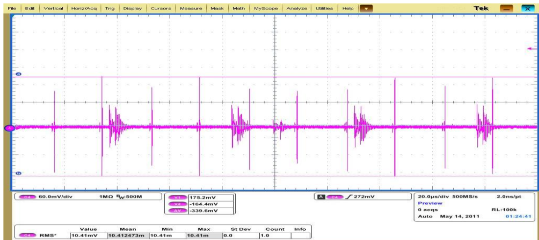
Figure 4.35 Interleaved PFC Controller Frequency Foldback Pin(probe10x)
