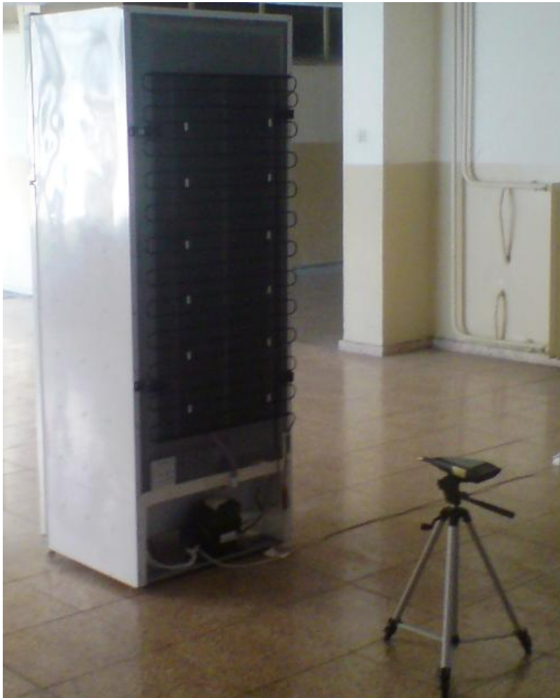
Figure 4.22 Sound measurement when the refrigerator is sitting on the floor ( \alpha = 0 ).
