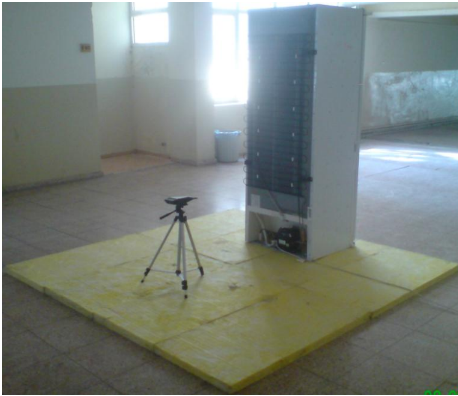
Figure 4.27 Sound measurement when the refrigerator is sitting on glass wool ( \alpha = 0.30 ).
