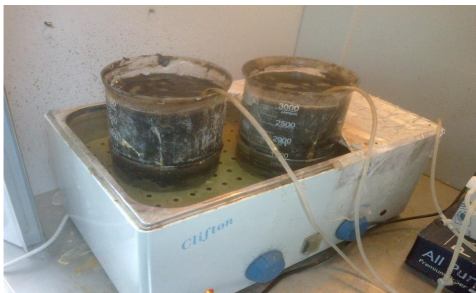
Figure 3.2 Semi-batch aerobic digesters
